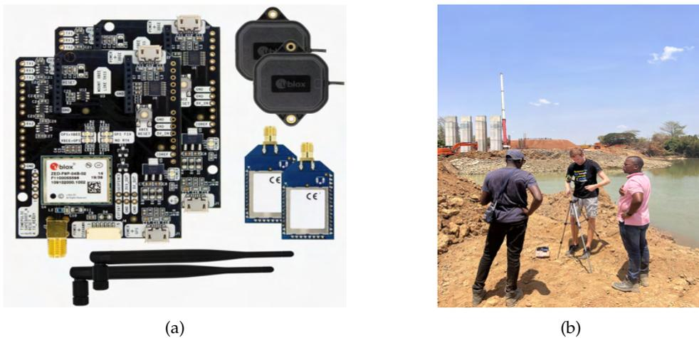
Figure 2.9.: (a) The simpleRTK2B - Starter Kit LR, from: [ArduSimple \[2023\]](#) (b) Setup of the simpleRTK2B base together with the BPA staff.
