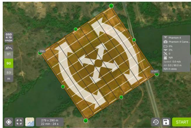
Figure 3.3.: Flight plan, from: Pix4Dcapture [2018].
