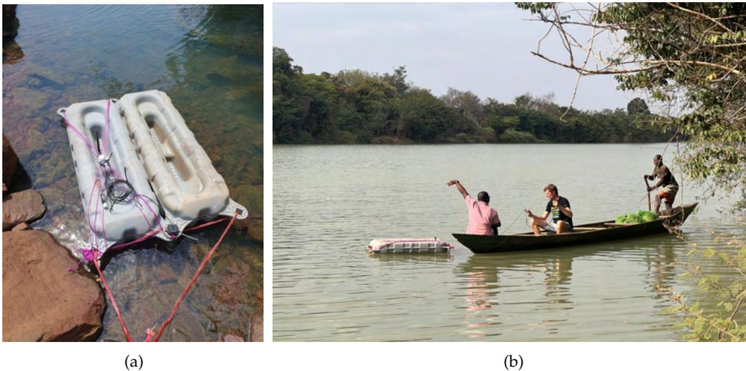
Figure 2.8.: (a) The attachment of the cost-effective Deeper Sonar Chirp+ and the RTK-GNSS on the floaters. (b) Measuring the wet bathymetry of the Black-Volta River using a local fisherman his canoe.
