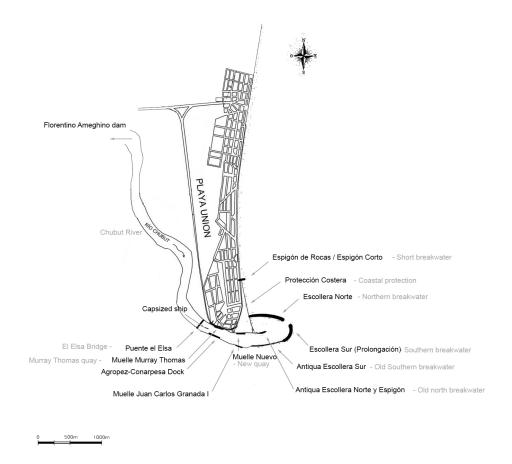
Figure 3.6: Overview of the hard structures in the area (Adapted from (Hugo Juan Donini, 2021))
