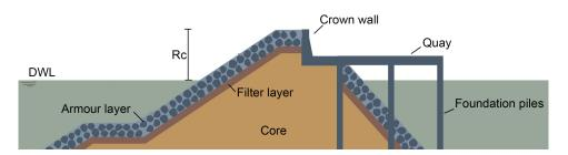
Figure 8.8: Cross section of the design of the new breakwater, adapted from Van der Meer et al. (2018)
