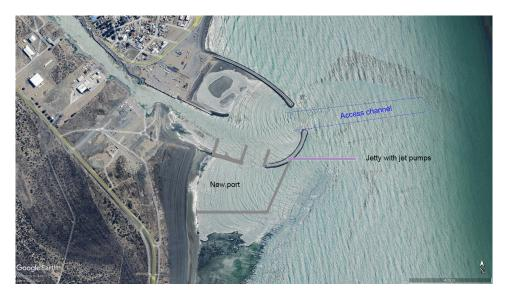
Figure 8.10: Layout new port with sediment bypass
