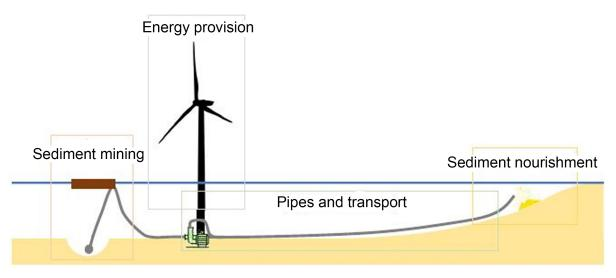
Figure J.6: Sandwindmill (adapted from Rutteman (2021))
