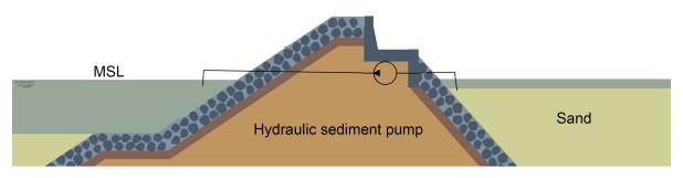
Figure 8.5: Schematizing of the sediment bypass using pumps on the northern breakwater, adapted from Van der Meer et al. (2018)
