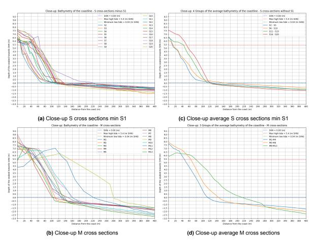
Figure 4.11: Close-up of the S and M cross of the bathymetry analysis of the bathymetry data provided by Savioli et al. (2011)
