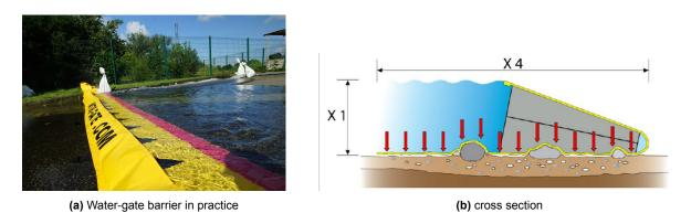
Figure K.3: Water-gate flood barrier (Flood protection solutions (2023))
