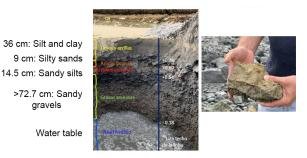
Figure 3.3: Ground layers (left) and tuff stone (right) (Serman y Asociados s.a., 2019)
