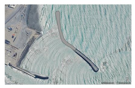
Figure 8.3: New design of opening up the northern breakwater
