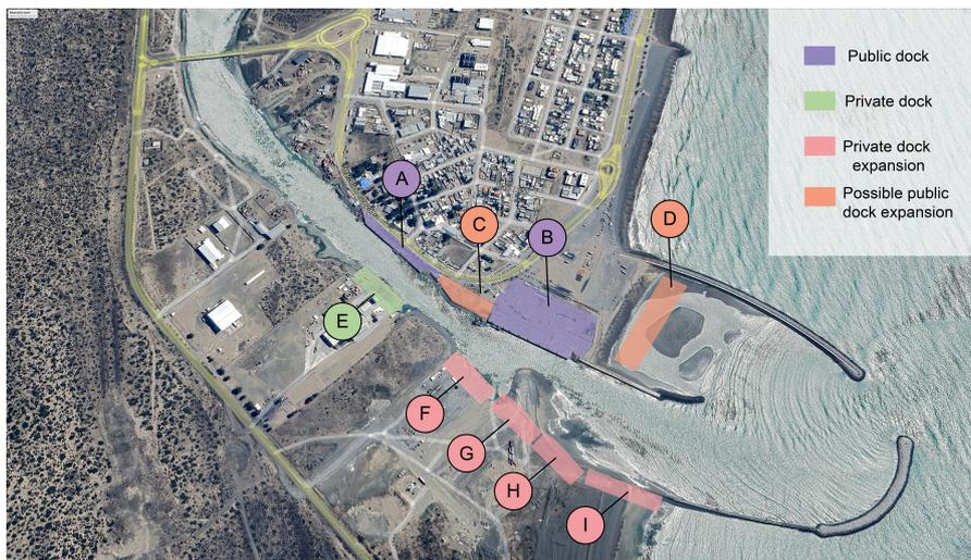
**Figure 5.1:** Overview of the port and development plans (Adapted from Google Earth 2023)
