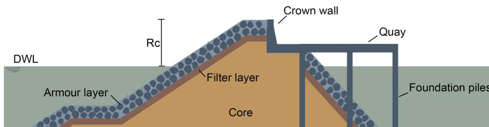
**Figure 8.8:** Cross section of the design of the new breakwater, adapted from Van der Meer et al. (2018)
