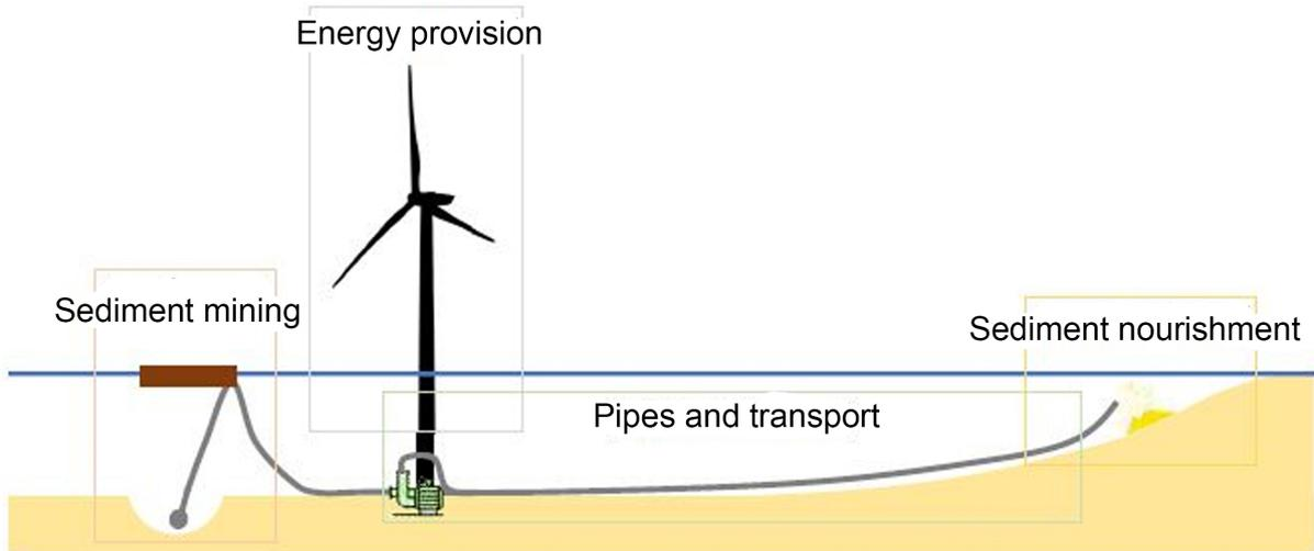
**Figure J.6:** Sandwindmill (adapted from Rutteman (2021))
