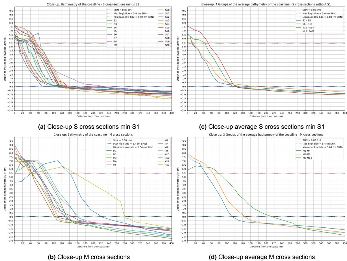
**Figure 4.11:** Close-up of the S and M cross of the bathymetry analysis of the bathymetry data provided by Savioli et al. (2011)
