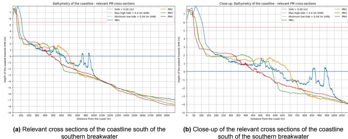
**Figure 8.7:** Analysis of the bathymetry data south of the southern breakwater
