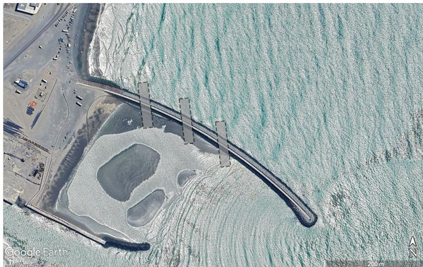
**Figure 8.4:** Schematizing of the tunnels underneath the breakwater
