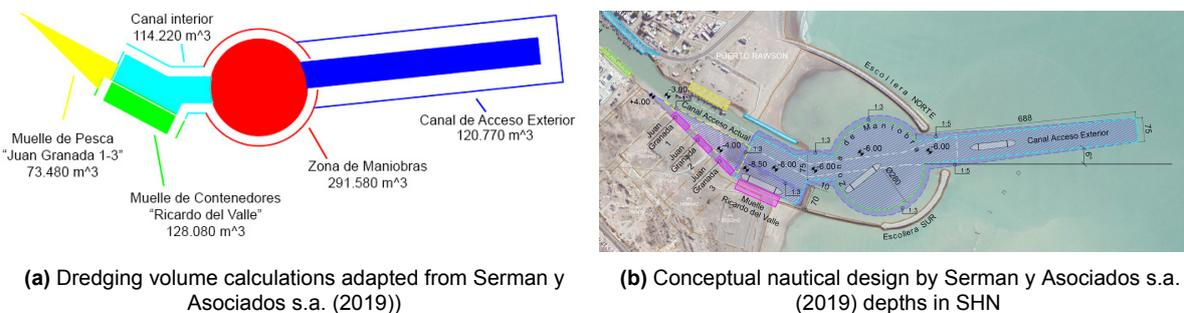
**Figure 5.2:** Location of the new docks and conceptual design for the new port
