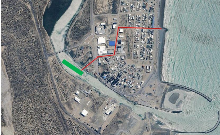
Figure 8.11: Lay-out of the sediment pass pumping system
