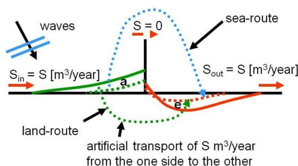
**Figure 8.9:** Principle sand by-pass system (van de Graaff, 2022)
