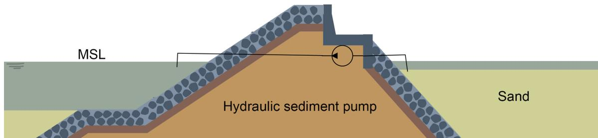
**Figure 8.5:** Schematizing of the sediment bypass using pumps on the northern breakwater, adapted from Van der Meer et al. (2018)
