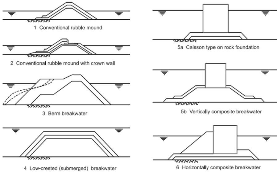
**Figure J.1:** Different types of breakwaters acquired from De Graauw (2022)
