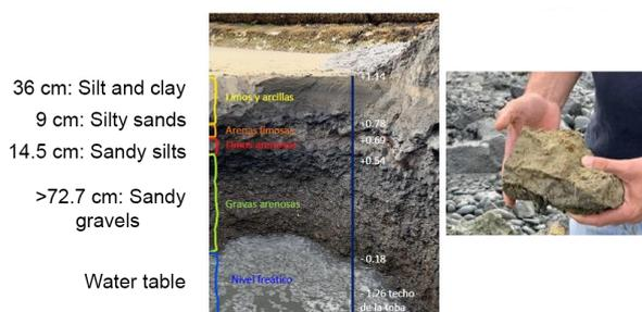
**Figure 3.3:** Ground layers (left) and tuff stone (right) (Serman y Asociados s.a., 2019)
