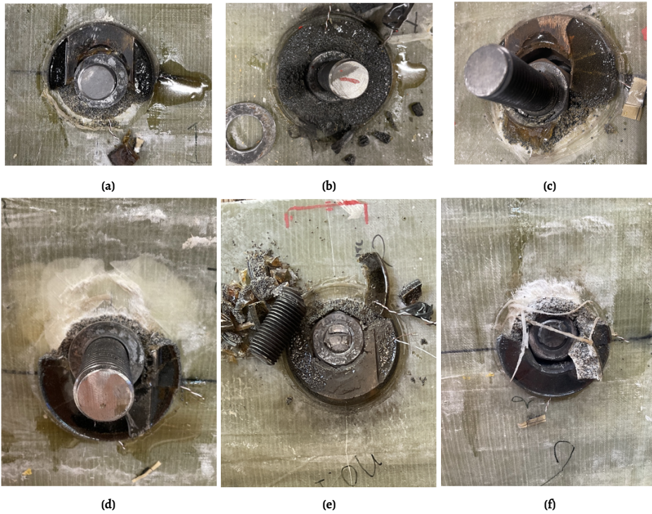
Figure 6.13: Damages of composite deck and SRR piece with or without bolt shear failure of iSRR connectors: (a) S-40-RT-U-2-B, (b) S-60-ET-U-1-B, (c) S-40-ET-U-1-B, (d) S-40-RT-U-2-T, (e) S-60-ET-U-1-T, (f) S-60-ET-U-2-T.
