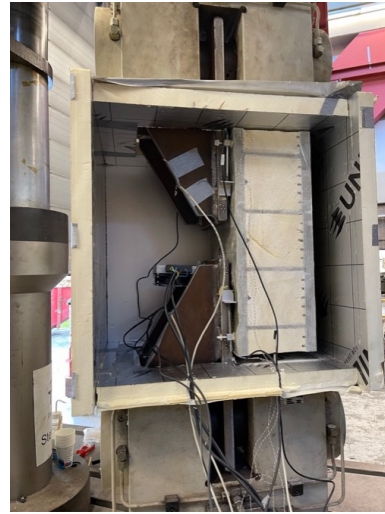
Figure 5.13: Test set-up of cyclic and static tests under elevated temperature: (a) Schematic view of the chamber, (b) Open chamber.
