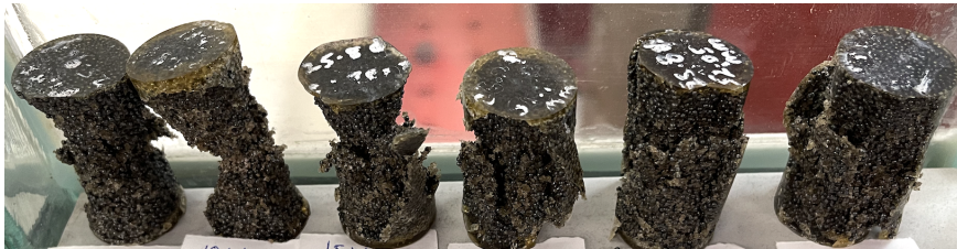
Figure 4.12: Failure mode of SRR material under cyclic uniaxial compression (fatigue).
