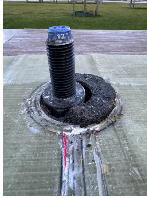
Figure 6.16: Failure mode of re-tested iSRR connector subjected to fully reversed cyclic loading.
