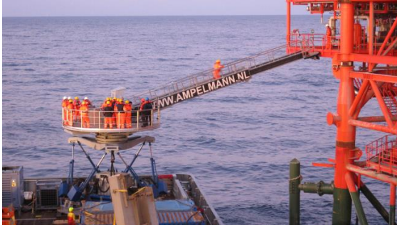
(a) The Ampelmann system is built to compensate the motion of the vessel to safely transfer employees and supplies. It consists of six hydraulic cylinders that compensate 6 degrees of freedom. The cylinders react on the motions of the barge and stroke in order to keep the platform stabilized. Therefore, this is an active heave compensation system.
