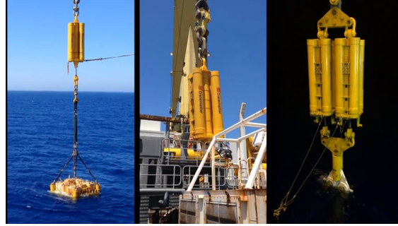
(b) A crane-master is placed between a crane and the load, the system is then tuned to compensate to motions of the crane. This enables a constant hoist speed and decreases the impact loads. With the tuning of the system the dynamic characteristics of the crane-master are changed such that the motions are cancelled adequately. No power is added to the system, hence, this is a passive heave compensation system.
