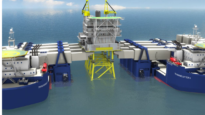
Figure 1.3: The twin marine heavy lift system, from (TMHL). The two vessels lift the topsides simultaneously using the buoyancy tanks, extra contra weight is created by ballasting the outer tanks (not visible in this illustration).
