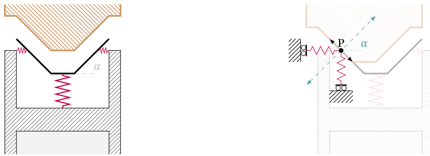
(a) Modelled representation of the LMU based on the literature and the schematics of Figures 3.4a and 3.4b. This is used as an input to derive the model for the impact conditions.
