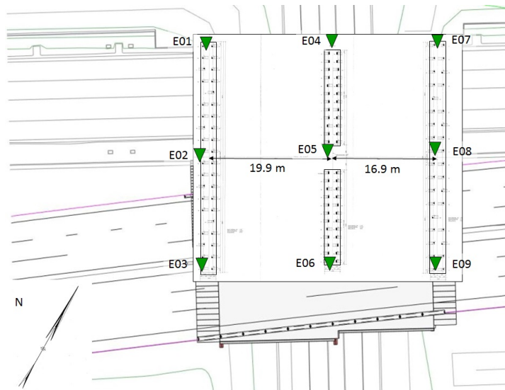
FIGURE B.11: Top view of the existing pile plan of viaduct KW150 and the locations of the old CPT set [bron]
