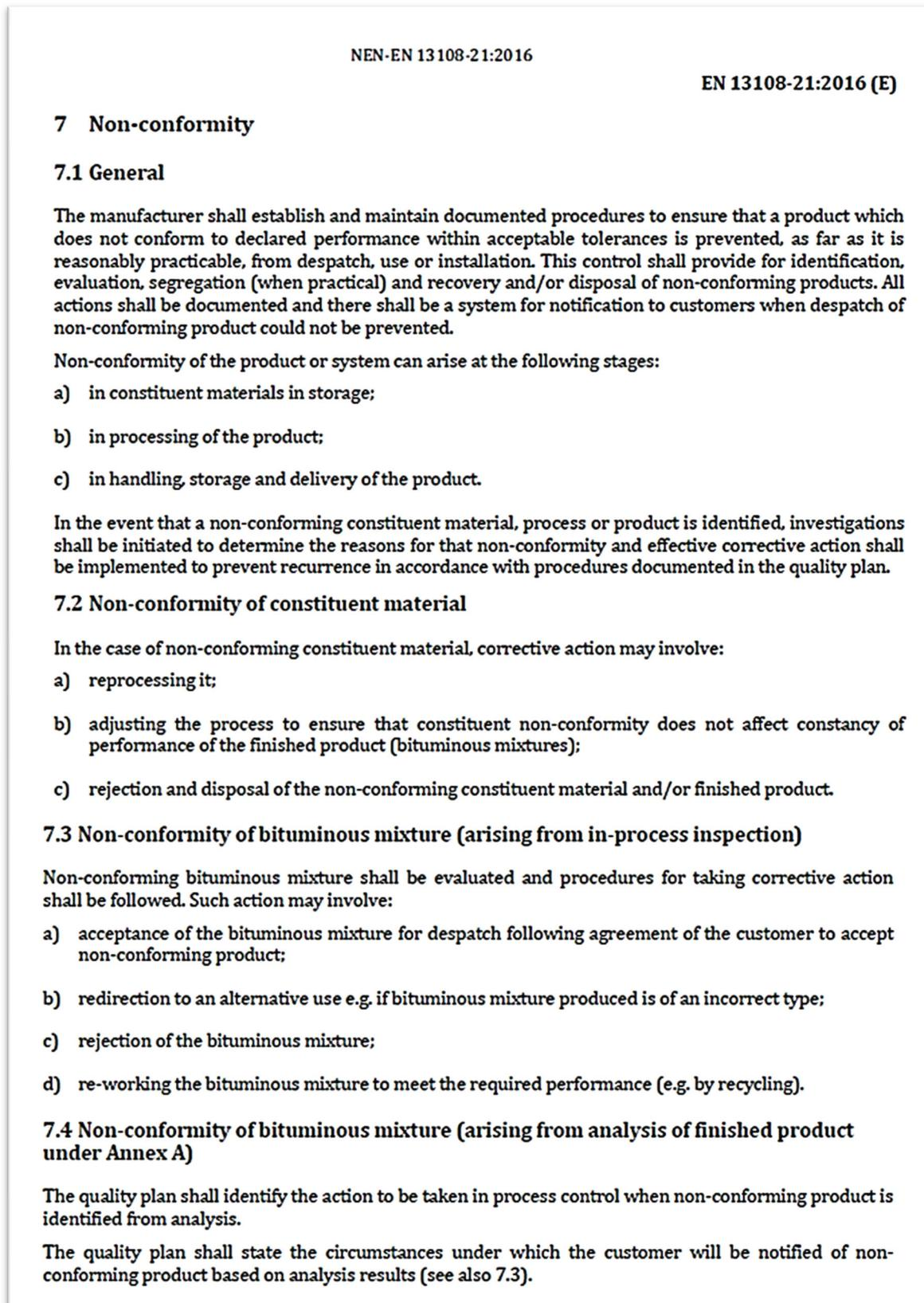
Figure 2.24: FPC non-conformity requirements (EN 13108-21 version 2016)
