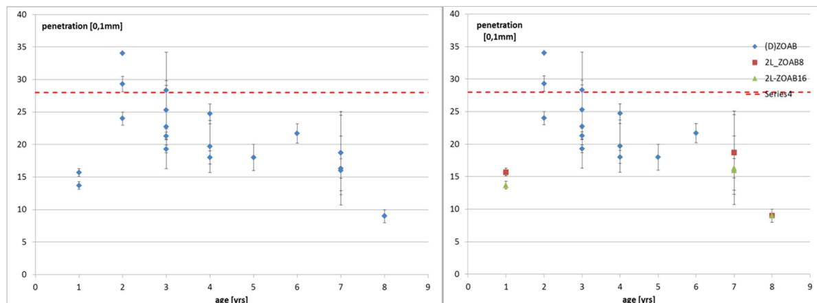
Figure 3.22: Penetration as a function of age for all sections (left) and with the different types of PA indicated (right)
