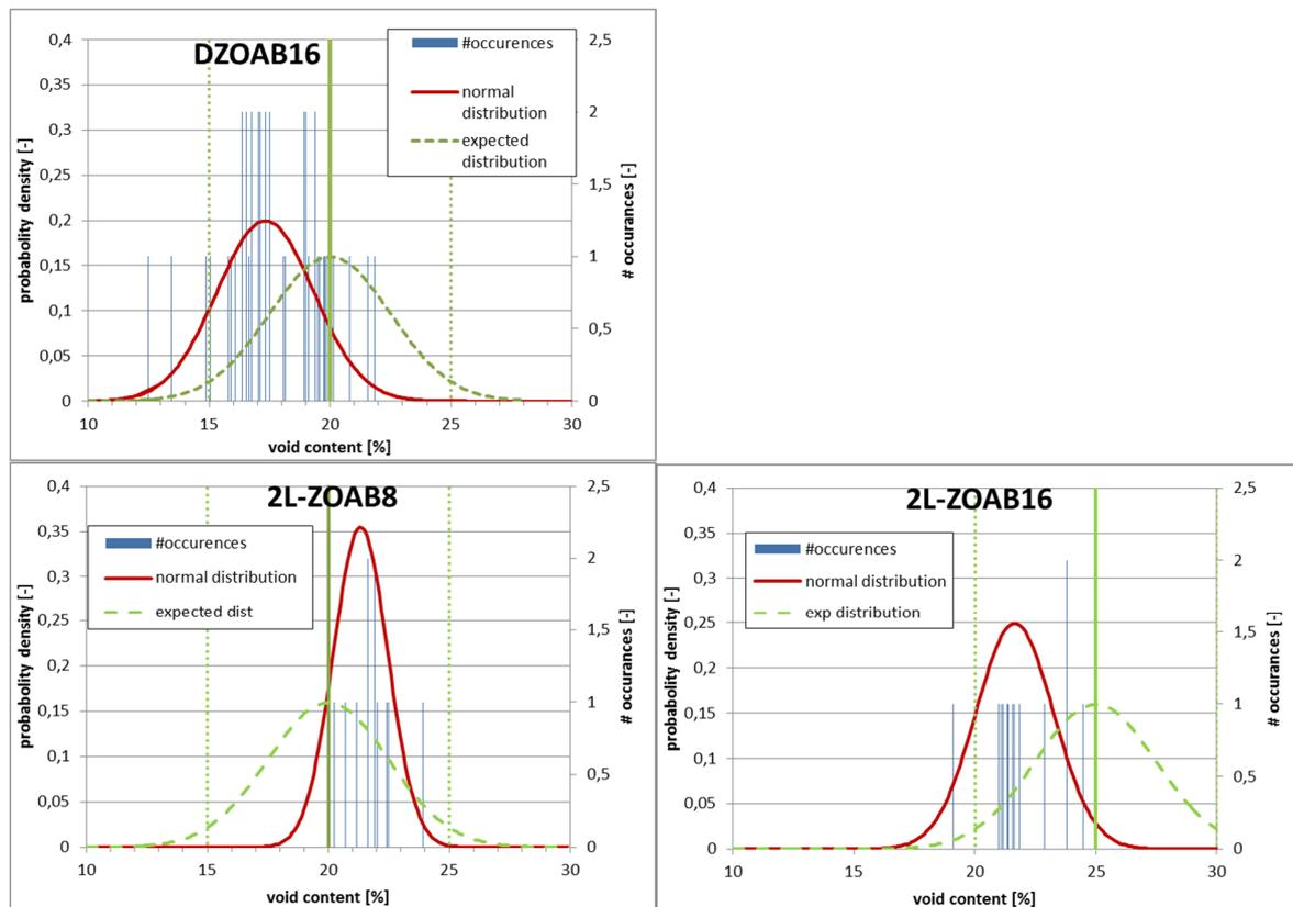
Figure 3.11: Distribution (lines, left axis) and occurrence (columns, right axis) of void content for the three types of mixtures
