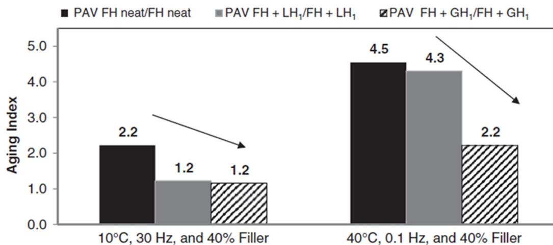
Figure 3.35: Ageing indices of neat bitumen (FH: Flint Hills PG64-22) and mastics prepared with FH neat bitumen and limestone (LH<sub>1</sub> at 40% by volume) or granite (GH<sub>1</sub> at 40% by volume) filler (Moraes & Bahia 2015a).
