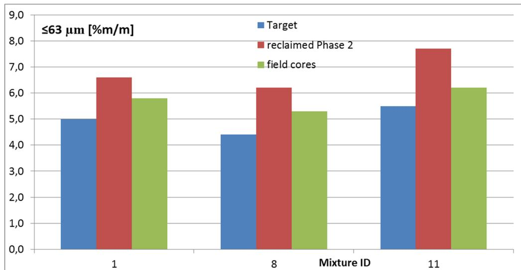
Figure 3.50: Target and realized amount of fines for Phase 2 and field cores
