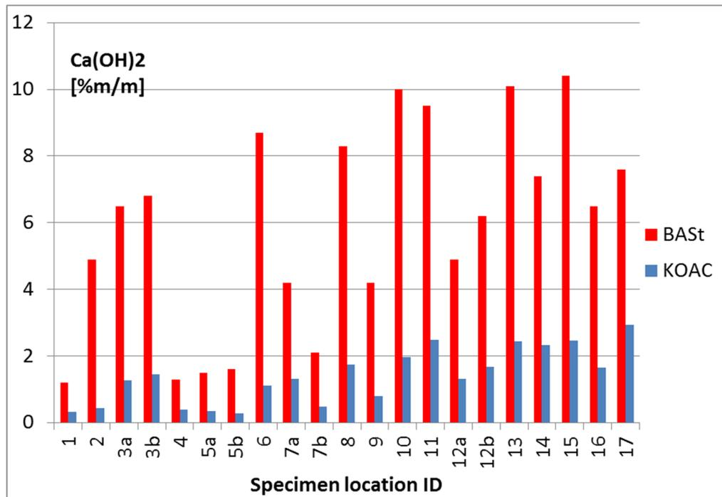
Figure 3.47: Results on the hydrated lime content determined with titrimetry from BAST and Kiwa KOAC
