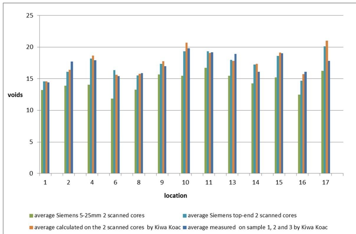
Figure 3.17: Calculated overall void content and void content over part of the height from the scans of DZOAB 16 samples compared to the calculated and measurement values by Kiwa KOAC
