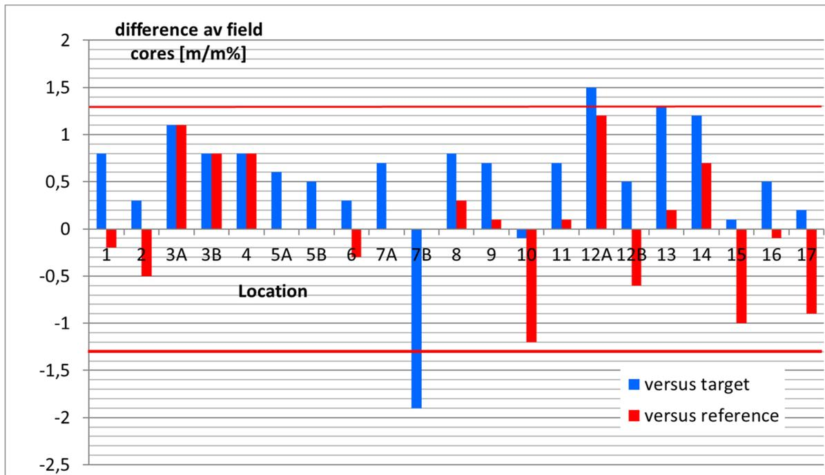
Figure 3.13: Difference in m/m% material  $\leq 0,063\text{mm}$  in the field cores vs target and reference composition
