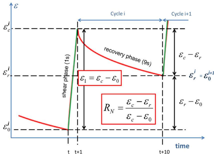
Figure 3.24: Data analyses principle used in the MSCR test Hirsch, 2017a, with some additions
