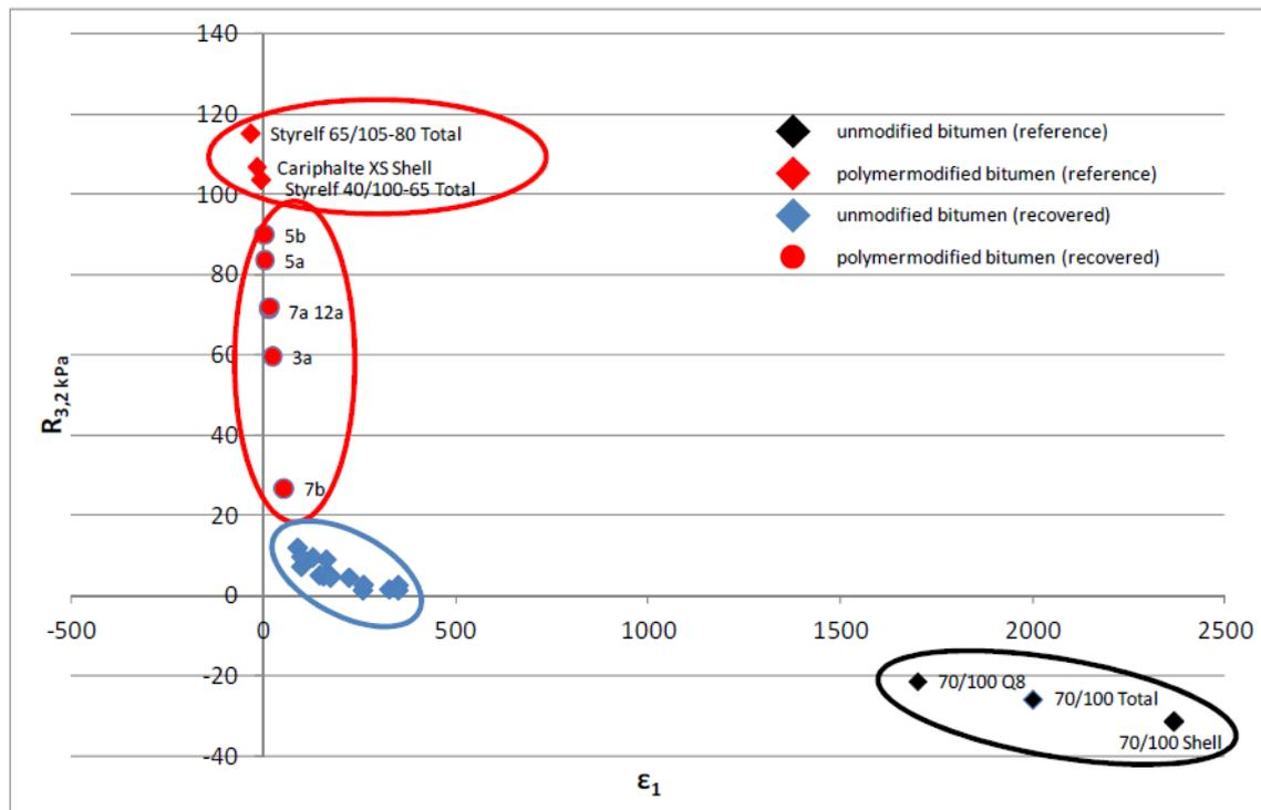
Figure 3.26: Graphical representation of the results from the MSCR test (Hirsch, 2017a)
