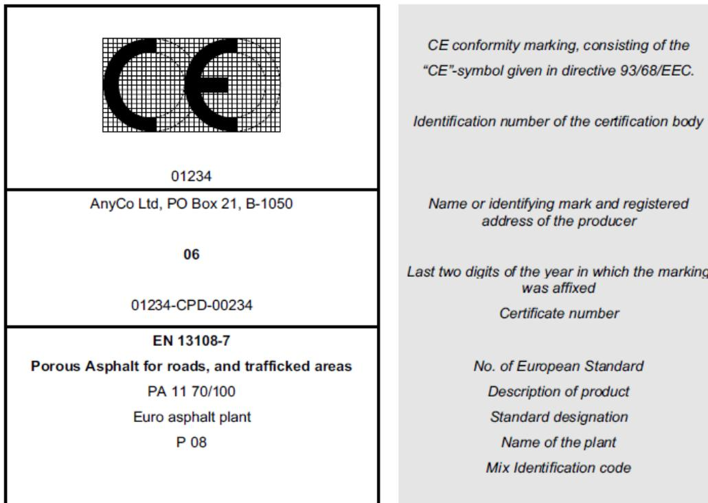
Figure 2.10: Example of the delivery ticket (Fig. ZA.1b of EN 13108-7:2006)
