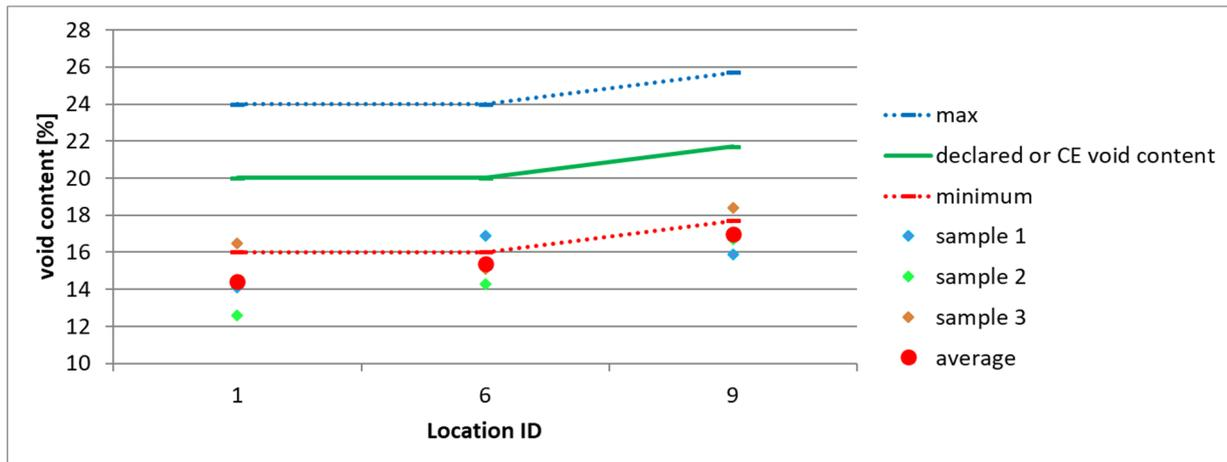
Figure 3.12: Individual results and requirements for three locations (L1, L6 and L9)
