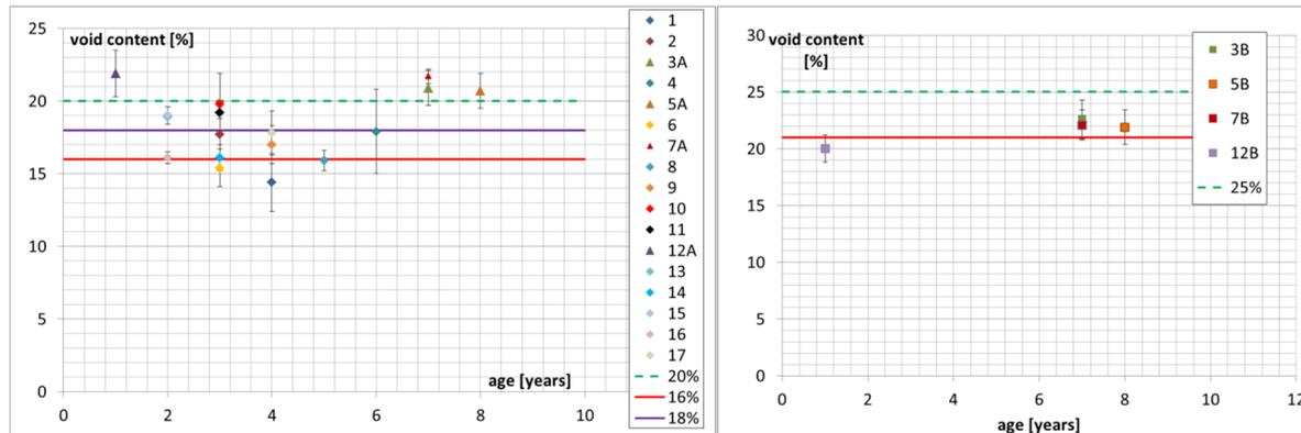
Figure 3.10: Average void content versus the age of the sections (at the time of sampling in 2016), left DZOAB 16 and 2L-ZOAB 8, right 2L-ZOAB 16
