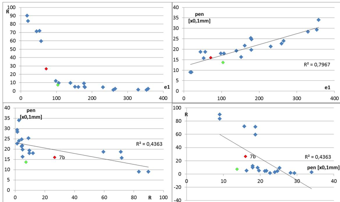
Figure 3.28: Plotting  $\epsilon_1$ , R and penetration versus each other in various combinations, green marker=12B, red=7B
