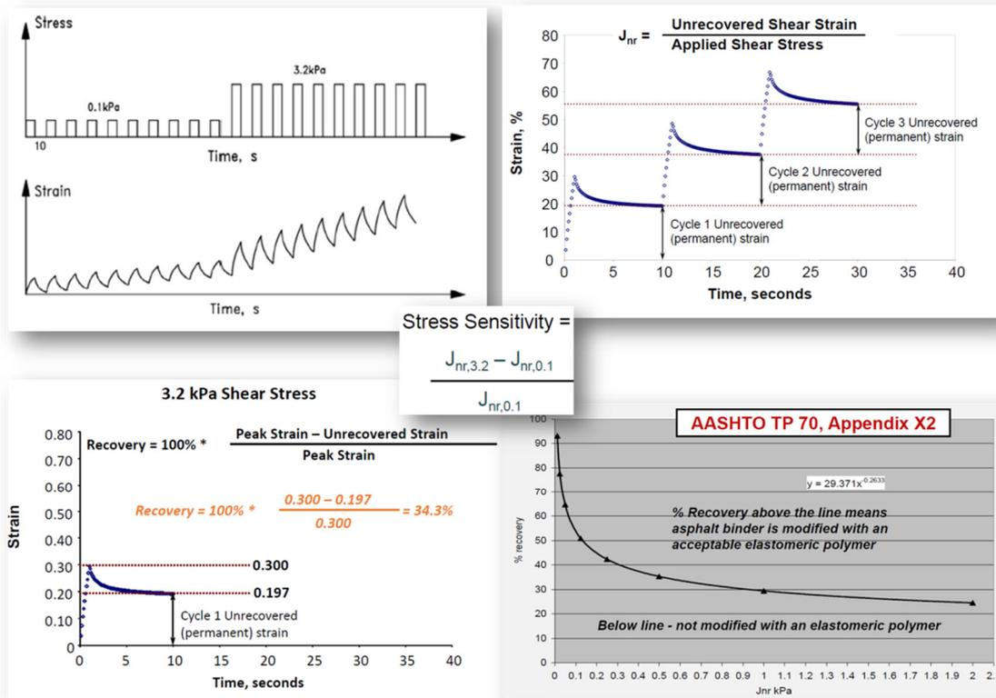
Figure 3.25: MSCR test principle (AASHTO TP70)
