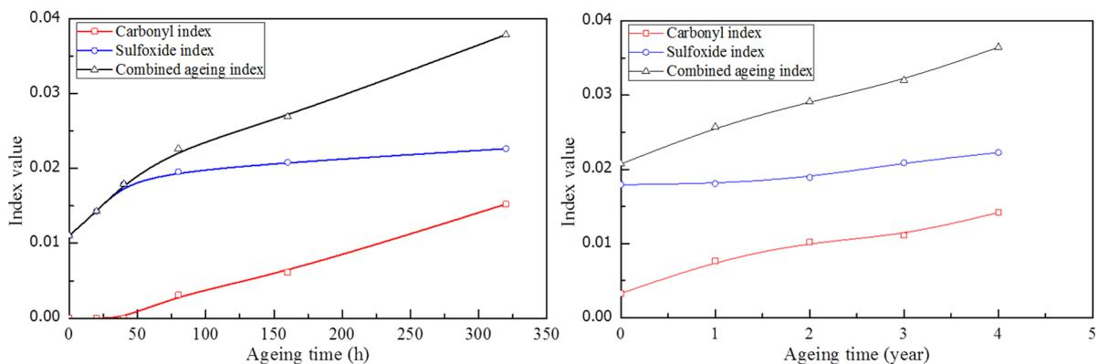
Figure 3.53: C=O and S=O development during aging in the lab (left) and in the field (right) Jing, 2019
