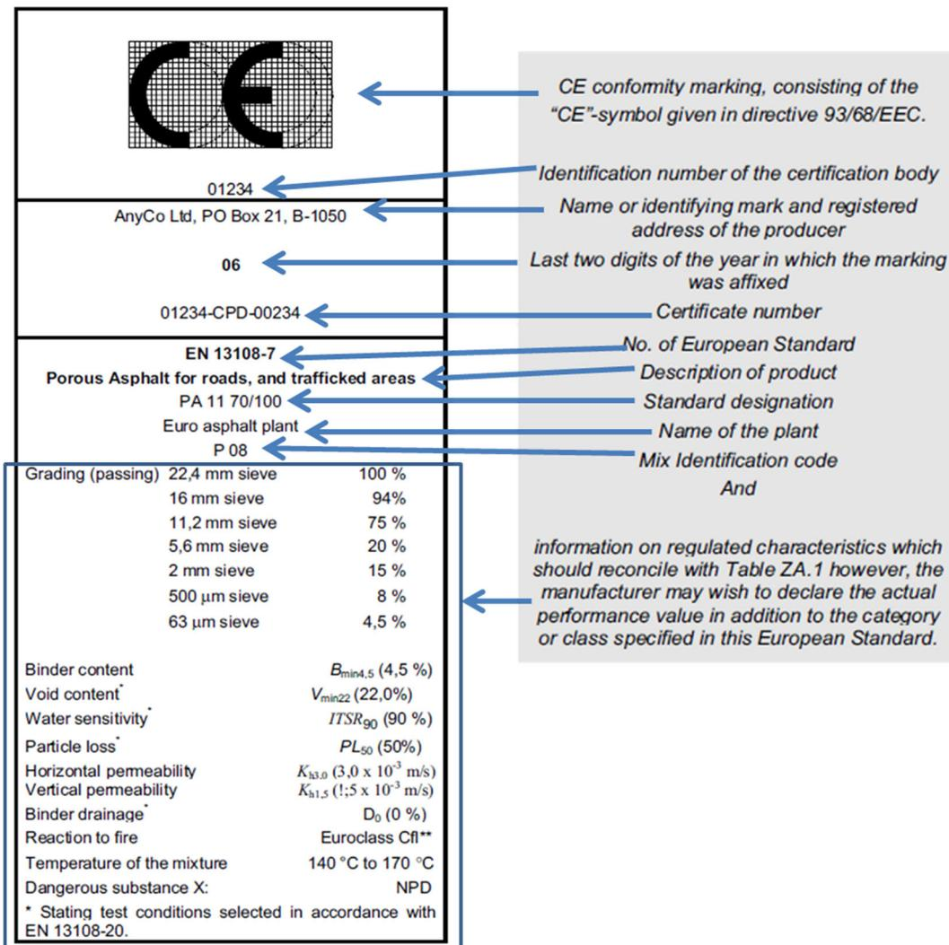
Figure 2.11: Example of CE marking given in Annex ZA EN 13108-7:2006 as Figure ZA.1a
