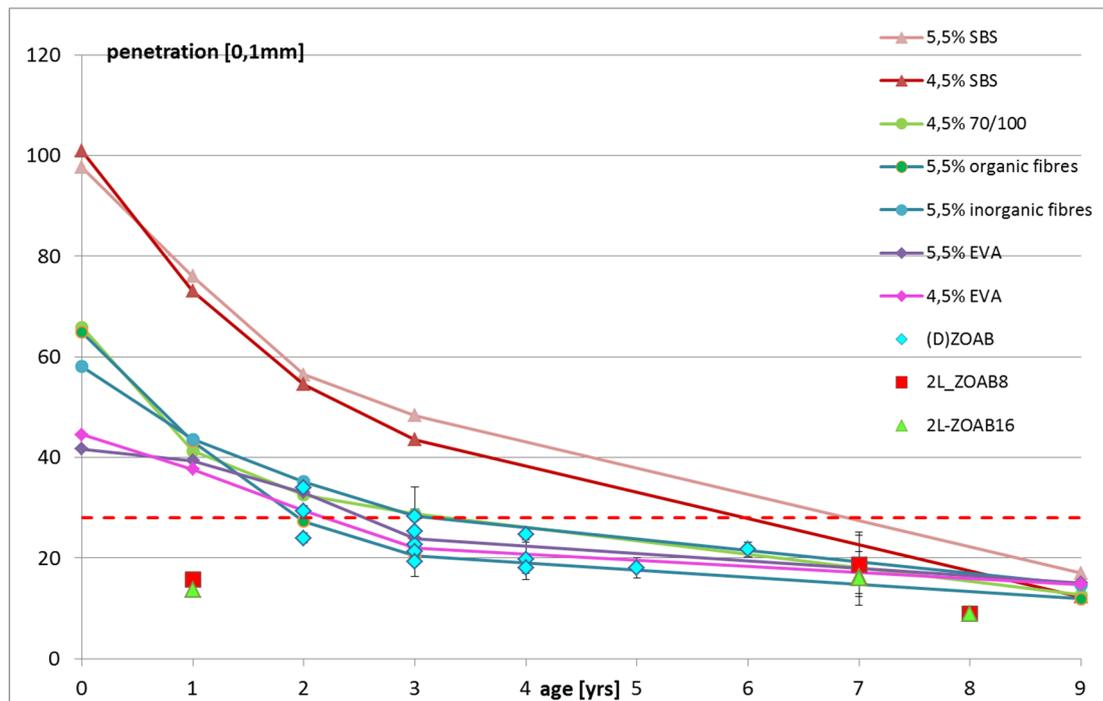
Figure 3.23: A selection of the penetration over time results from Voskuilen et al. (2004) combined with the values found for the cores from the road sections in this project
