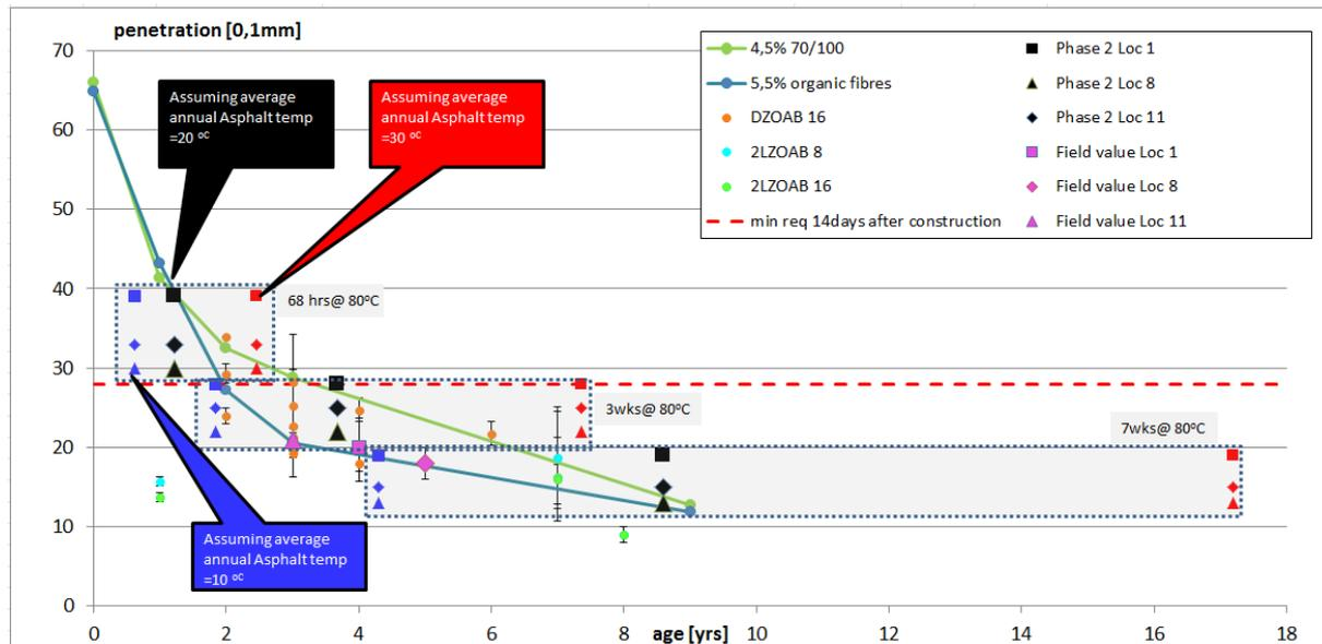
Figure 3.51: Adding the penetration values from phase 2 to Figure 3.2334
