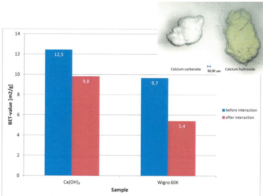
Figure 3.42: Change in surface area of the filler after interaction with bitumen and the visibly remaining bitumen coating on the filler particles Hirsch, 2017c
