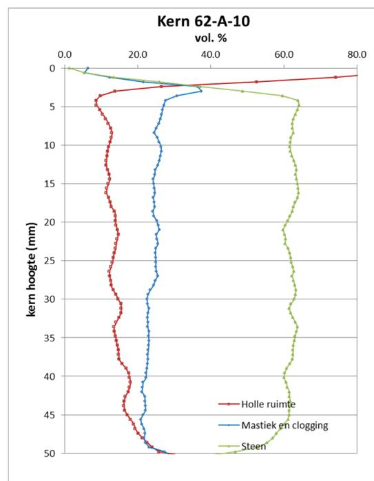
**Figure 3.16: Low percentage of voids at the top increasing with depth. Increasing percentage of mortar with depth**
