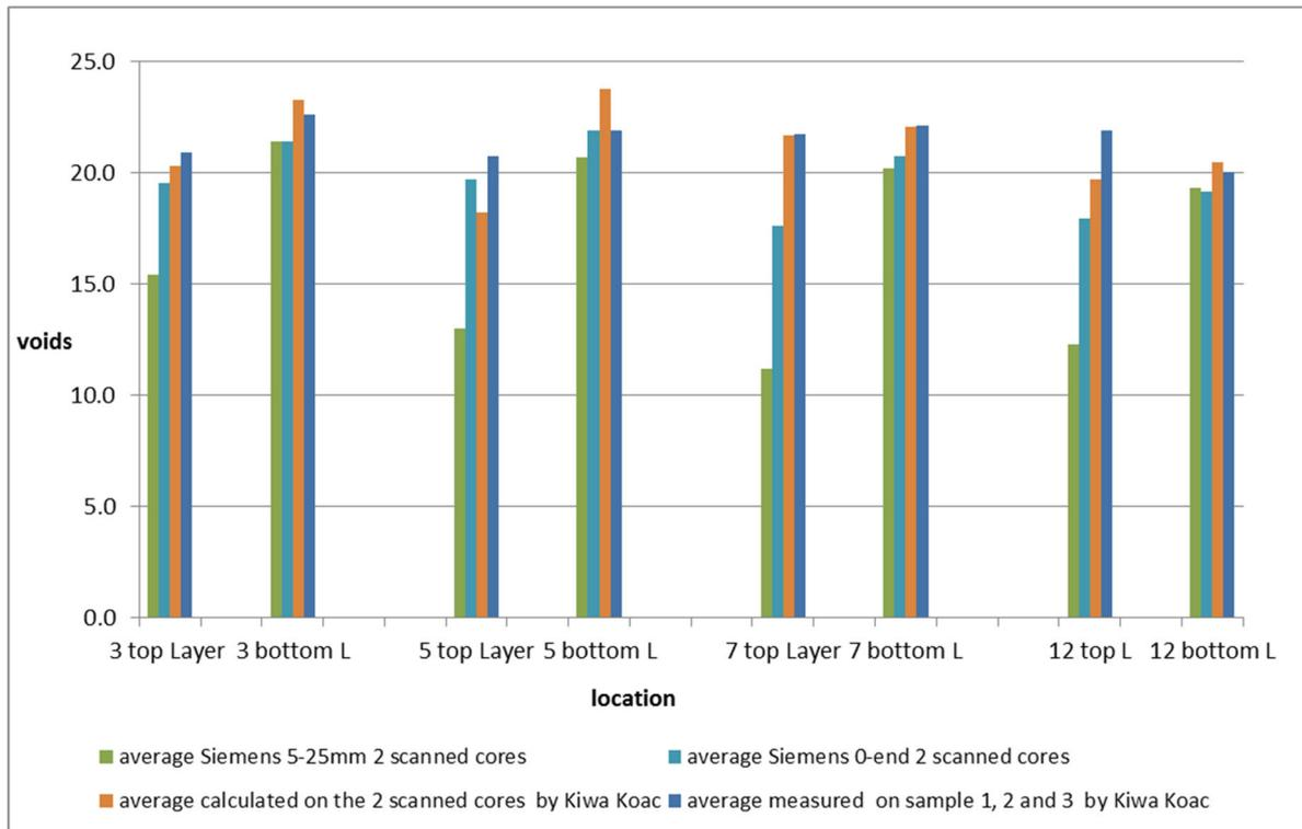
Figure 3.18: Calculated overall void content and void content over part of the height from the scans of 2L-ZOAB 8 and 16 samples compared to the calculated and measurement values by Kiwa KOAC
