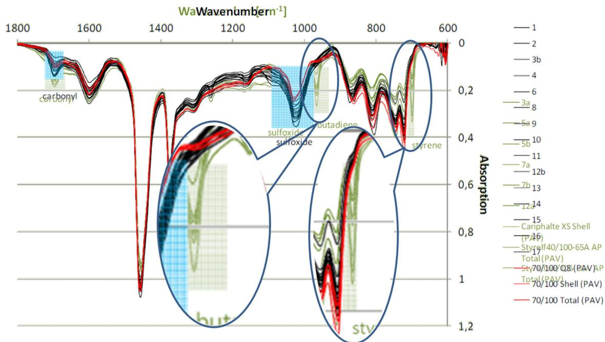
Figure 3.30: Combined signals for aged PMBs and pen grade bitumen from Hirsch, 2017a
