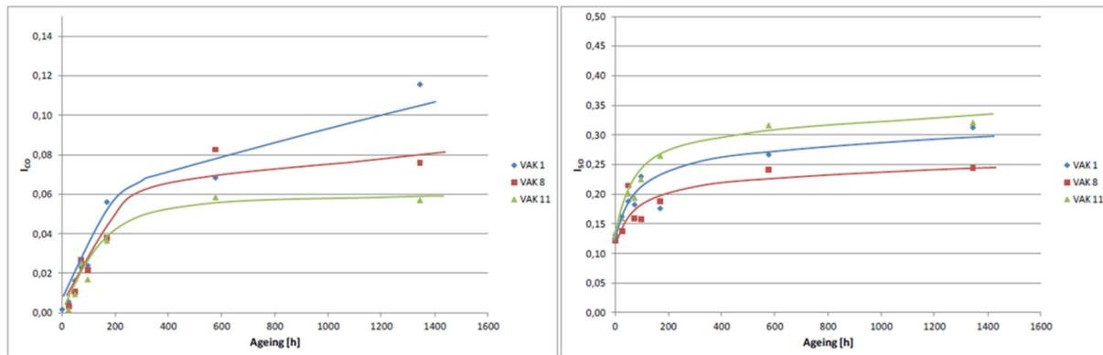
Figure 3.54: C=O (left) and S=O (right) development during lab aging according Voskuilen, 2019
