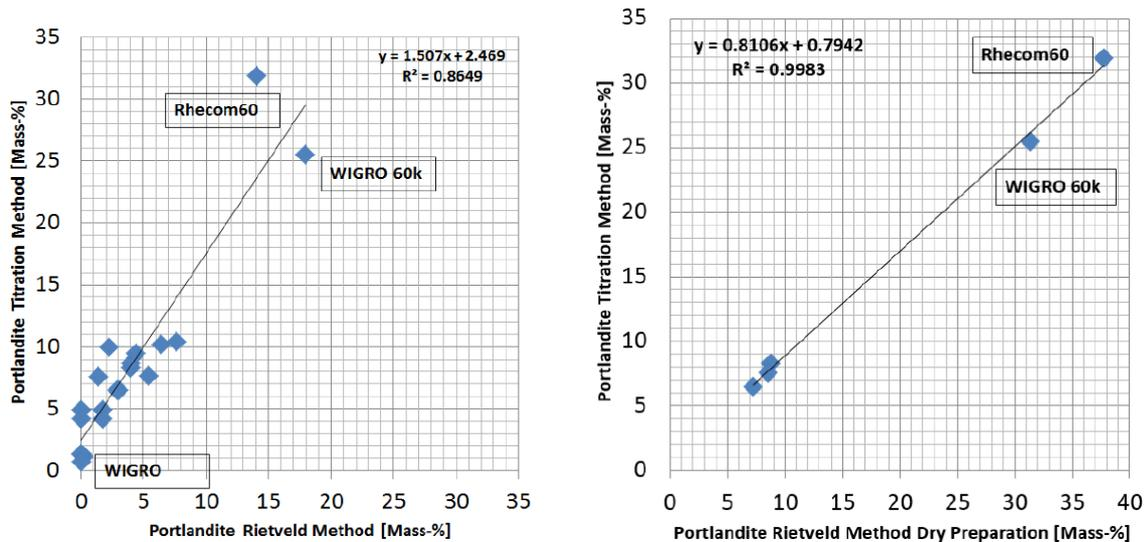
Figure 3.46: XRPD using Rietveld method comparison of  $\text{Ca}(\text{OH})_2$  content Hellman, 2018b compared to tritration Hirsch, 2017b for the wet (left) and dry (right) preparation method in XRPD Hellman, 2018b
