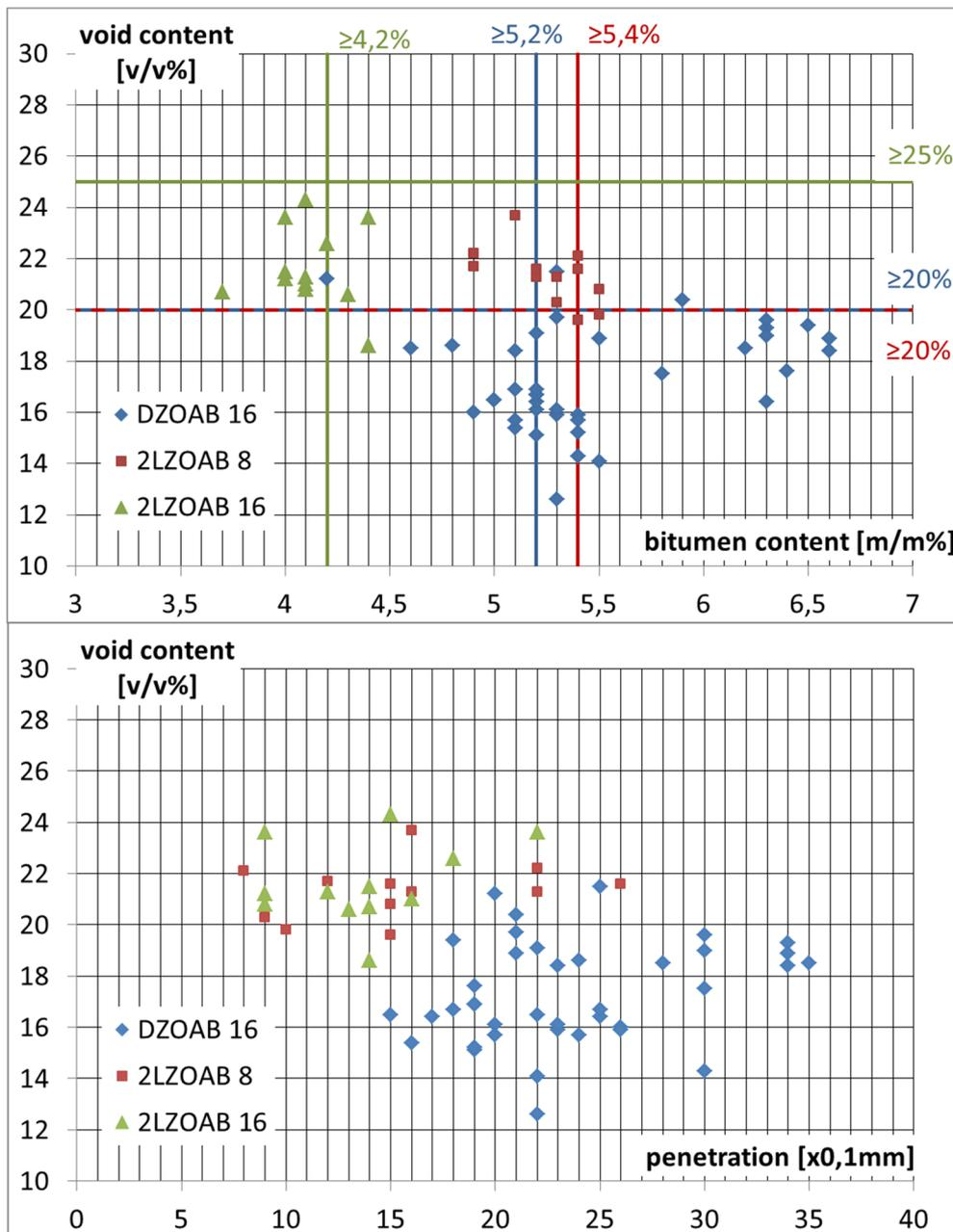
Figure 3.14: Plot of the void content versus bitumen content(top) and versus penetration of the bitumen (bottom), distinguishing the three groups of mixtures
