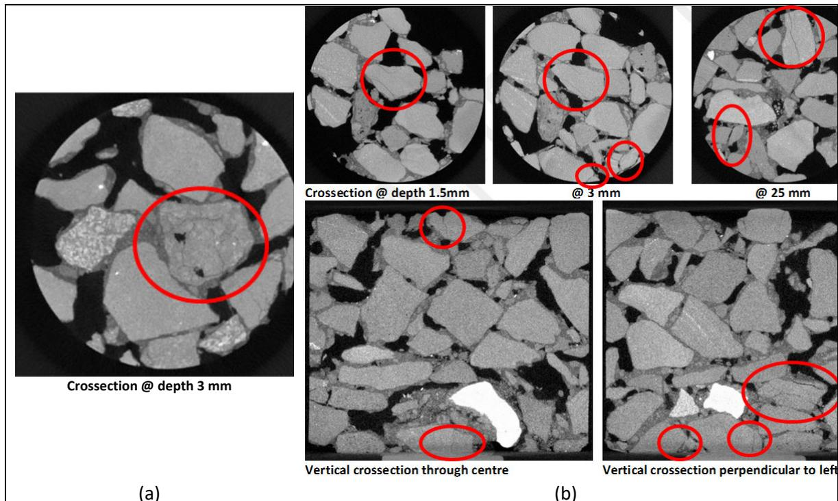
Figure 3.63: Example of (a) weathering patterns (location 17) and (b) cracks (location 9)
