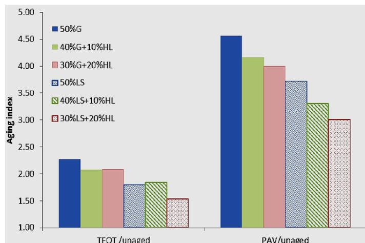
Figure 3.36: Ageing indices of granite and limestone mastics with and without the addition of hydrated lime. Two ageing conditions were considered: TFOT ageing at 163°C for 5 hours and PAV ageing for 20 hours at 90°C following the TFOT27 oven ageing. (Alfaqawi et al., 2017).
