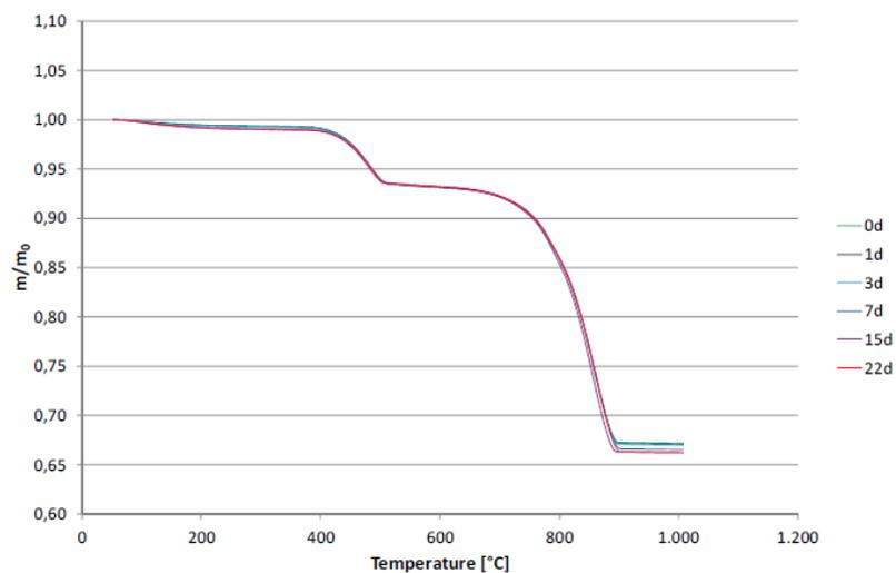
Figure 3.39 Thermogravimetry (TGA) analysis results of Wigro 60K (25%  $\text{Ca}(\text{OH})_2$ ) over a period of 22 days under laboratory conditions Hirsch, 2017c
