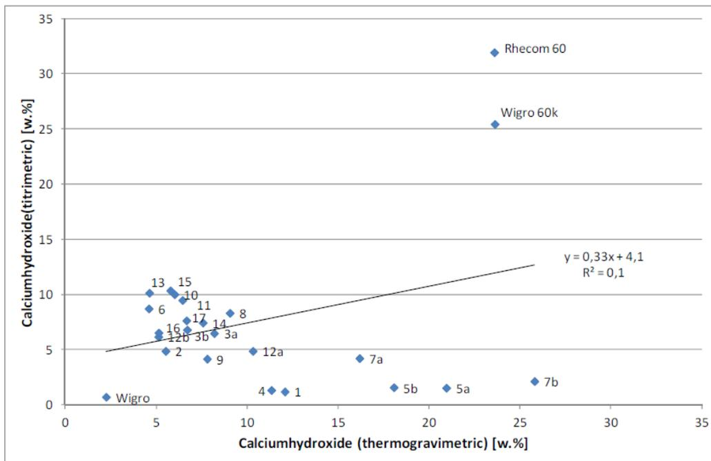
Figure 3.44: Comparison of the Ca(OH)<sub>2</sub> content found using titrimetry and thermography Hirsch, 2017b
