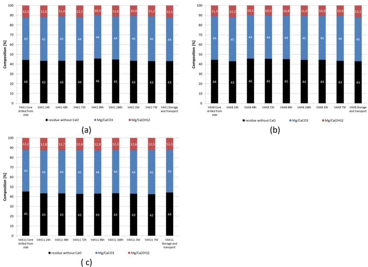
Figure 3.56: Titrimetry results for the lab aged mixtures and field cores for location 1 (a), 8 (b) and 11 (c)
