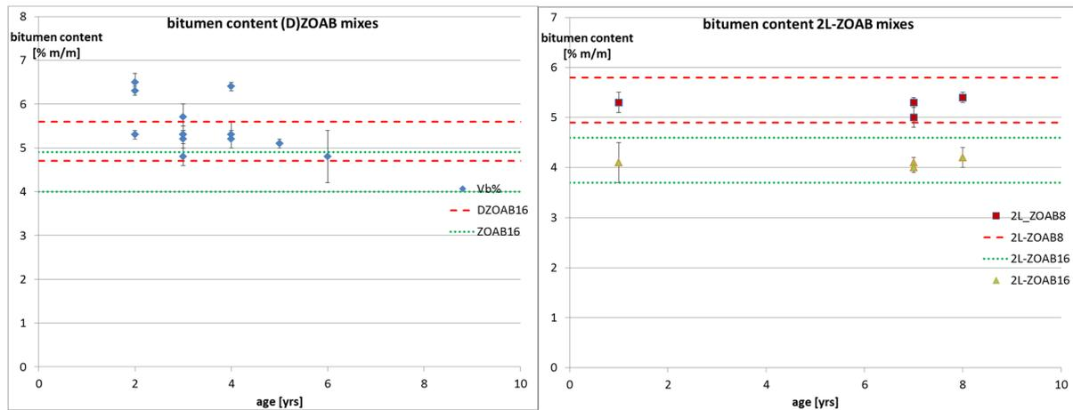
Figure 3.19: Bitumen content (n=3) for (D)ZOAB 16 (left) and 2L-ZOAB 8 and 2L-ZOAB 16 (right), with the corresponding margins
