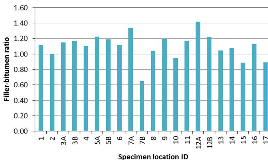
Figure 3.34: Results on the filler-bitumen ratio based on the average filler and bitumen content values in Table 3.16 and Table 3.12
