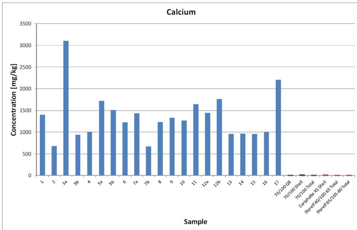
Figure 3.32: Calcium content in the reclaimed and reference bitumen
