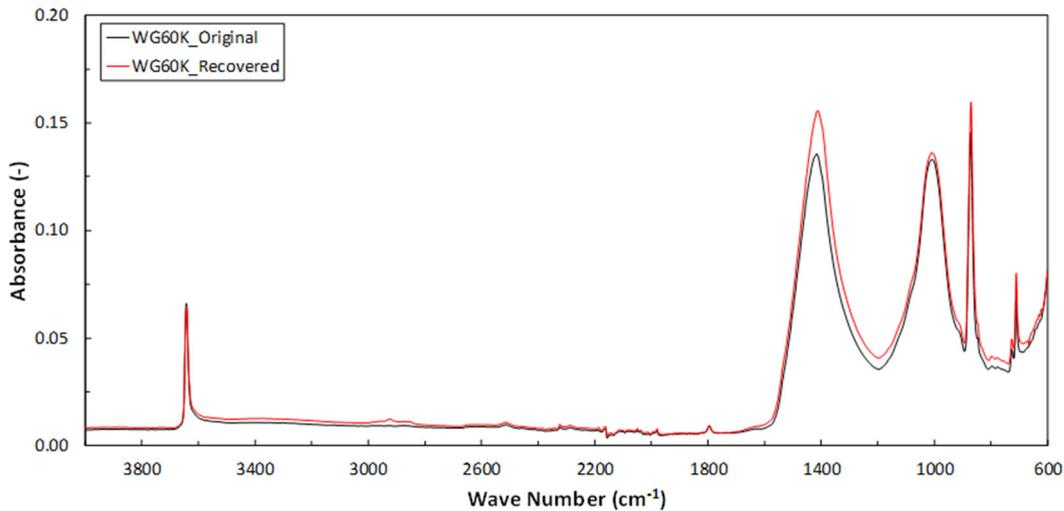
Figure 3.40: Fourier Transform infrared (FT-IR) spectra of the original and recovered (after PAV ageing) mineral filler Wigro 60K Mastoras, 2019
