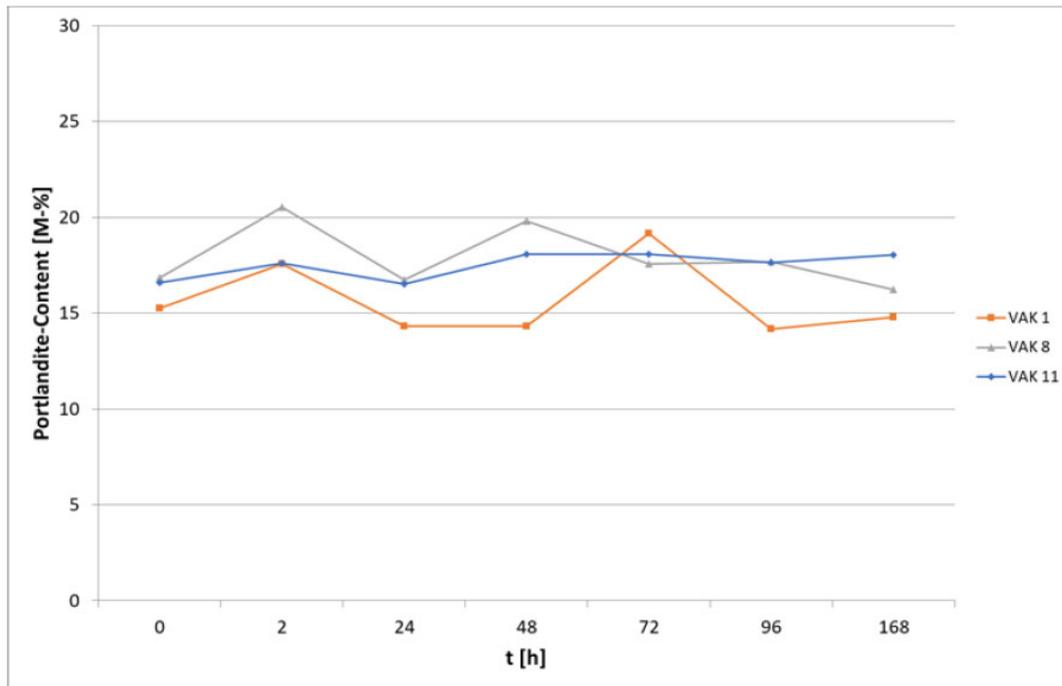
Figure 3.55:  $\text{Ca}(\text{OH})_2$  content found from XRPD on dry-prepared specimens in various stages of aging (Table 3.23) reproduced after Hellman, 2019
