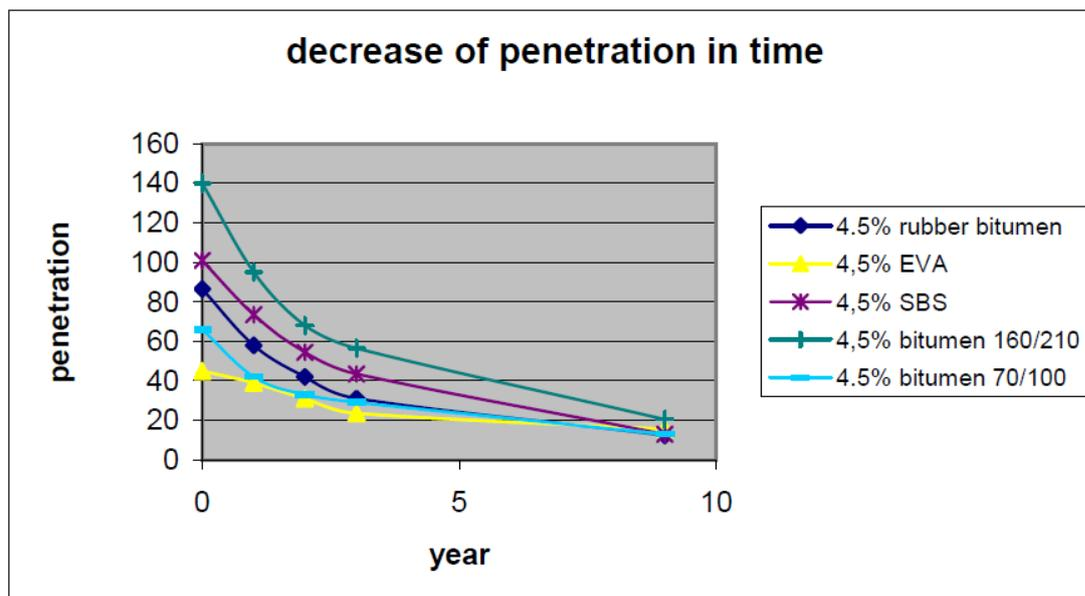
Figure 3.21: reduction of penetration of ZOAB 16 mixtures over time (after: Voskuilen et al., 2004)<sup>21</sup>
