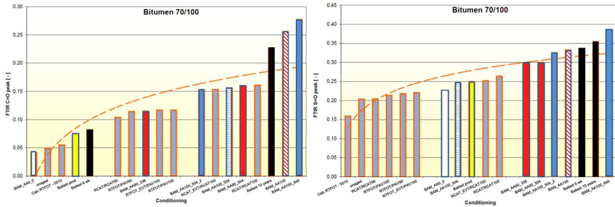
Figure 3.52: C=O and S=O ratio ranking for various aging conditions (lab and field), Besamusca et al. (2016)
