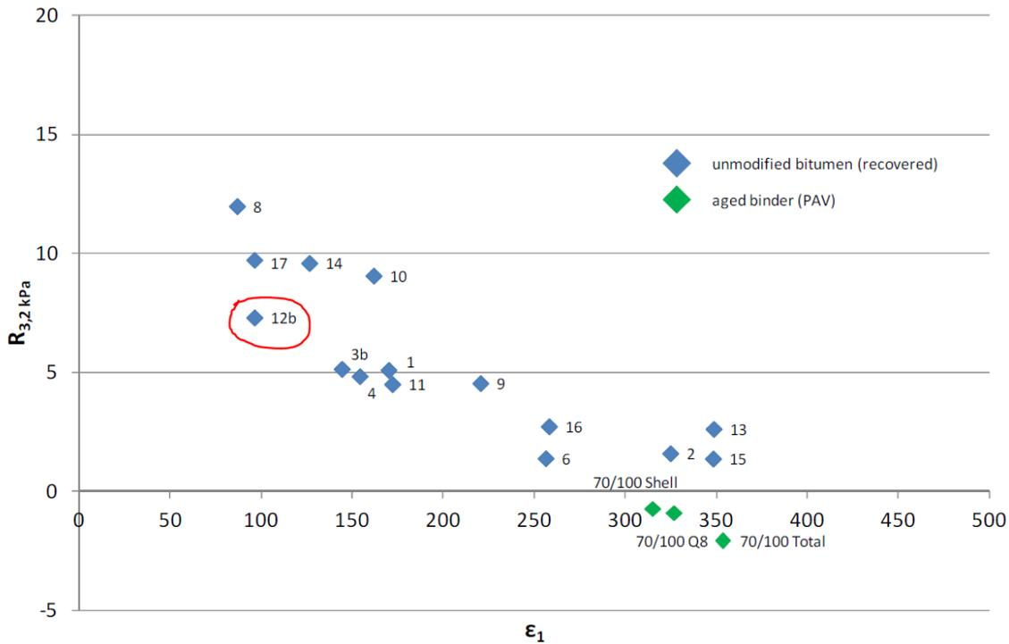
Figure 3.27: Close up of the penetration binders from the MSCR test, indicating 12B as a penetration binder
