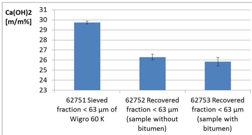
Figure 3.58: Graphical results showing Ca(OH)<sub>2</sub> content in Wigro 60K, after dry mixing and after mixing with bitumen
