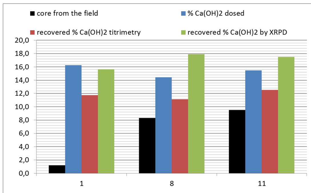
Figure 3.57: Dosed and reclaimed, through titrimetry and XRPD, respectively amounts of  $\text{Ca}(\text{OH})_2$  (Table 3.24)
