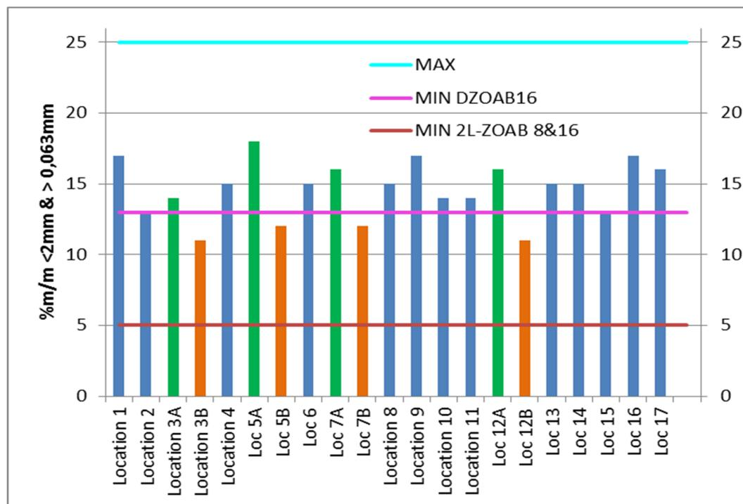
Figure 3.59: Average (n=3) sand fraction found for the various the locations (blue=DZOAB 16, green=2L-ZOAB 16, red = 2L-ZOAB 8) and the requirements for this fraction
