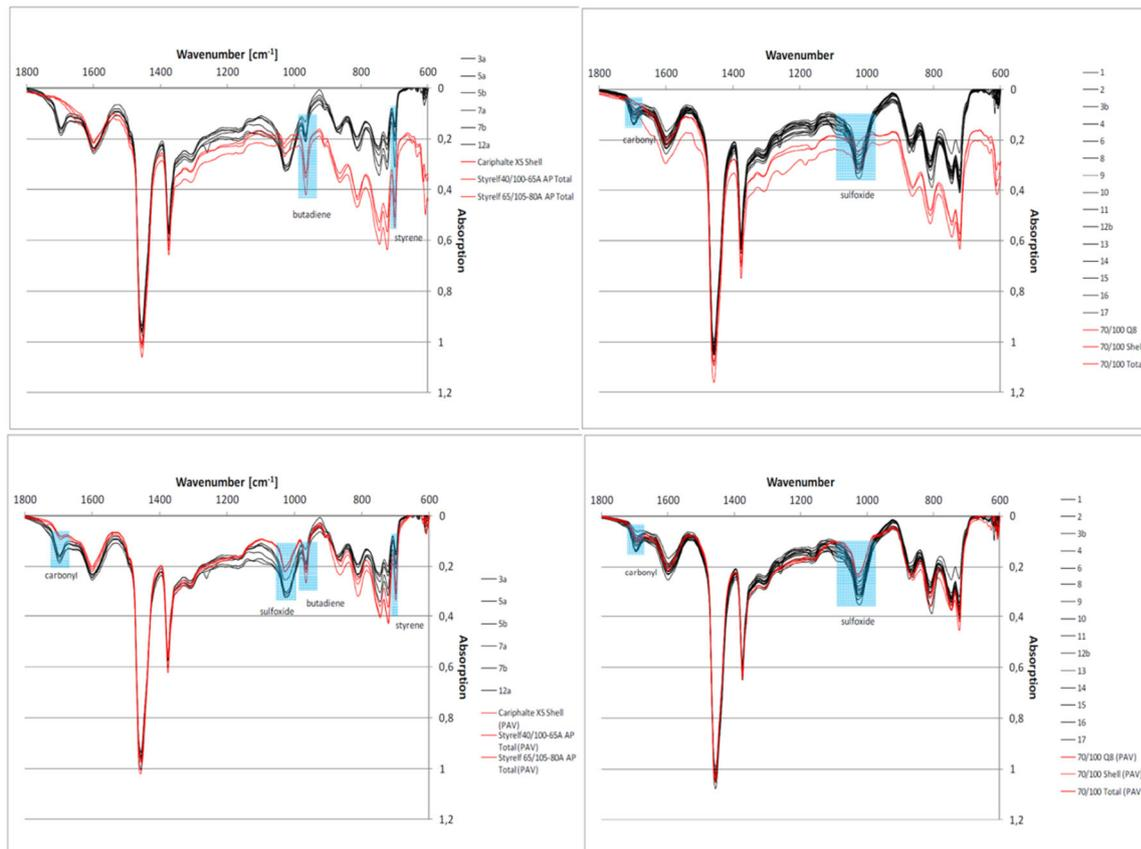
Figure 3.29: FTIR spectra, left is the PMB and right are pen graden bitumens, top are the unaged reference binders and bottom are the results from the reclaimed bitumen from the field cores (Hirsch, 2017a)
