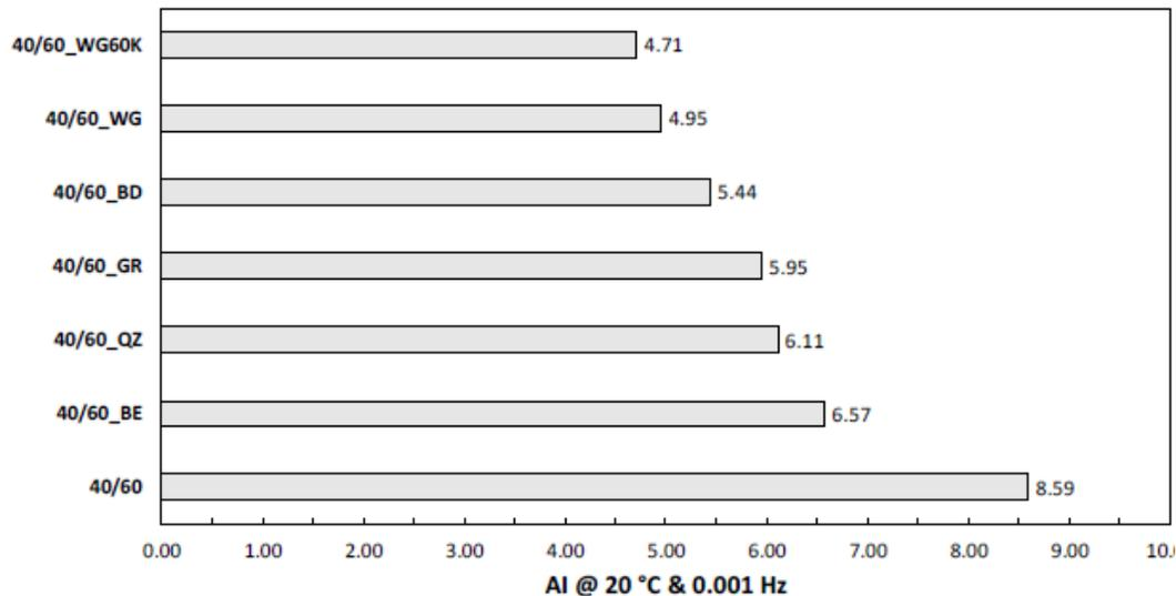
Figure 3.37: Ageing indices (AI) for mastics prepared with pen grade 40/60 bitumen and Wigro 60k (WG60K), Wigro (WG), Baghouse dust (BD), Granite (GR), Quartz (QZ) and Bestone (BE) fillers in a 1:1 ratio by mass<sup>28</sup>.
