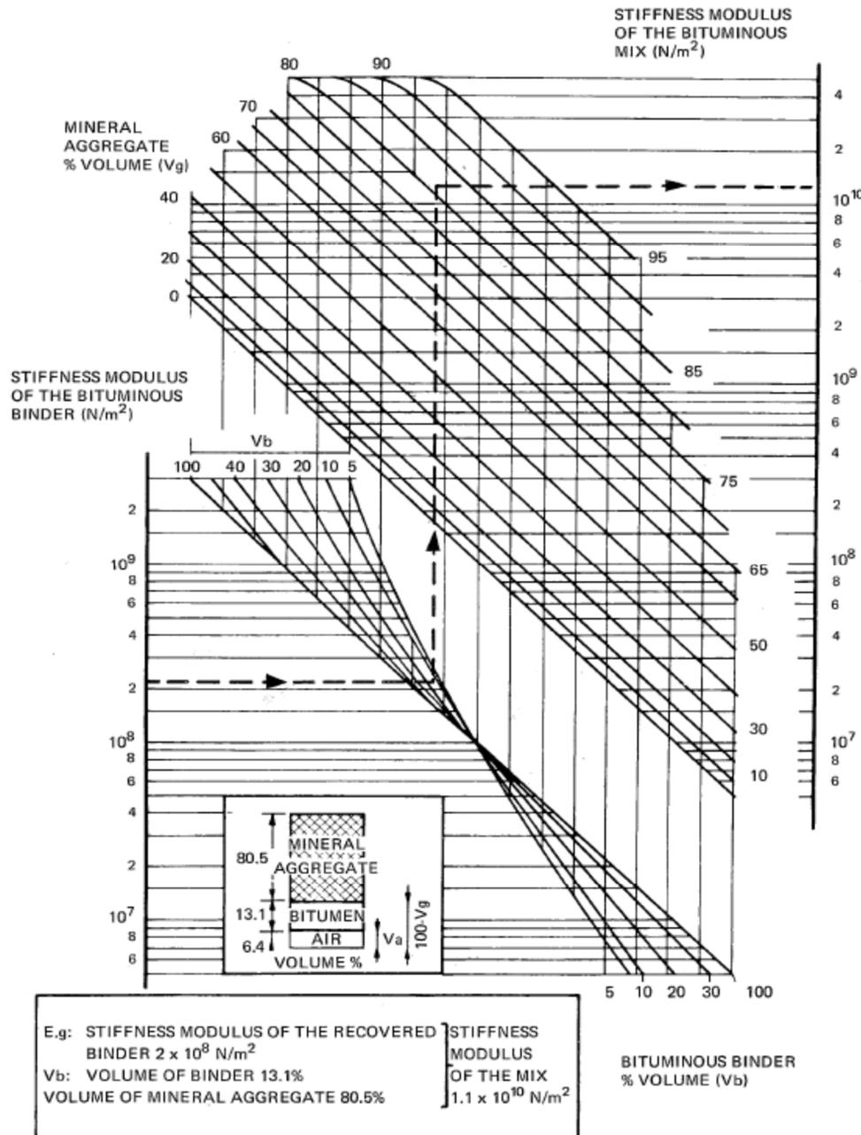
Figure 4.1: Uge nomograph, linking stiffness to volumetric mixture composition (Bonnaure, 1977)
