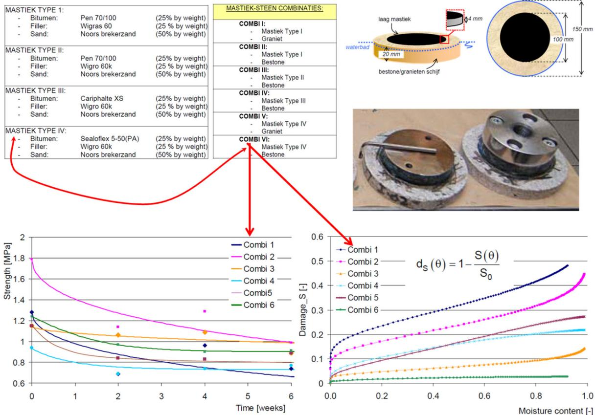
Figure 3.41: Effect of active filler on moisture sensitivity (compare combi II and III)
