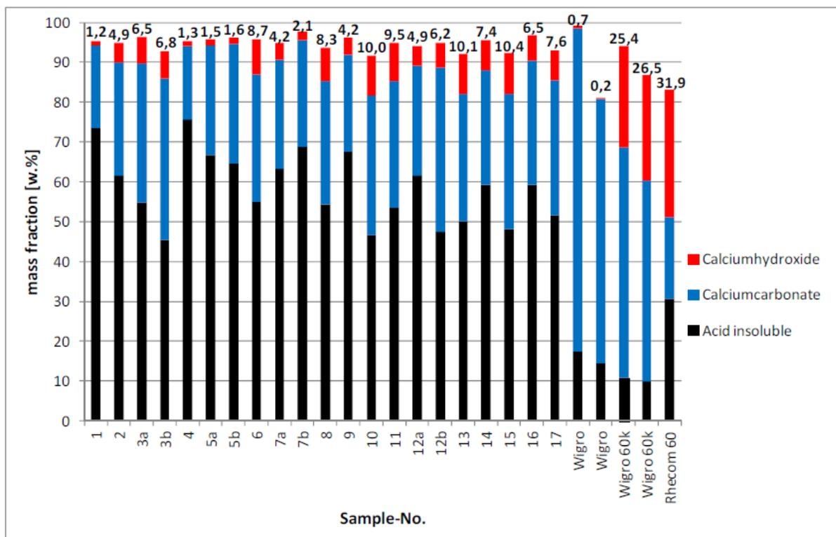
Figure 3.43: Filler composition as found from the combined titrimetric-volumetric-gravimetric methods (numbers above the columns refer to the calcium hydroxide content) Hirsch, 2017b
