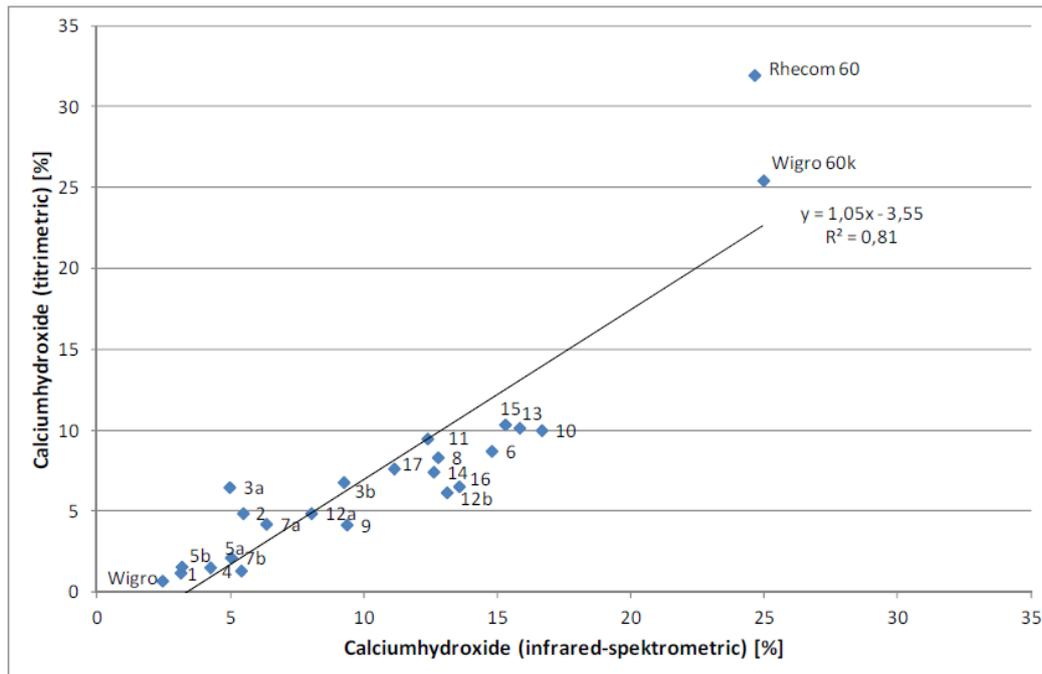
Figure 3.45: Comparison of Ca(OH)<sub>2</sub> content found using titrimetry and FTIR Hirsch, 2017b
