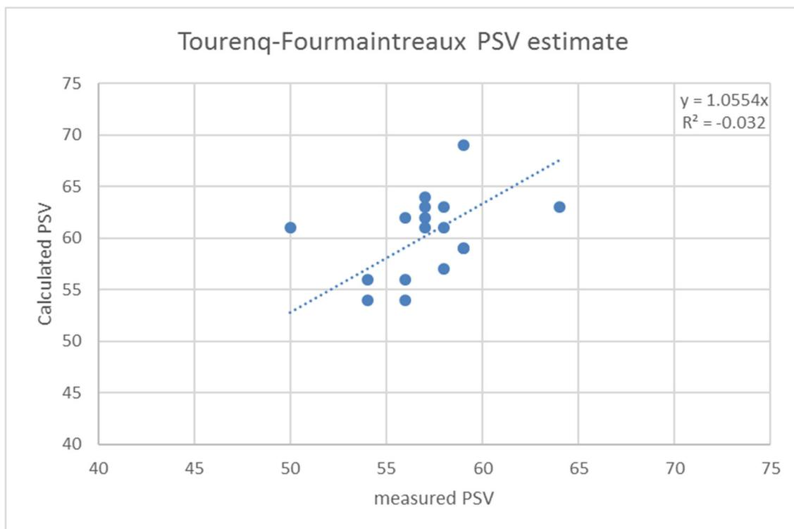
Figure 3.62: PSV calculated with the Tourenq regression equation (Tourenq et al., 1971) compared with the measured values.
