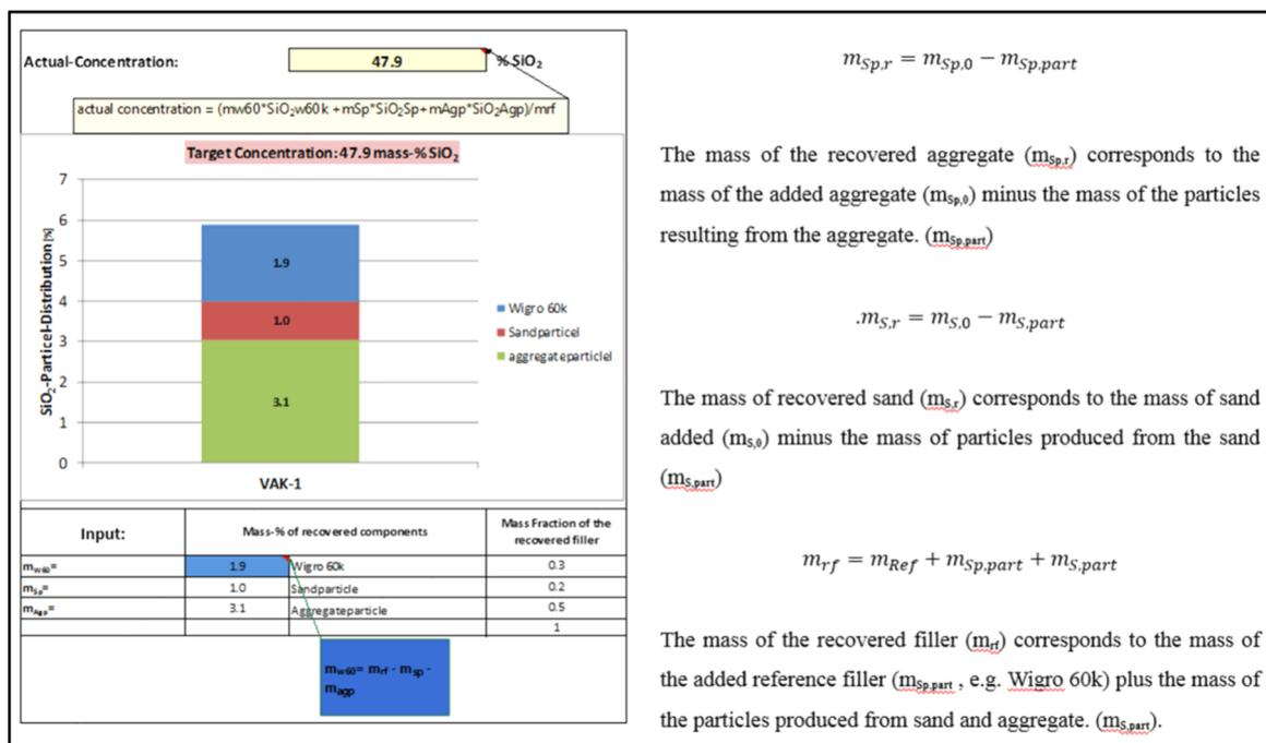
Figure 3.49: Concept of Mass Balance calculation by Core Power (presentation 21 March 2019, in Delft)
