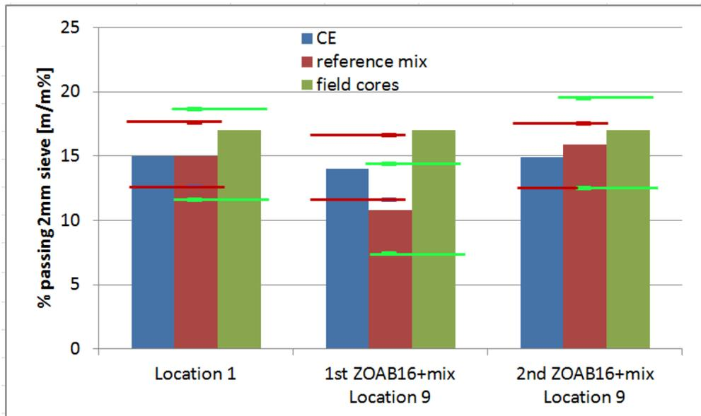
Figure 3.60: Individually declared and measured values compared to the boundaries between CE and reference composition (red) and reference composition and field values (for n=3, green)
