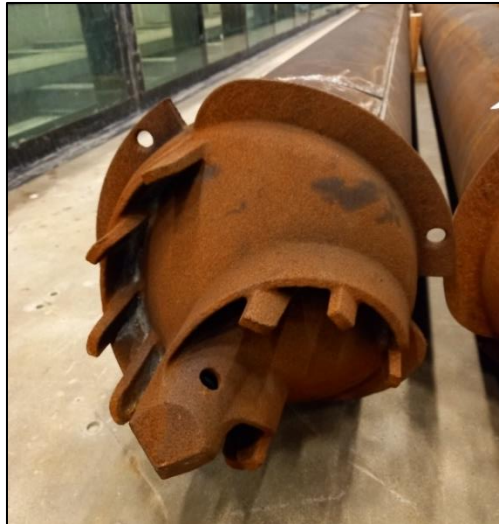
Figure 3.1: Screw tip of the SIc piles. The same tip was also used for the SI piles
