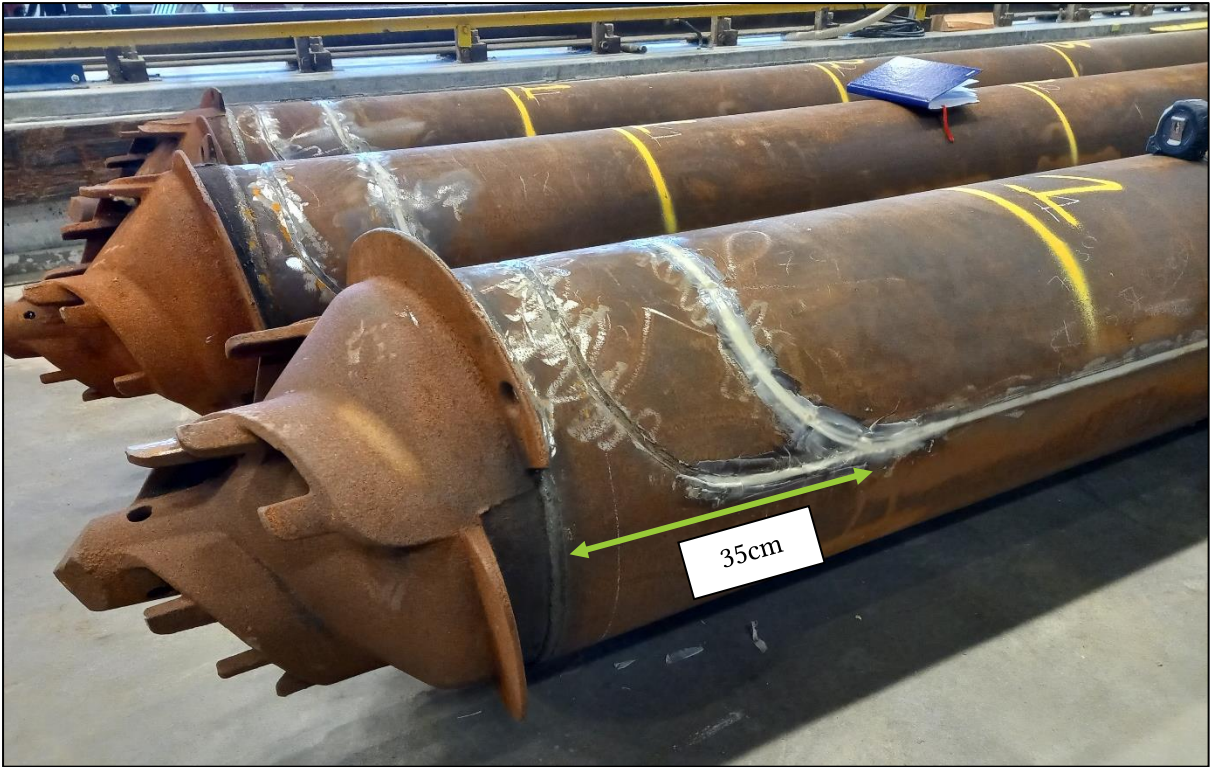
Figure 4.7: Grooves prepared at pile tips, showing the glued-in-placed FO cable transitioning from one side to another. Two grooves were created at the pile tip, although only one groove was ultimately used. The distance to the last possible FO reading is shown
