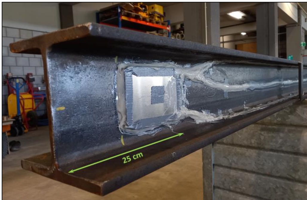
Figure 4.4: Protective cassette at the bottom of the reinforcing of the SI piles. The lowermost measurement was therefore roughly one pile diameter from the base of the reinforcing
