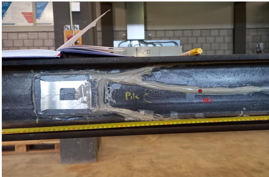
Figure E.1: Base of the H-beam reinforcing of an SI pile. Each fibre optic cable runs to the connection box where a fusion splice connects one optical fibre in the cable to the other optical fibre in the same cable. The Point (a.) is referred to as the “last gluing point” and is last reasonable axial strain measurement before the cable bends into the connection box
