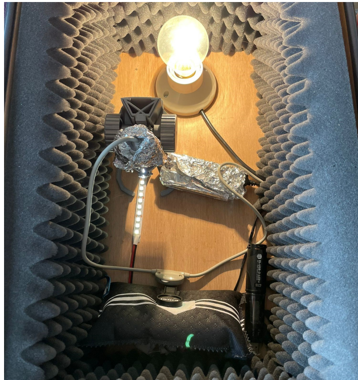
Figure B.1: Setup used for the measurements (excluding the lid and using 1 microphone). All components mentioned above are visible
