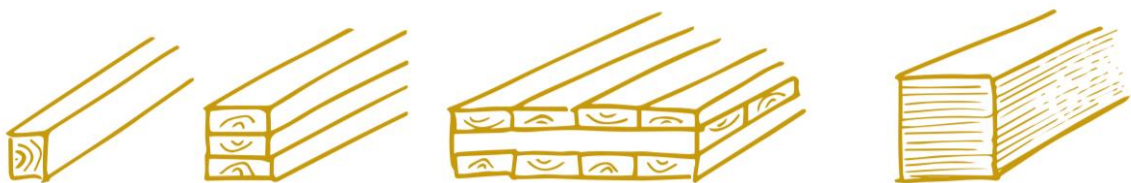
Figure 23: from left to right, solid timber, glued laminated timber, cross laminated timber, and laminated veneer lumber
