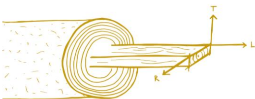
Figure 21: Longitudinal, tangential, and radial direction of timber
