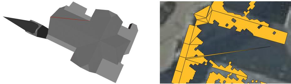
Figure 6.19: Example of a small 'closure' surface occurring in the 3D city model (left, building is located at Portlandstraat 57). The irregular shape can lead to erroneous results as the region growing method 'fills up' and labels the entire shape as 'deviation'.
