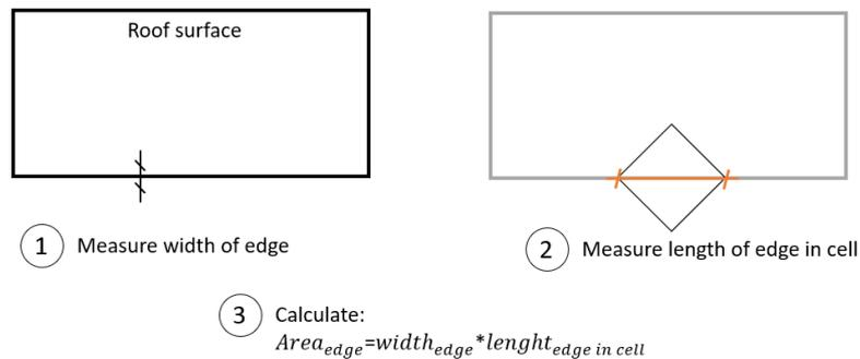
Figure 6.7: Schema showing the approach used in the case of roof edges. Beforehand, the constant width was measured so that in the subsequent steps only one dimension was left to measure.
