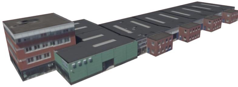
**Figure 3.10:** Sample building Albert Plesmanweg 103 used for the exploratory study, downloaded from the Rotterdam 3D city model. One can note the roofs which have been modeled as flat planes while roof windows visible in the texture are actually not flat.
