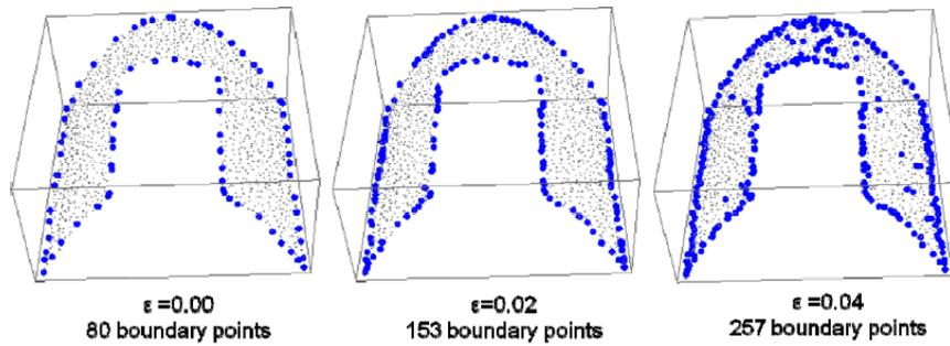
Figure 4.9: Results of the improved approach shown in figure 4.6 that are shown in Wang and Shan (2009). The improved consists of adding a threshold to avoid labeling points close to the local convex hull border as 'non-boundary' points. One can see that some critical corner points are not identified in this version either.
