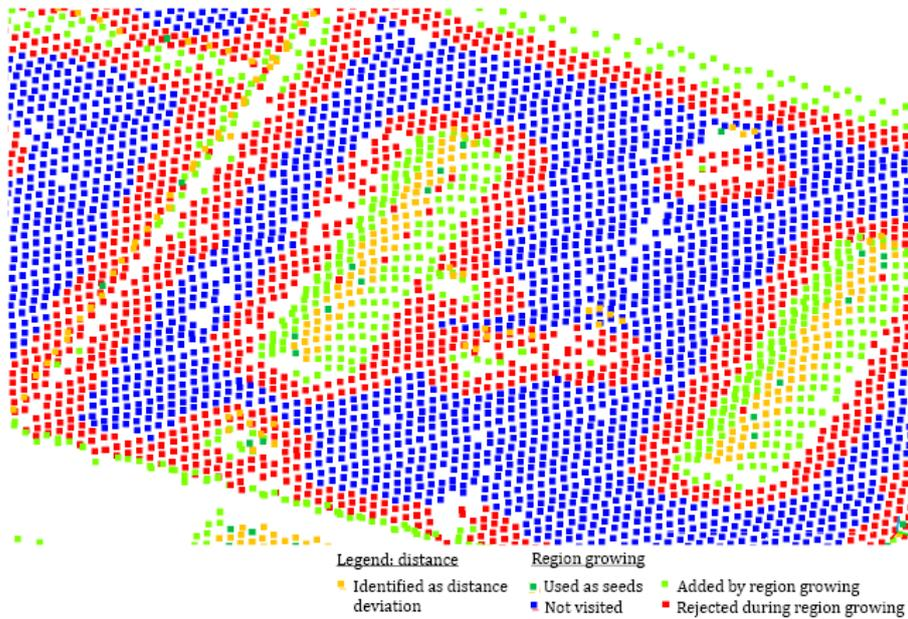
Figure 3.27: Illustration of the distance deviation identification and subsequent region growing approach(settings used: 40cm distance tolerance, 5.73 degrees angular tolerance and 10 for both KNN settings).
