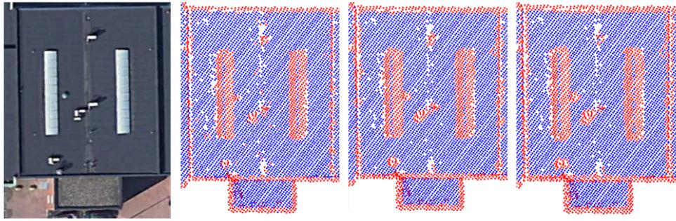
Figure 3.19: Results obtained for normal vectors obtained by using PCA on different KNN neighborhood settings. Normal vectors diverging more than 5 degrees from a vertical one are colored red, others blue. From left to right: satellite image from google earth (taken on 15/01/2019), KNN settings of 5, 10 and 15.
