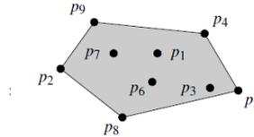
Figure 4.1: Example of a convex shape for a set  $P$  of input points (De Berg et al., 1997).
