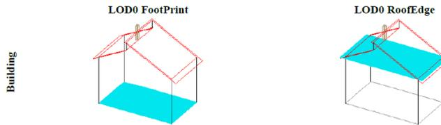
Figure 1.10: Representations of a building as a polygon in LOD0 (Gröger et al., 2012)
