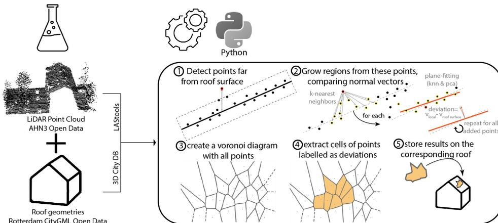
Figure 7.1: Illustration of the method developed for the identification of 'deviations' of LiDAR compared to LOD2
