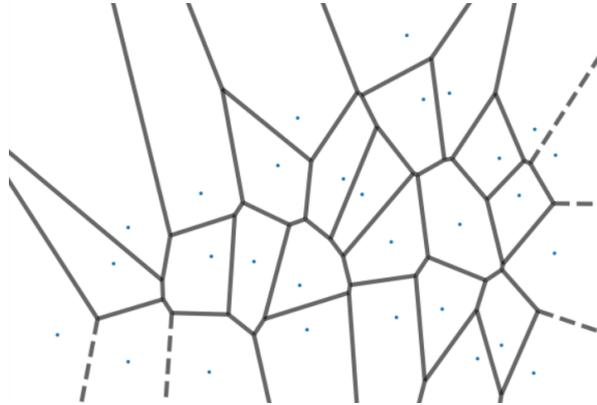
**Figure 4.4:** Example of the Voronoi diagram obtained for a set of points. Space is divided into cells. Any point lying inside a cell is closer to the respective input point of that cell than to any other input point (in blue).
