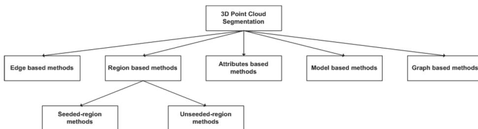
Figure 3.1: Taxonomy of 3D point cloud segmentation methods as proposed by [Nguyen and Le \(2013\)](#)
