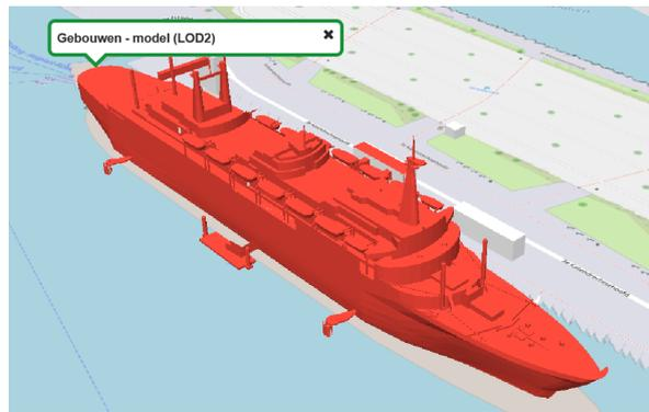
Figure 7.3: Example of a 'building' (actually a ship) that is labeled as LOD2 while it rather seems to fulfill LOD3 standards.
