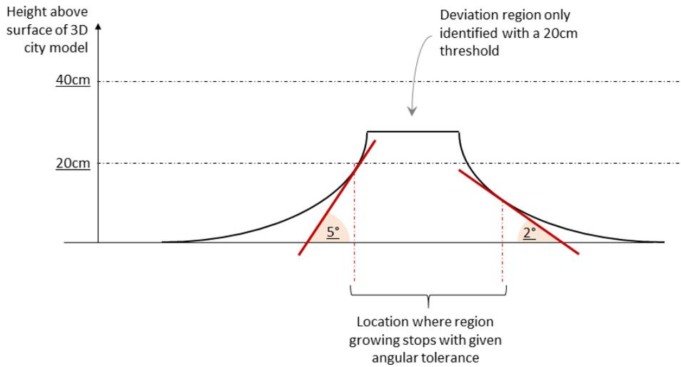
Figure 6.3: Schema explaining the impact of settings for a 'deviation' of height 25cm. This one will only be detected with a height threshold of 20cm, not 40cm. In the case presented here, the 'deviation' will 'grow' stop growing depending on the angle tolerance used (earlier for 5 degrees than 2 degrees).
