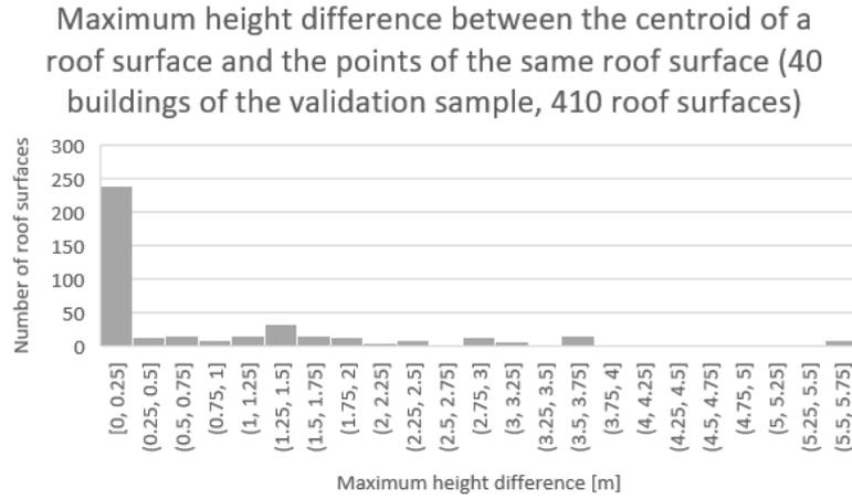
Figure 5.7: Histogram showing the distribution of the maximum difference between any point and the centroid, per roof surface.
