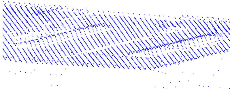
**Figure 3.11:** Close up zoom on roof windows in the [AHN](#) point cloud. Here, the height deviations of the roof windows are indeed present.
