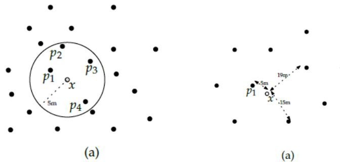
Figure 3.3: Illustration of the fixed-distance neighbors (FDN) (left) and KNN (right) approaches. While on the left all points within 5m are selected independently of their number, on the right the three closest points are selected independently of their distance (source: course material GEO1015).
