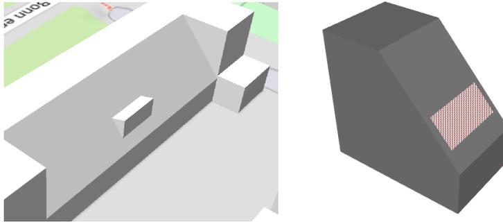
Figure 3.9: Example of an object of class *OuterBuildingInstallation* in the Rotterdam 3D city model: the dormer (left image). On the right, one can see that this results in a hole (inner border) in the roof geometry.
