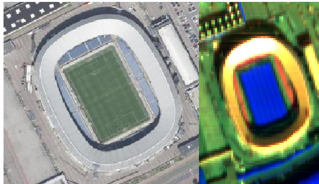
Figure 5.5: Illustration of the need for orthorectification. On the left: nearly orthorectified aerial image of the Feyenoord stadium (source: PDOK aerial imagery 2016). On the right: false color acapex imagery of the same stadium with the effect of projection (Red = 399-413 nm, Green = 1145-1155nm, Blue=2423-2432nm).
