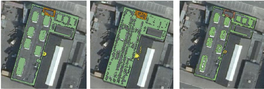
Figure 6.4: Example of the result obtained by applying the method to a roof with windows which are missing in the 3d model. Settings used here are 20cm (all three images) for the distance threshold and 2.56 (left), 1.13 (middle) and 5.73 (right) degrees for the angle threshold. Background imagery: (c) pdok
