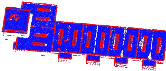
Figure 3.18: Normal vectors obtained by applying principal components analysis on  $KNN=10$  neighborhood. The normal vectors that diverge more than 8 degrees from a vertical one are colored in red, the other ones in blue. Note the blue points at the very inside of the roof windows.
