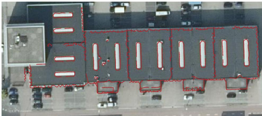
Figure 4.11: Example result obtained by implementing the pseudo-code presented in figure 4.10 to the result of which an extract was presented in 4.7. To allow easier implementation, the line segments were not closed in the cases where a circular line segment should be generated. In some cases, the minimum spanning tree is quite literally a tree: it is not composed of a single line segment but of several connected ones.
