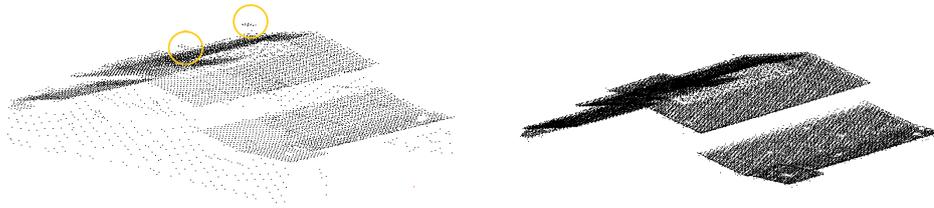
Figure 3.7: Samples of the two available point clouds. On the left AHN, the chimneys on the roof can clearly be seen. In contrast, the points of the chimney are completely missing in the example on the right (City of Rotterdam point cloud).
