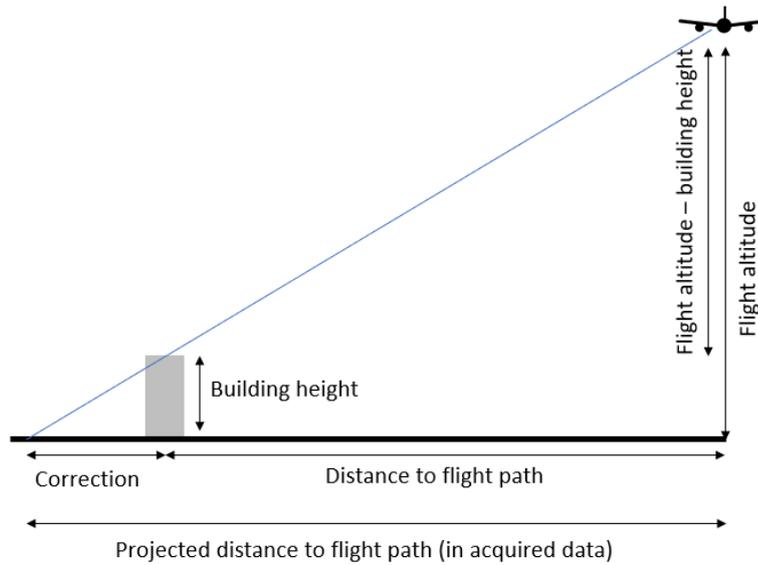
Figure 5.6: Trigonometric approach to the correction of perspective distortion in aerial images (production of orthophotos).
