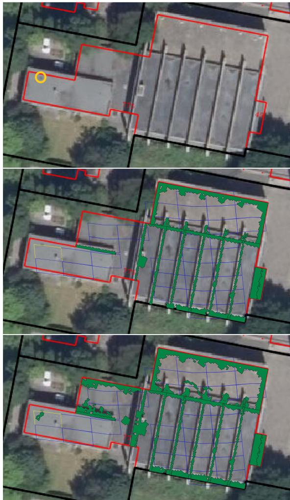
**Figure 6.6:** Example of a 'deviation' (identified in ground 'truth', left picture), that is not identified using the 40cm, 5 degrees setting (middle), leading to a commission error for the class 'clean' - in opposition to the 20cm, 2 degrees setting (bottom) where the cell is correctly classified as 'non-clean'. One might further note that in the same cell but at the bottom right, there is a 'deviation' which was identified by neither of the two methods. Background imagery: (c) PDOK, 2016
