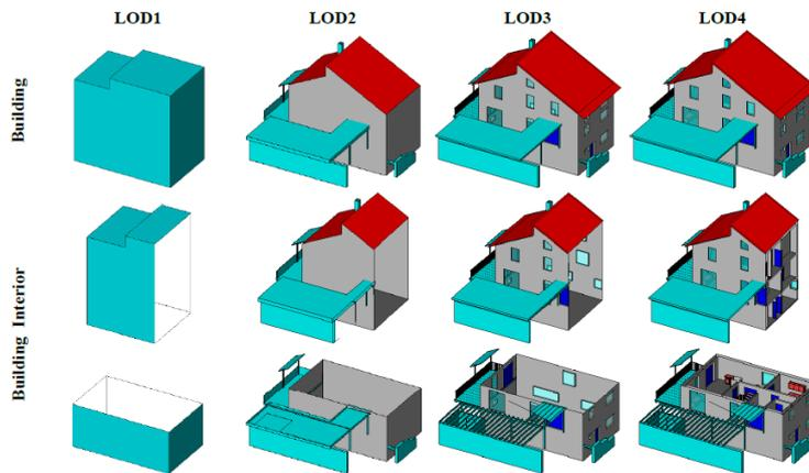
Figure 1.11: Building representation in LOD1-4 (Gröger et al., 2012)
