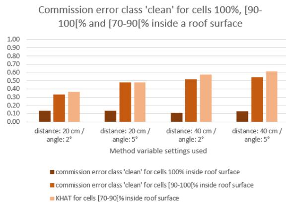
**Figure 6.14:** Commission error for the class 'clean' evolution for cells 100%, [90-100%] and [70-90%] inside a roof surface. With all settings, an increasing trend can be observed. The increase is however less pronounced for the 20cm and 2 degrees setting.
