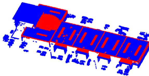
Figure 3.14: Same calculation as in the previous figure, but with the higher density point cloud (red: distance exceeding 20cm, others blue). Just as in the previous example, one can note a cluster of deviations on the left side. These are probably due to a roof slope that is absent in the 3D city model.
