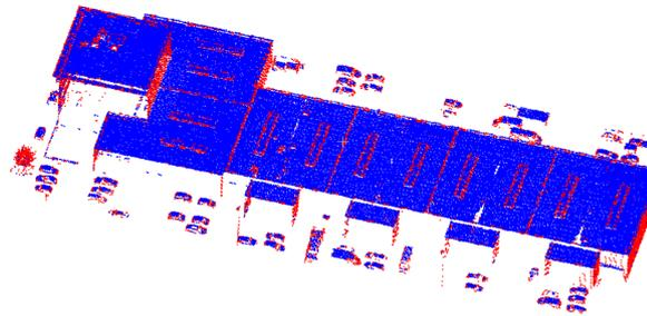
Figure 3.16: Results of the height difference within neighborhood ( $KNN=3$ ) computation but using a higher definition point cloud. One can note influence of the point density.
