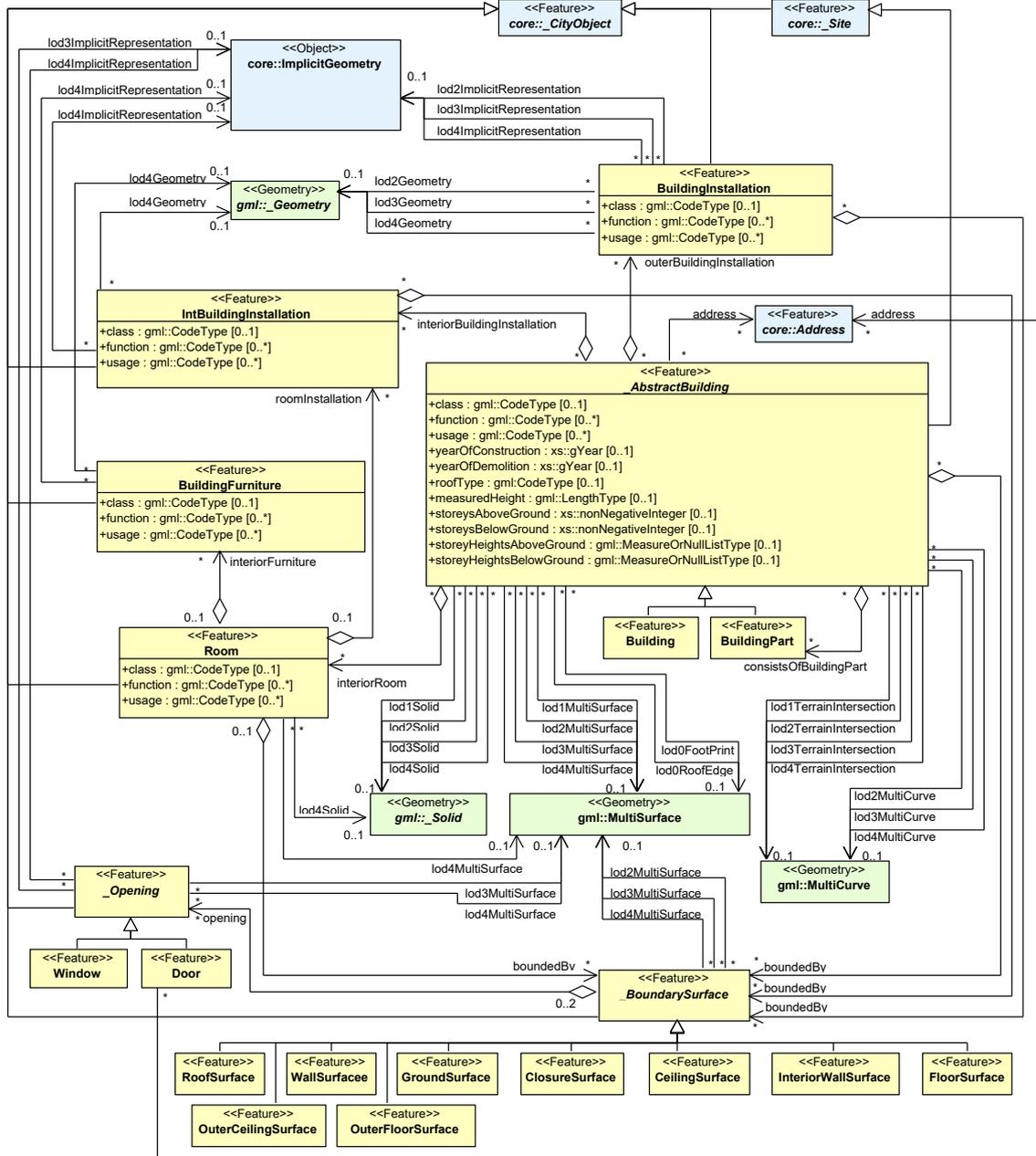
Figure 8.1: UML diagram of the CityGML building class (Gröger et al., 2012).
