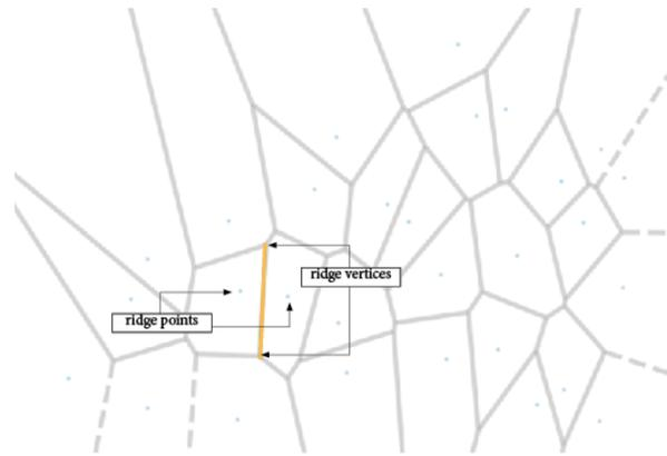
Figure 4.15: Illustration of the meaning of the terms 'ridge points' and 'ridge vertices' (as used in *scipy.spatial.Voronoi*), for a given Voronoi diagram edge.
