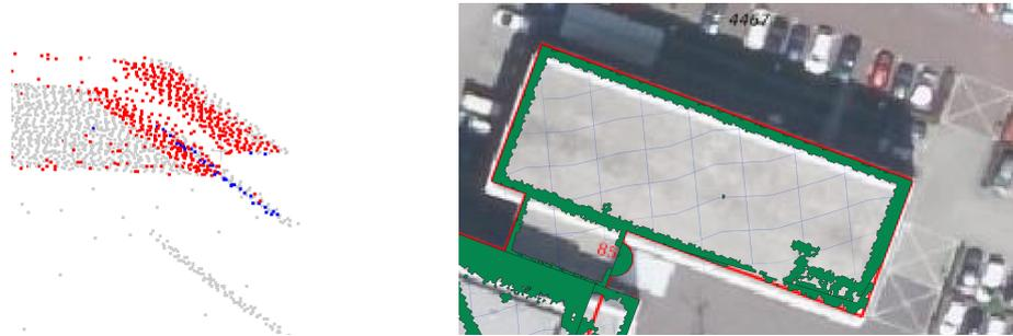
Figure 6.20: Example (Waalhaven O.z. 85) of a building where the method (visualizations with setting 20cm and 5 degrees) leads to an overestimation of the roof edges. As can be seen on the left, the region growing algorithm grows beyond the actual edge object (points in blue are the seeds, points added by region growing are colored in red). The result can be seen on the right. While the edge on the aerial image is estimated at 80cm, the method identifies an edge of about 140cm.
