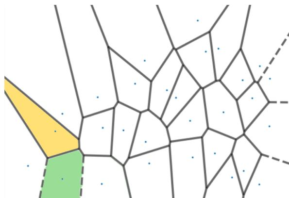
Figure 4.12: Example of the Voronoi diagram obtained for a set of points. One can observe that i) cells of points belonging to the vertices of the convex hull are non-closed and (e.g. green cell) ii) that some closed cells have a vertex located outside the convex hull (e.g. yellow cell).
