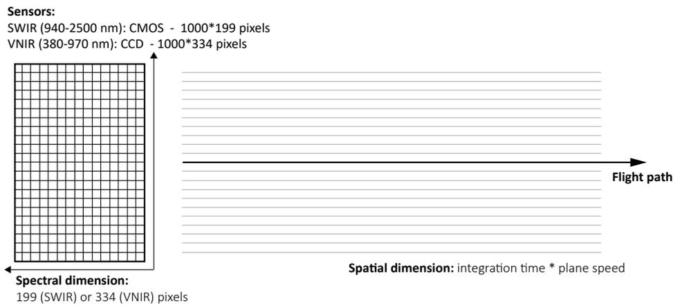
Figure 5.3: Illustration of the different dimensionality involved during data acquisition with the APEX device.
