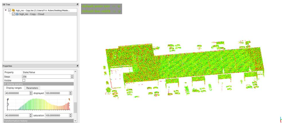
Figure 3.22: Curvature values obtained by applying principal components analysis on  $KNN=5$  neighborhood on the higher density point cloud. Note the red points at the very inside of the roof windows. Note: values on the left are curvature  $\times 100$
