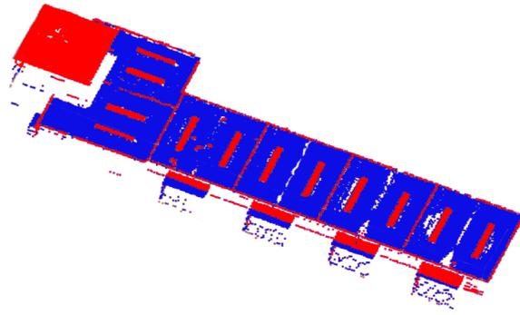
Figure 3.12: Distance of the points with regard to the roof surface of the 3D city model. Points with a distance exceeding 30cm are colored red, others blue. One can see that roof windows are partially identified; points close to the crease edge, to the junction with the roof are missing.
