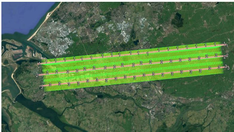
Figure 5.1: Overview of the flight lines of the hyperspectral acquisition performed by the [APEX](#) on 17 September 2014 in Rotterdam. Background imagery: (c) google earth
