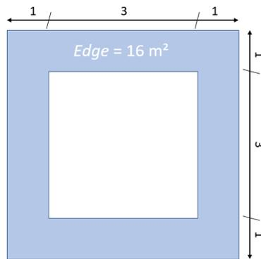
Figure 7.2: Schema showing the ambiguity of modeling roof edges with regard to the CityGML LOD standards. The edge here has a total attached area of  $16 m^2$  and should thus be modeled. But if it split in two parts, the attached area would be too low to be modeled while the edge might be nearly as relevant.
