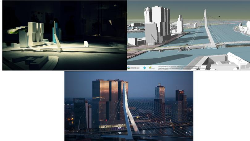
**Figure 1.9:** Both physical urban scale (top left) and a digital city model (top right) are abstractions of the reality (bottom). The main difference lies in the storage of ‘meaning’, i.e. of semantics.<sup>2</sup>
