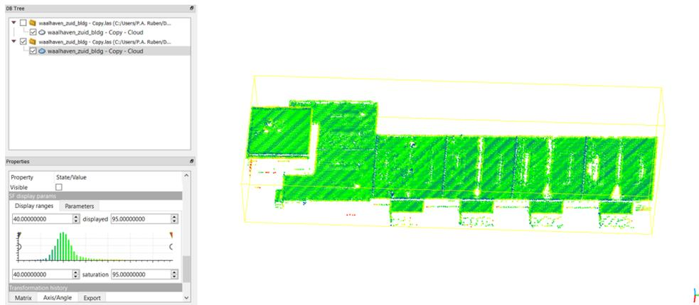
Figure 3.21: Curvature values obtained by applying principal components analysis on a  $KNN=20$  neighborhood. Note the red points at the very inside of the roof windows. Note: values on the left are curvature  $\times 100$
