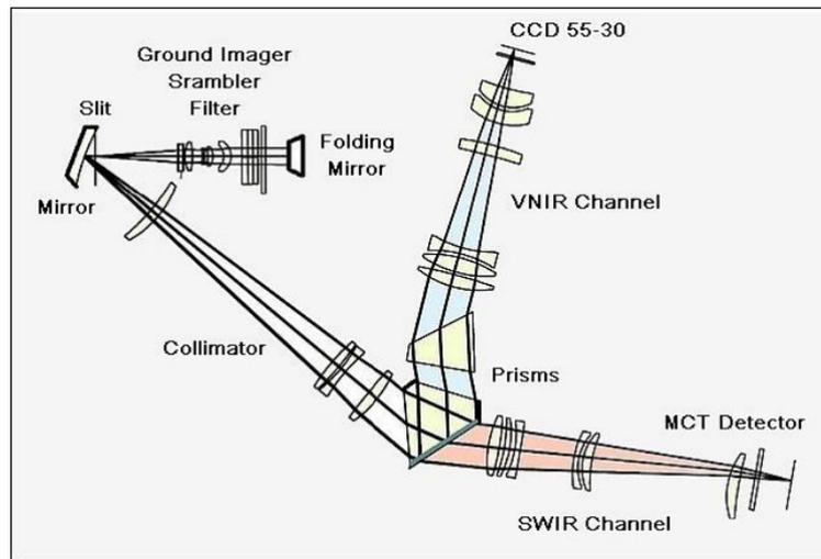
Figure 5.2: Optical design used in the apex spectrometer (ESA Earth Observation Portal Directory, n.d.).
