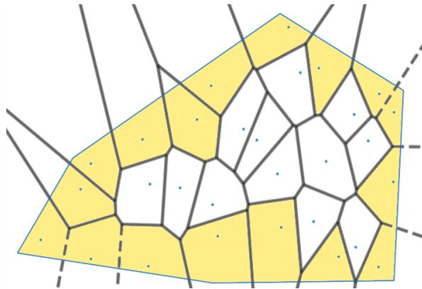
Figure 4.14: Illustration of the usage of a bounding box to limit the extent of non-closed and outlying cells. The roof surface geometry is shown as a blue line and the affected cells are colored in yellow.
