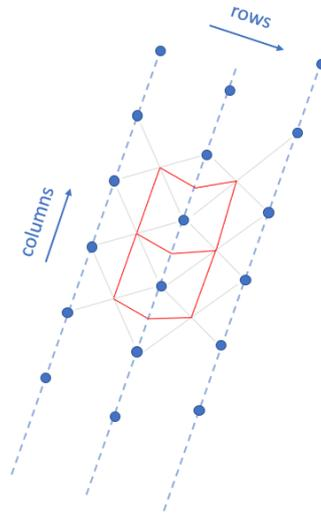
Figure 5.4: Approach allowing to generate a mesh using the orthorectified centerpoints of the 8 neighbouring pixels.
