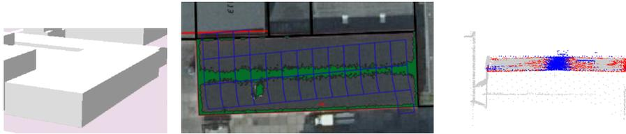
Figure 6.17: Example of a building (Van Meelstraat 44) that has erroneously been modelled with a fully flat roof in the 3D city model of Rotterdam (image on the left). 'Deviations' identified in the middle of the roof (blue in the point cloud in the middle, green on the aerial image on the right), do not represent a material 'deviation' but simply the peak of the slightly gabled roof surface (visualisation in the middle and right obtained for 20cm and 5 degrees settings).
