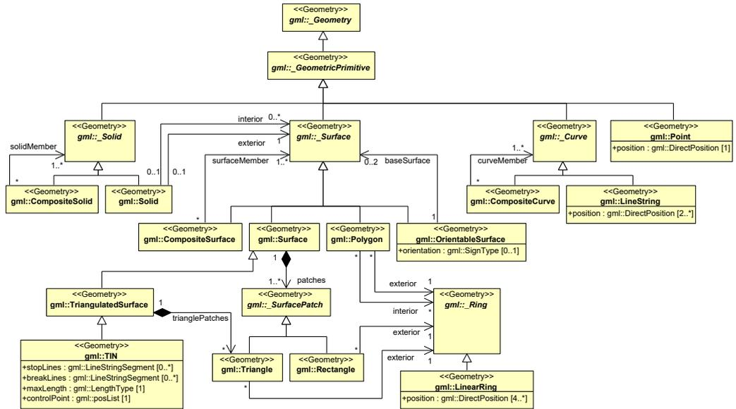
Figure 8.2: UML diagram of the CityGML geometry model (Gröger et al., 2012).
