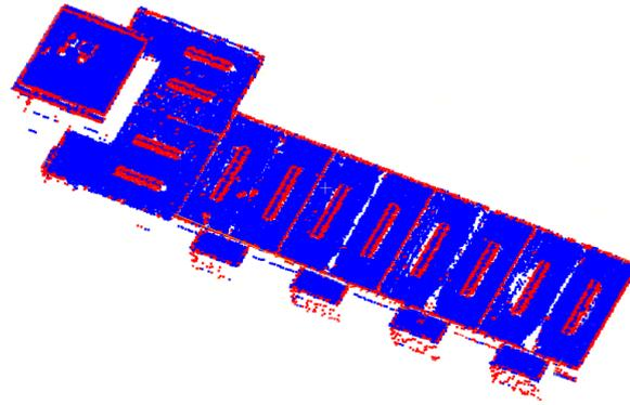
Figure 3.15: Result of the height difference within the neighborhood ( $KNN=3$ ) of each point. A threshold of 5cm was applied: points above it are colored red, others blue.
