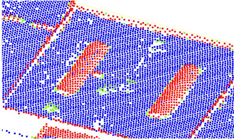
Figure 4.7: Example result obtained by implementing the pseudo-code presented in figure 4.6 (10-nearest neighbor setting). The points that were labeled as 'deviations' are in green if they were labeled as border points too and in red otherwise. The points in blue are the ones of the initial set that were not labeled as 'deviations'.
