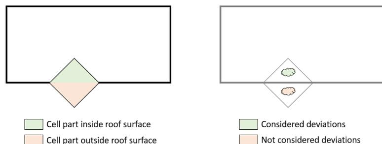
Figure 6.12: Schema showing the case of cells that are not entirely inside a roof cell. In that case, only the 'deviations' in the part inside the roof cell are taken into account.
