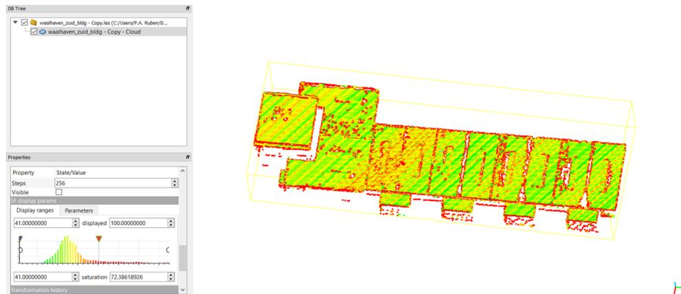
Figure 3.20: Curvature values as computed for each point with a KNN=5 setting. One can see curvature values change along some of the roof window crease edges. Other changes with smaller but still considerable magnitudes seem to be related to the scan lines and noise. Note: values on the left are curvature  $\times 100$
