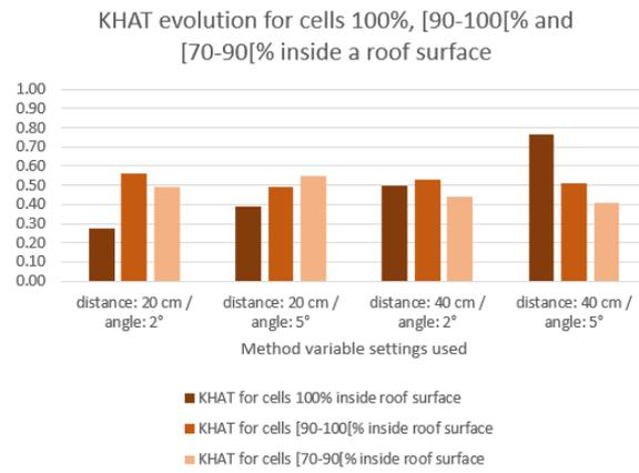
**Figure 6.13:** KHAT evolution for cells 100%, [90-100%] and [70-90%] inside a roof surface. For all cases with a setting of 20cm, the khat tends to increase when loosening the cell in roof surface criterion. For the 40cm, 2 degrees settings, the trend is rather stable. In contrast, the 40cm, 5 degrees settings result in a decreasing trend.
