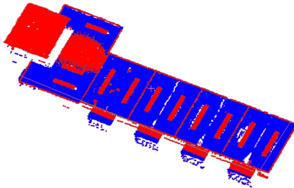
Figure 3.13: Distance of the points with regard to the roof surface of the 3D city model. Points with a distance exceeding 20cm are colored red, others blue. Note the red cluster on the left.
