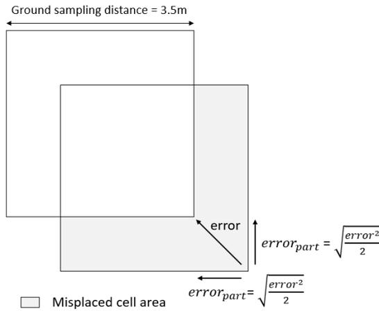
Figure 5.8: Illustration of the maximum impact of a potential inaccuracy on a cell of 3.5\*3.5m.
