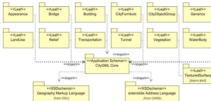
Figure 3.4: UML diagram illustrating the different modules of CityGML (Gröger et al., 2012). This thesis will only cover the 'Building' module
