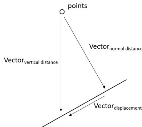
Figure 3.26: Illustration of the trigonometric equation to calculate the vertical distance.
