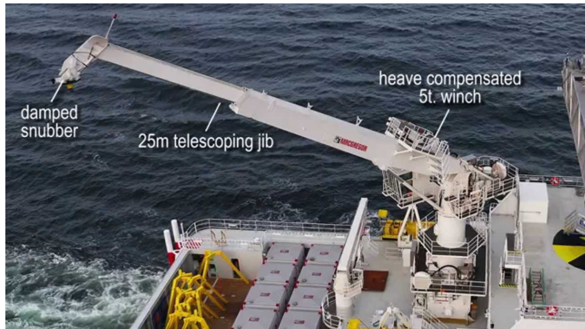
Figure 2.18: Motion compensated offshore crane, [www.youtube.com/Cargotec, 2018]
