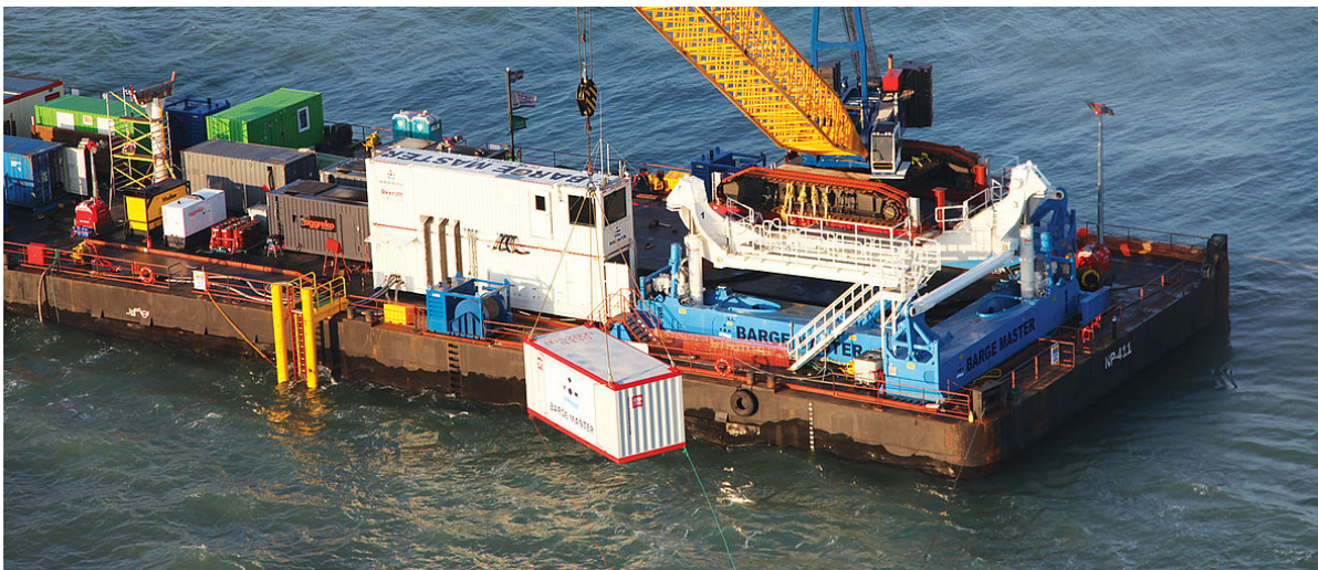
Figure 2.17: Heavy payload vessel motion compensated platform, [www.barge-master.com, 2018]
