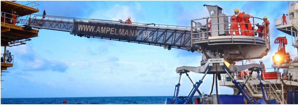
Figure 2.16: People transfer with an Ampelmann platform, [www.ampelmann.nl, 2018]
