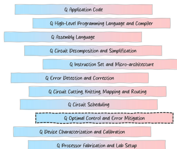
Figure 1. Overview of the system design of a quantum accelerator with classical control and various software modules required for research and development is shown on the left. The different abstraction layers for full-stack quantum computing are shown on the right. This research pertains to the optimal control layer highlighted with a dotted outline.
