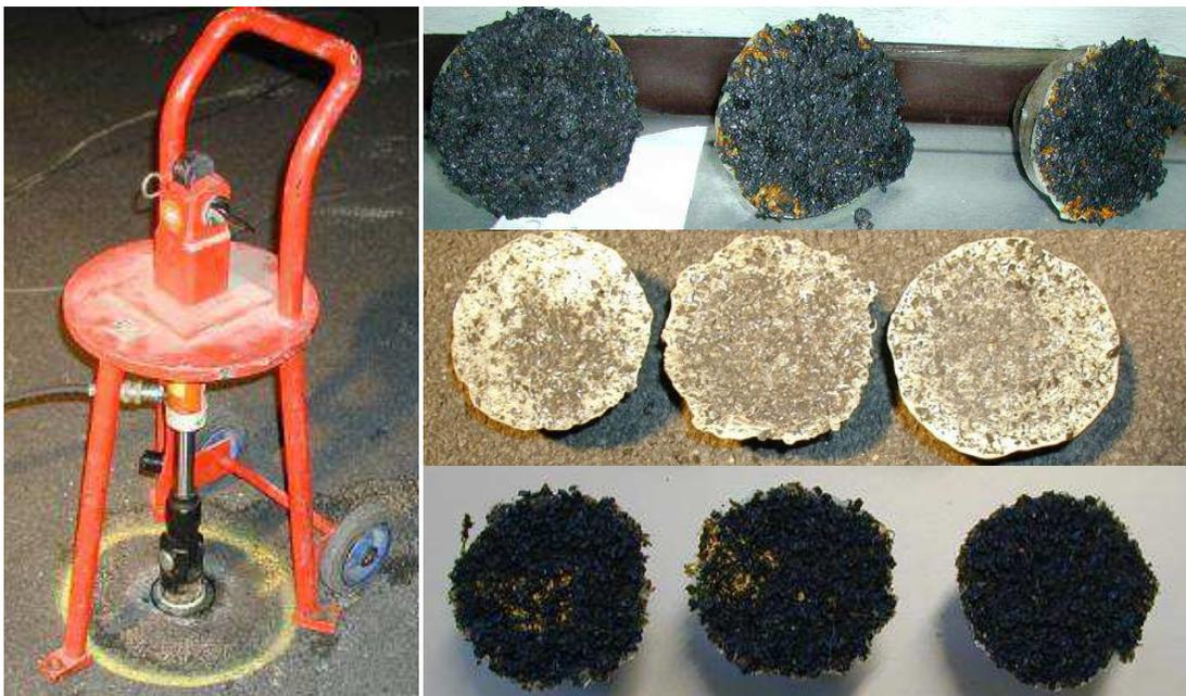
Figure 2-7 Setup for bonding tests (left) and examples of tested surface coatings
