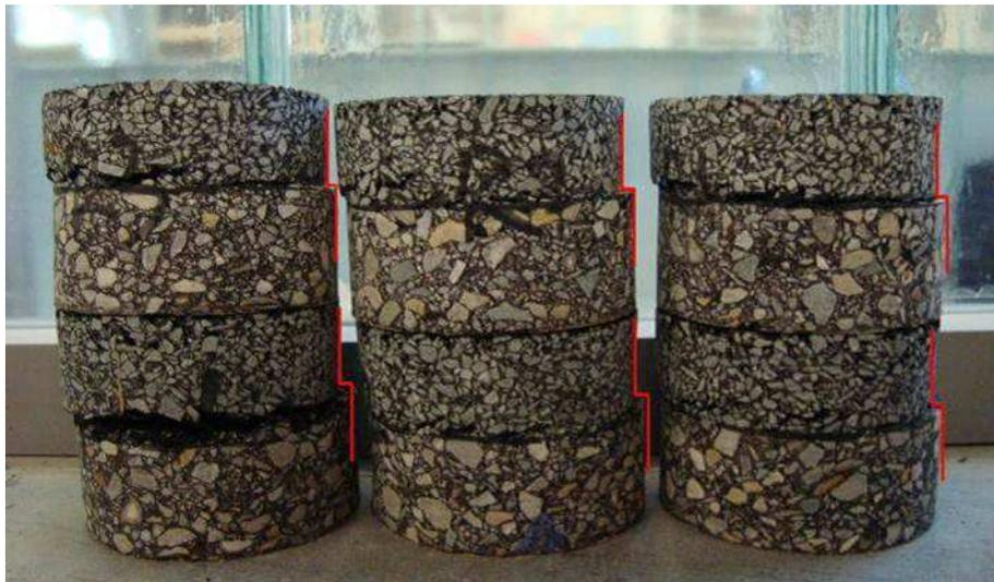
Figure 6-15 NRTSL specimens after Leutner shear test
