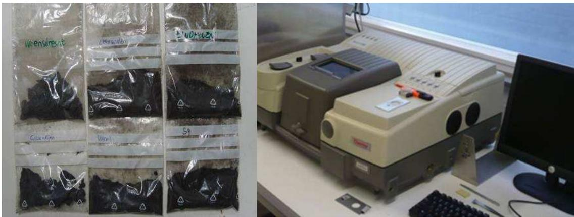
Figure 4-19 Powder of tar-containing antiskid mixtures and FTIR tester
