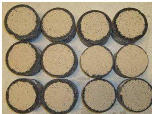
Figure 4-16 Sand patch test on tar-containing antiskid layers
