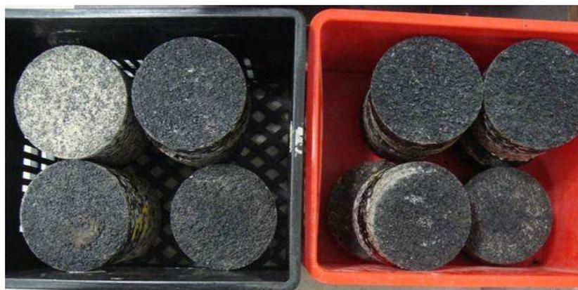
Figure 3-9 Schiphol cores with new Possehl antiskid layer
