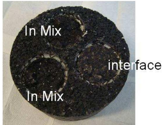
Figure 6-8 Failure in the asphalt mixture and at the interface
