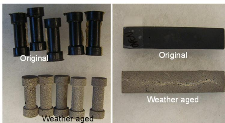
Figure 5-38 Specimens of the original and weatherometer aged specimens
