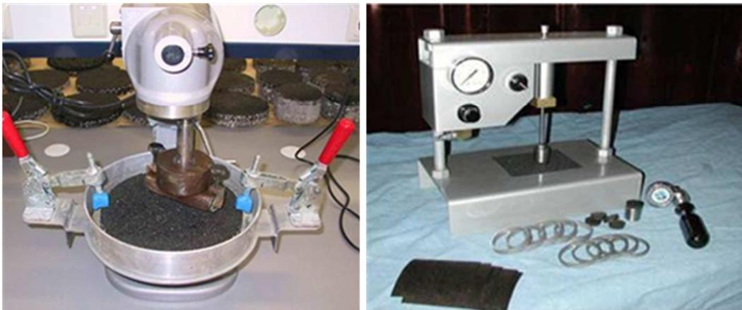
Figure 2-18 WTAT setup (left) and Cohesion test setup (right)
