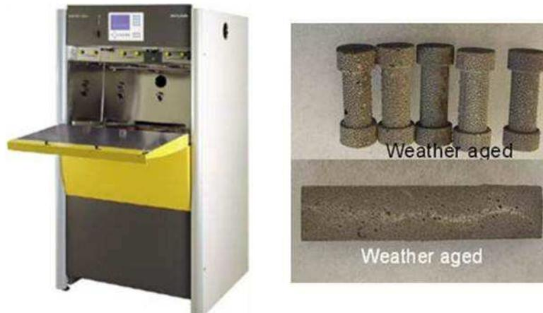
Figure 3-14 Weatherometer and DSR/DMA samples
