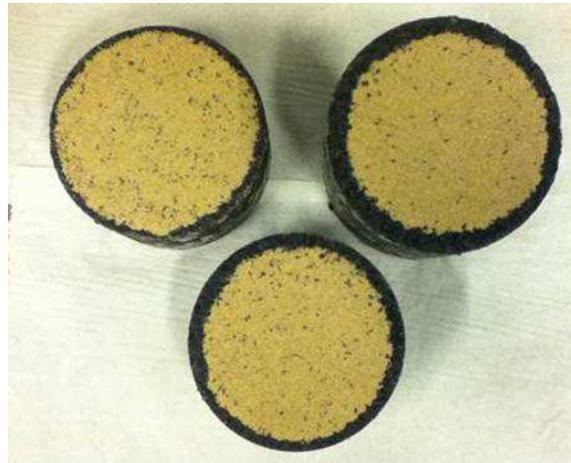
Figure 6-7 Spreading of the sand on the 150 mm diameter cores
