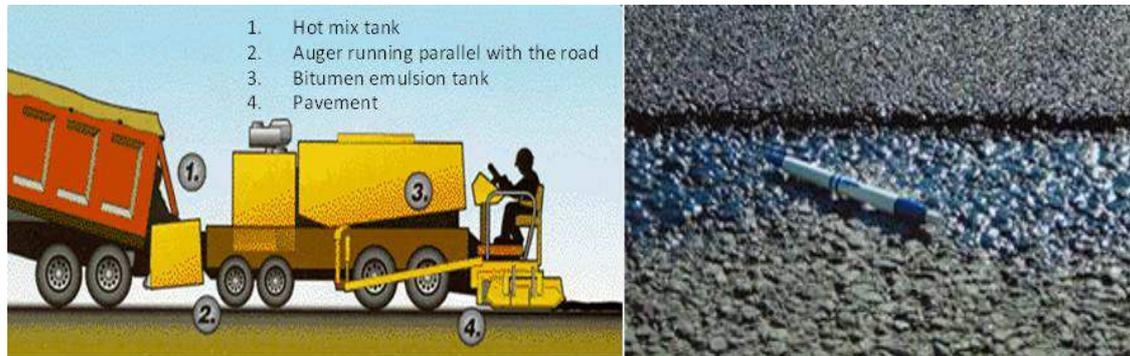
Figure 2-5 Specifically designed paving equipment and thickness of Novachip
