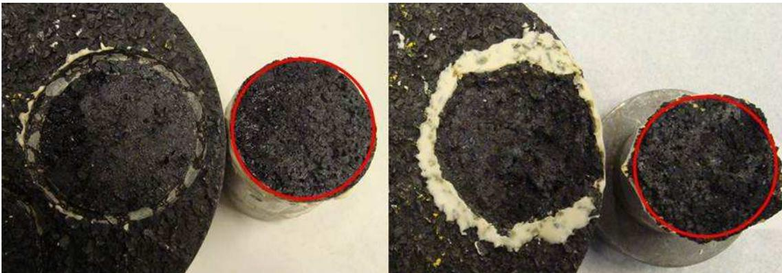
Figure 3-32 Failure surfaces at the interface
