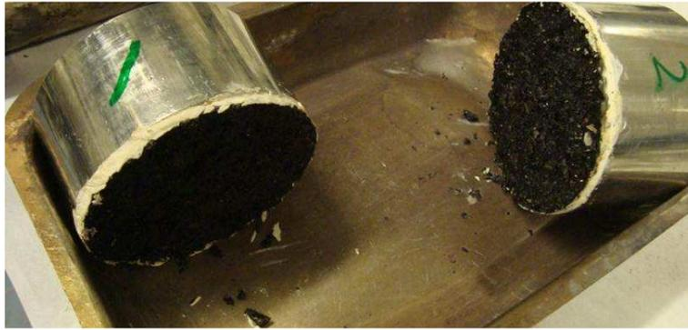
Figure 4-5 Deformations after one hour in the oven at 150 °C of type 1 specimen
