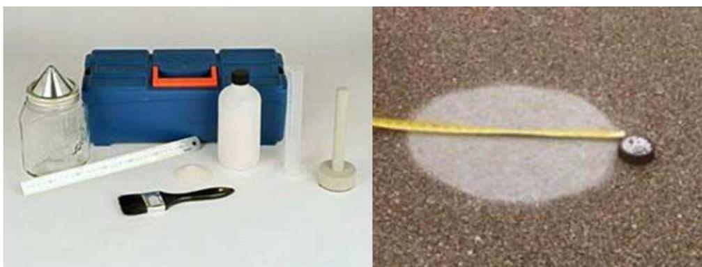
Figure 3-38 Sand patch test in the field<sup>6</sup>
