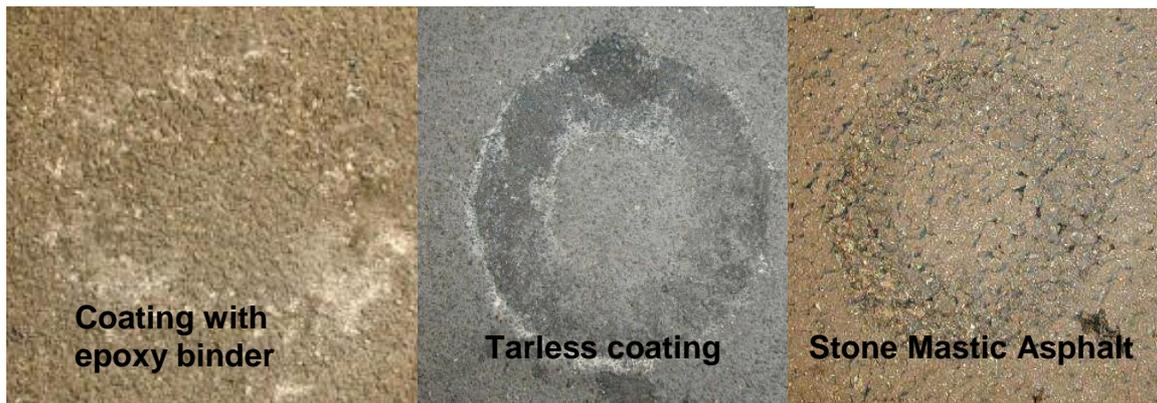
Figure 2-9 Results of raveling test on three different coatings
