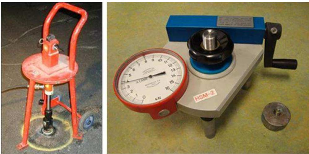
Figure 3-26 Simple pull test setups
