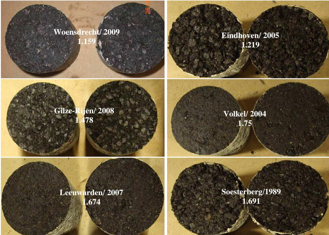
Figure 4-29 Interface failure surfaces after the Leutner shear test
