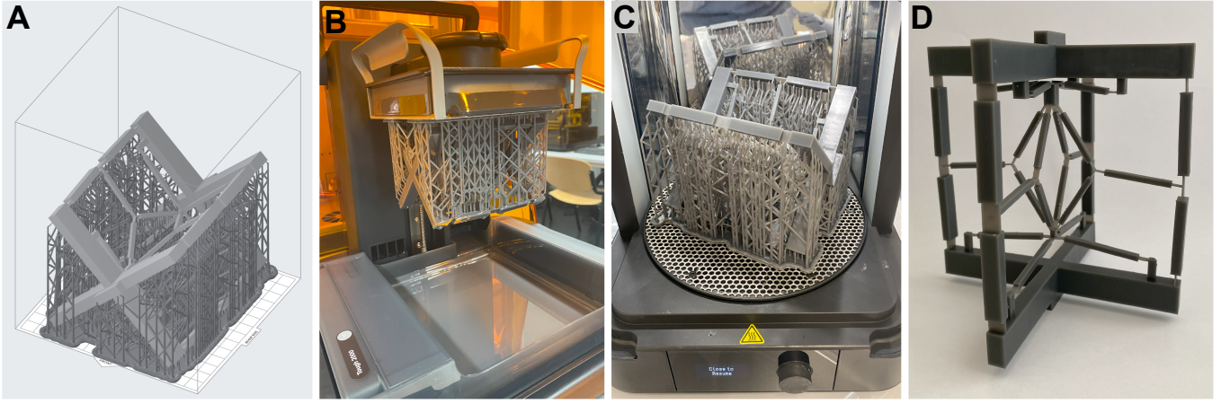
Fig. 6. Fabrication process of the unit cell prototype. A Screenshot of the 3D model in the slicer software 'PreForm', where the print settings and support structure are defined. B Photo of the just finished print inside the Formlabs Form 3 printer. C The printed structure inside the 'Form Cure' curing machine, where it is cured for 60 minutes at 70 degrees Celsius after it has been washed in IPA twice for 10 minutes. D The final unit cell prototype, after the support structure has been removed.
