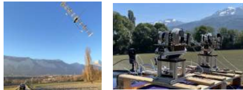
Fixed-distance flight test with Wind Fisher's developmental prototype towed by a vehicle (left). Prototype ground-station (right).
