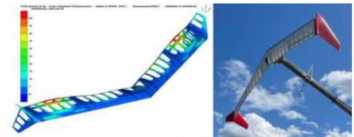
Modalanalysis (FEM) of the EnerWing-Gridshell. EnerWing-Gridshell docked on the mast of EK30
