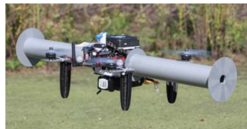
Magnus effect-based quadcopter system
