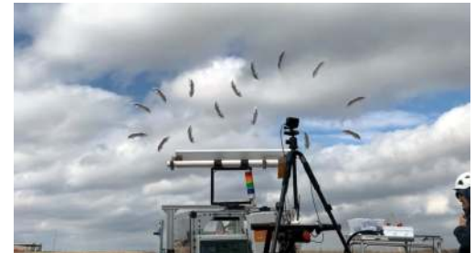
Images superimposed to depict the figure-of-eight flight path of the AWE kite during Phase 2 test (March 2023).
