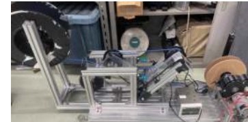
Top: Schematic diagram of winch separate-type tension power generation device, Bottom: Photo of experimental device
