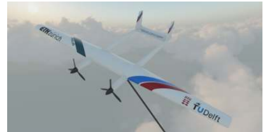
Rendering of the airborne component of the MegAWES large-scale AWE system [2].
