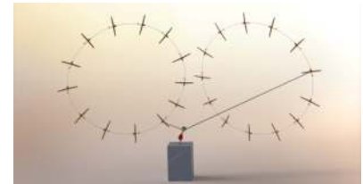
Figure 1: Stable flight path of a twin-kite system that uses only passive control mechanisms.
