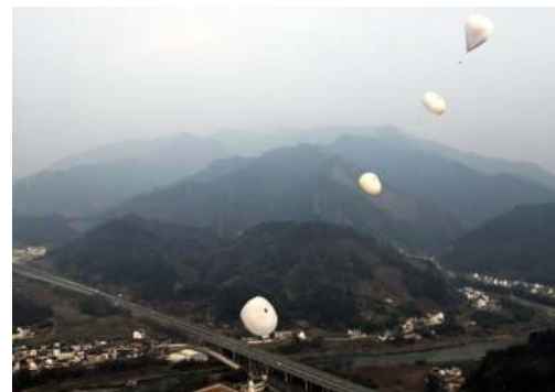
A parachute-based airborne wind energy system test.
