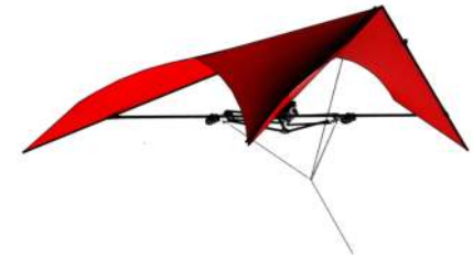
Bridle control system integrated in a delta kite.
