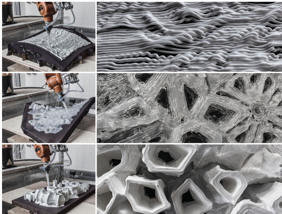
Figure 12. Robotic silicone printing experiments, linear continuous printing (top); cellular printing on a free form fabric (middle); prototype testing height, cantilevering and size ranges (bottom).
