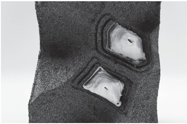
Figure 13. A test sample as a proof of concept prototype integrating subtractive robotic manufacturing applied on EPS and additive deposition of silicone with robotic arm.
