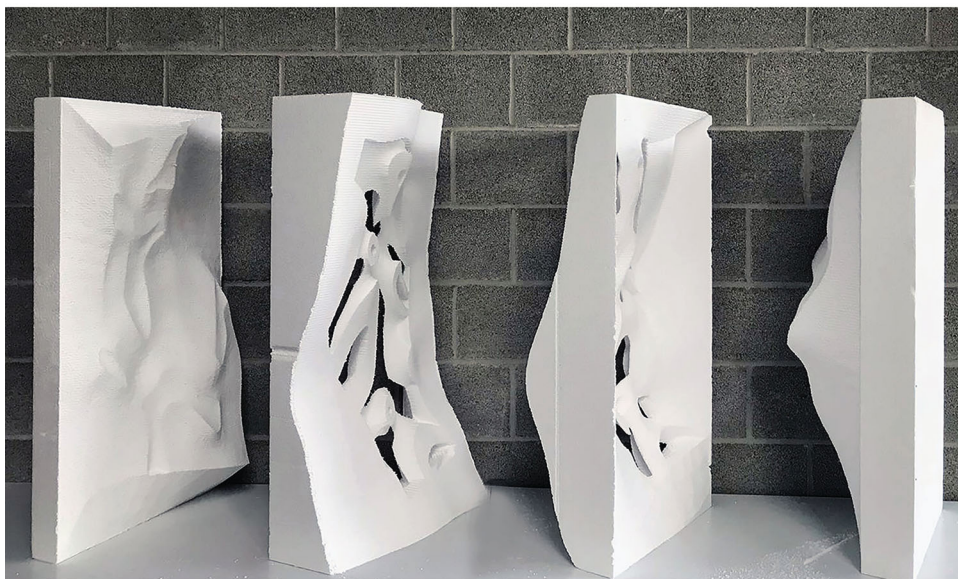
Figure 7. Mould of hybrid concrete prototype with four robotically produced parts.
