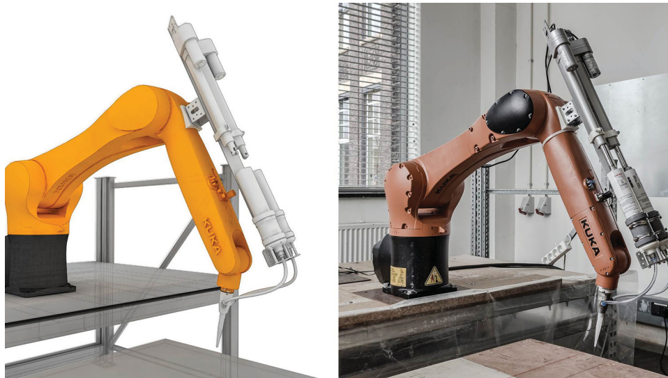
Figure 11. Parametric simulation with in KUKA|prc with integrated digital model of the extruder (left); robotic additive manufacturing setup for silicone printing with KR10-1100 (right).
