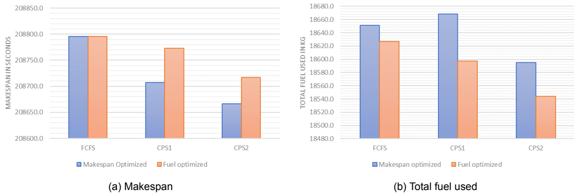
Figure 7.6: Effect on makespan and fuel by allowing a maximum position shift of 1 or 2 positions in the sequence. (a) Optimised for makespan, (b) optimised for fuel.
