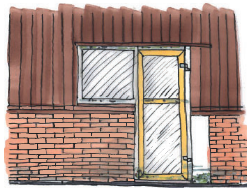
New finish of the North facade with steel plating and plastic windows/doors
