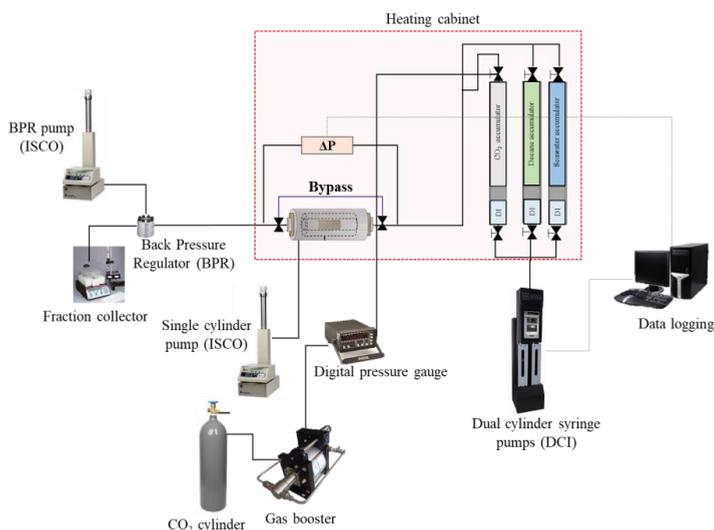
**Figure 4.1.** Schematic of the flooding unit.
