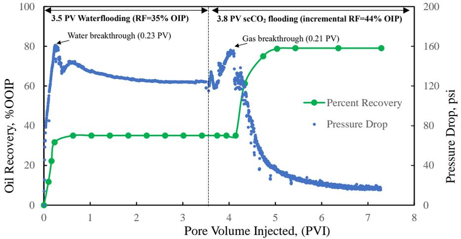
**Figure 4.2.** Oil recovery and pressure drop profile of secondary water flooding followed by miscible tertiary CO<sub>2</sub> injection conducted on composite #1.
