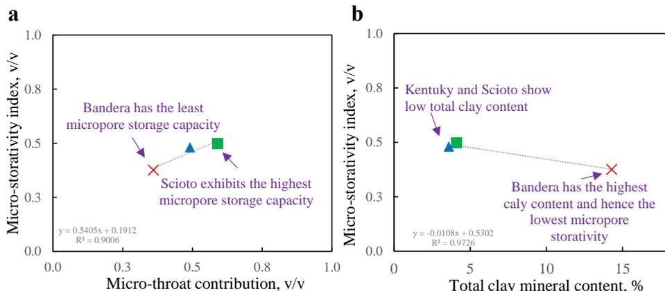
**Figure 3.5.** Cross-plots showing the relationship of micro-storativity index with: (a) micro-throat proportion; (b) total mineral content. (Note the trendlines show the relation between measurements).
