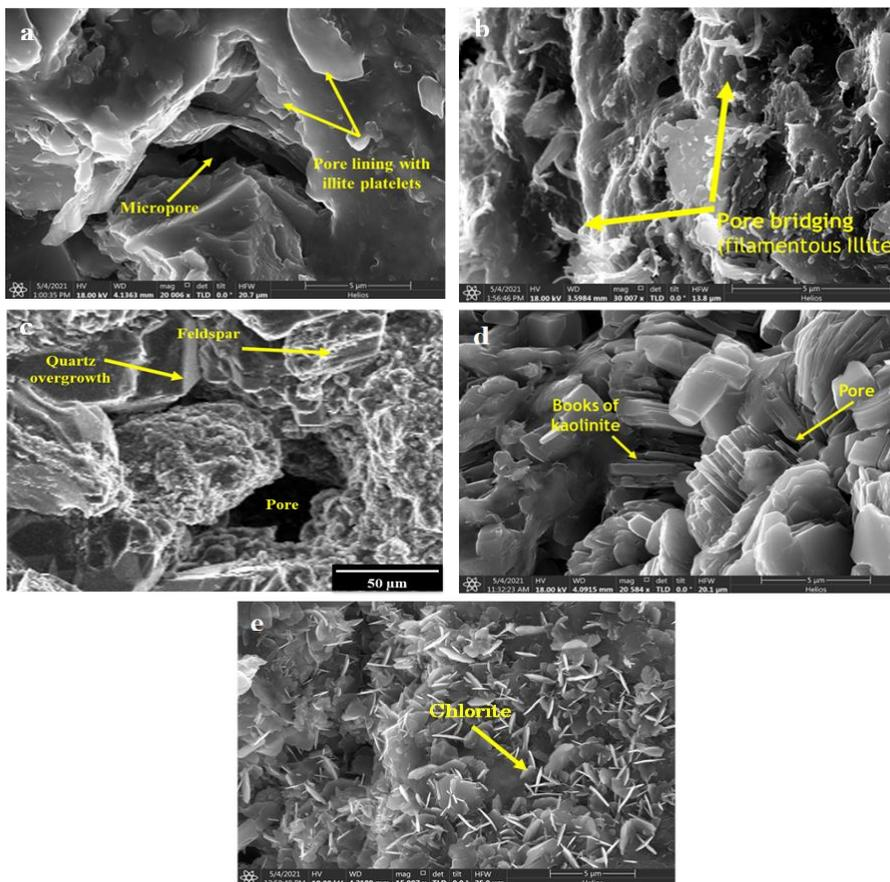
**Figure 2.4.** SEM images representing: (a) Scioto showing pore-lining with illite platelets and visible micro-pores, (b) Kentucky showing pore bridging with filamentous illite, (c) Bandera showing sharp surface as a result of the quartz overgrowths and visible pores between elongated grains, and top partly weathered feldspar with clays, (d) Kentucky showing books of kaolinite occluding pores, and (e) Bandera showing circular chlorite filling micropores.
