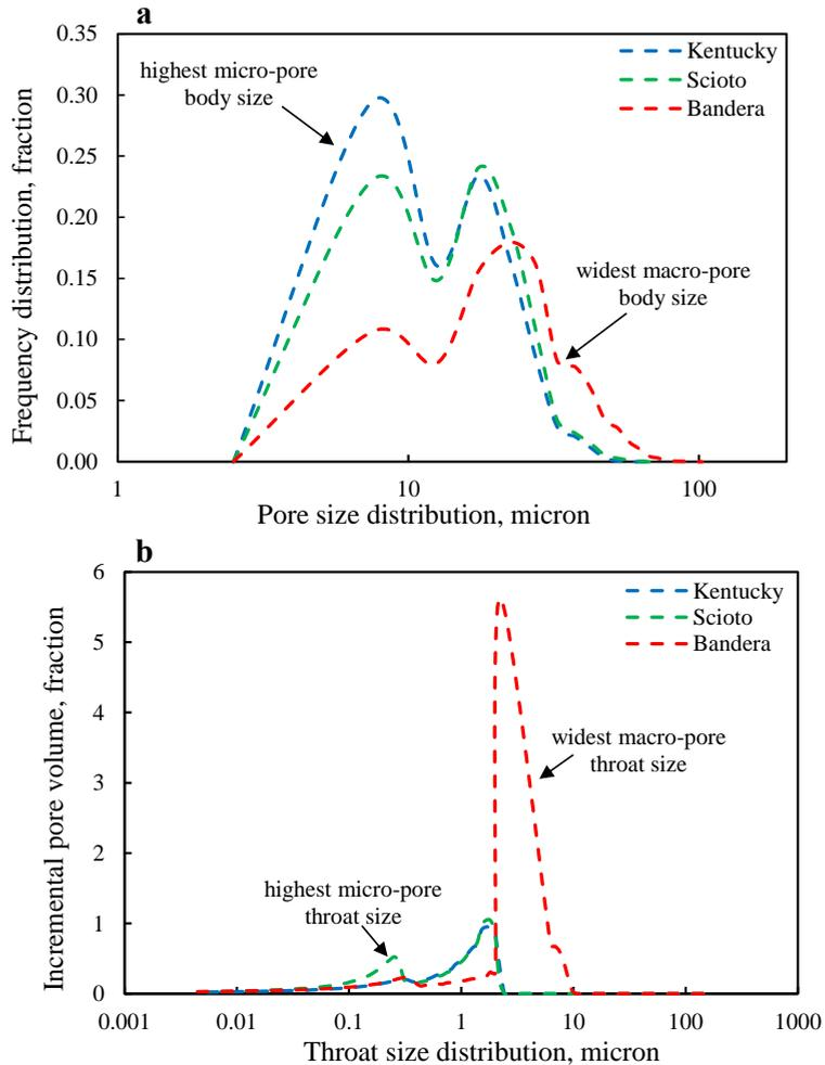
**Figure 2.7.** Pore and throat size and distributions of Bandera, Kentucky, and Scioto sandstones, where (a) shows pore-body diameter distributions obtained by Micro-CT scan and (b) represents pore-throat diameter distributions obtained with MICP.
