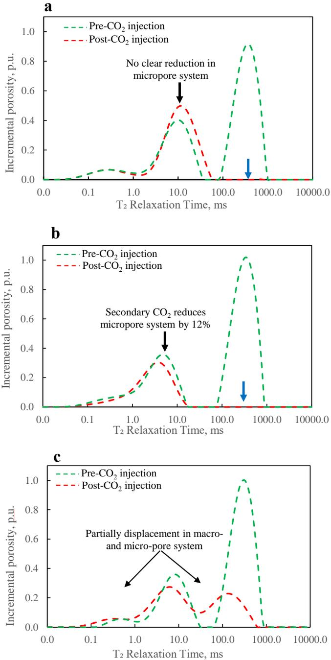
**Figure 4.7.** Incremental NMR T<sub>2</sub> of desaturated (green dashed line) and post CO<sub>2</sub> injection (red dashed line) for composite cores: (a) Tertiary miscible CO<sub>2</sub>; (b) Secondary miscible CO<sub>2</sub> injection and (c) Secondary immiscible CO<sub>2</sub> injection.
