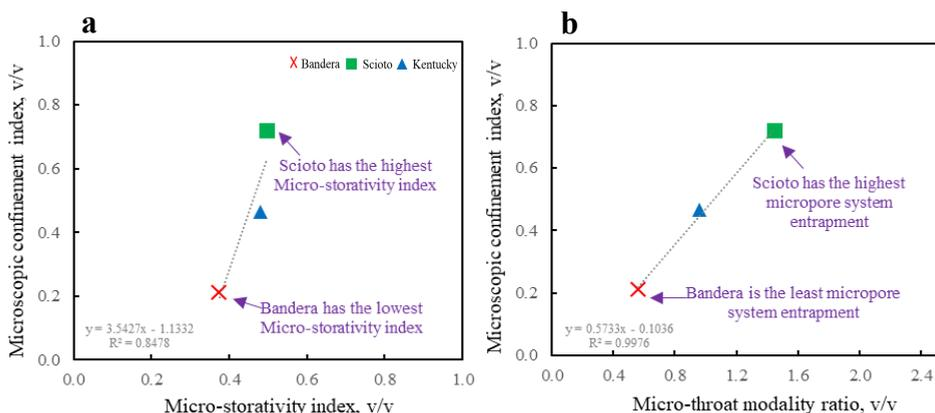
**Figure 3.4.** Cross-plots showing the relationship of microscopic confinement index of tested sandstones with: (a) micro-storativity index; (b) micro-confinement index. (Note the trendlines show the relation between measurements).
