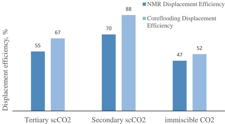
**Figure 4.11.** Displacement efficiencies obtained from NMR and core-floods.
