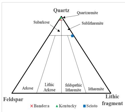
**Figure 2.5.** Classification of sandstone after Folk criterion, where Bandera and Kentucky sandstones could be classified as quartzarenite, while Scioto sandstone can be classified as Sublitharenite [69].
