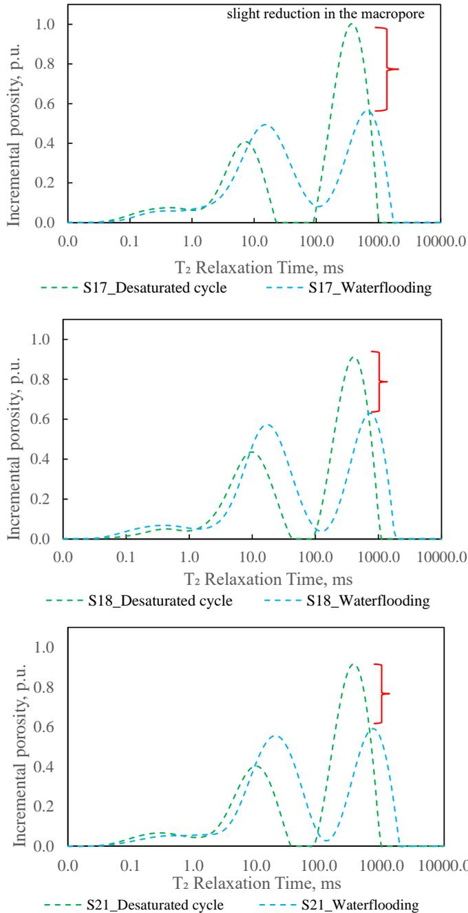
**Figure 4.9.** NMR T<sub>2</sub> curves of desaturated (green dashed line) and waterflooded (light blue dashed line) of composite core #1. A slight reduction in the macropore indicates poor displacement because of waterflooding (marked in red brace), while the extended NMR T<sub>2</sub> (light blue dashed lines) are due to the delay of surface relaxation caused by the remaining n-decane retained in the rock pore system.
