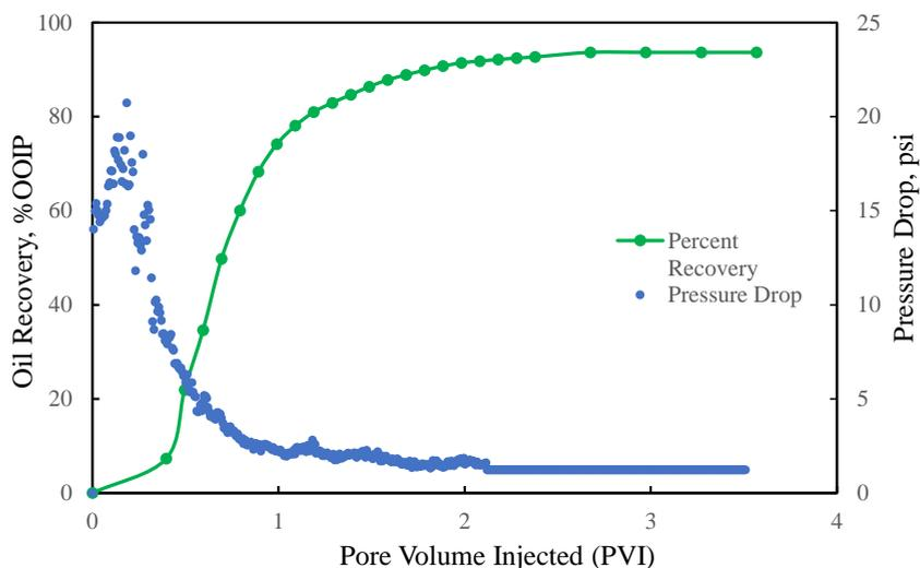
**Figure 4.3.** Oil recovery and pressure drop profile of miscible secondary CO<sub>2</sub> injection conducted on composite core #2.
