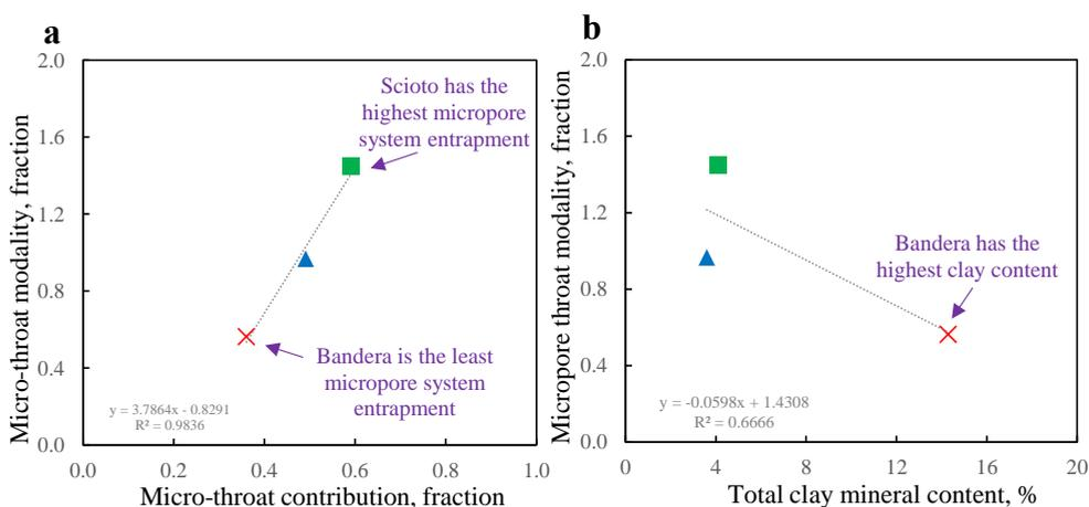
**Figure 3.6.** Cross-plots showing the relationship of micro-throat modality ratio of tested sandstones with: (a) micro-throat proportion; (b) total clay mineral content. (Note the trendlines show the relation between measurements).
