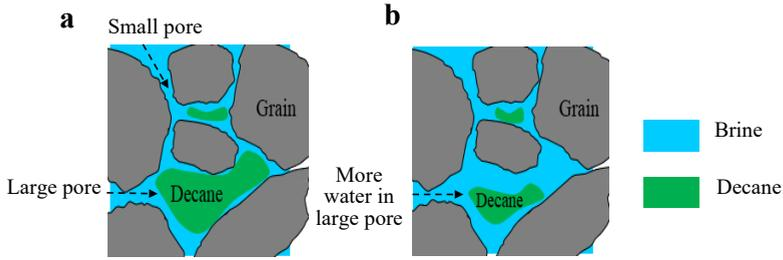
**Figure 4.10.** Schematic illustrating the drainage and waterflood covering. (a) Decane-desaturated case, where decane resides in big pores and water resides in small pores. (b) Waterflooding case showing brine imbibing big pores causing a slight reduction in decane saturation.
