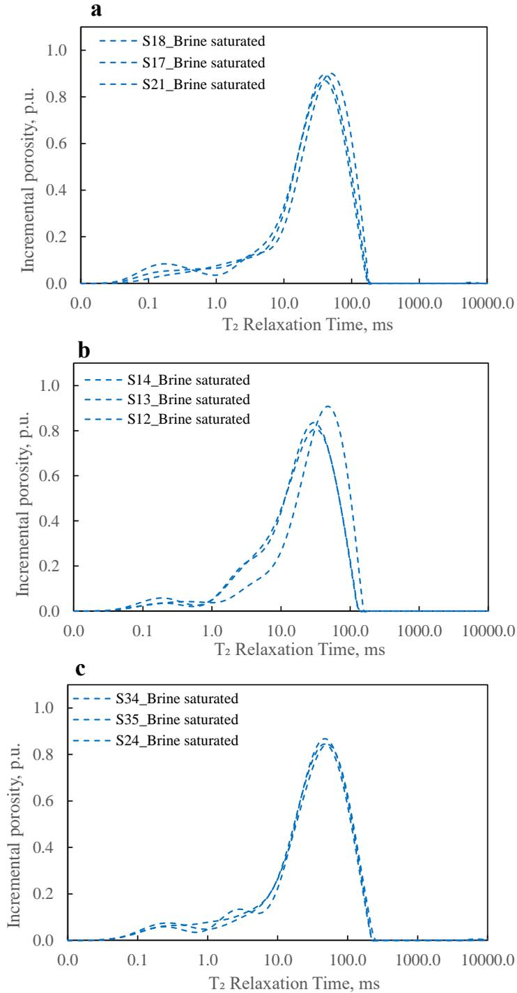
**Figure 4.5.** NMR T<sub>2</sub> measurements of brine-saturated composites of Scioto sandstone: **(a)** Composite #1; **(b)** Composite #2; and **(c)** Composite #3.
