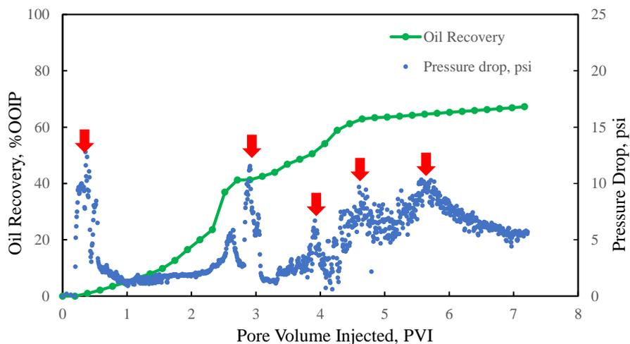
**Figure 4.4.** Oil recovery and pressure drop profile of immiscible secondary CO<sub>2</sub> injection conducted on composite core #3.
