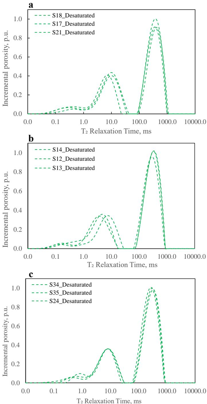
**Figure 4.6.** NMR T<sub>2</sub> measurements of desaturated composites of Scioto sandstone: (a) Composite #1; (b) Composite #2; and (c) Composite #3.
