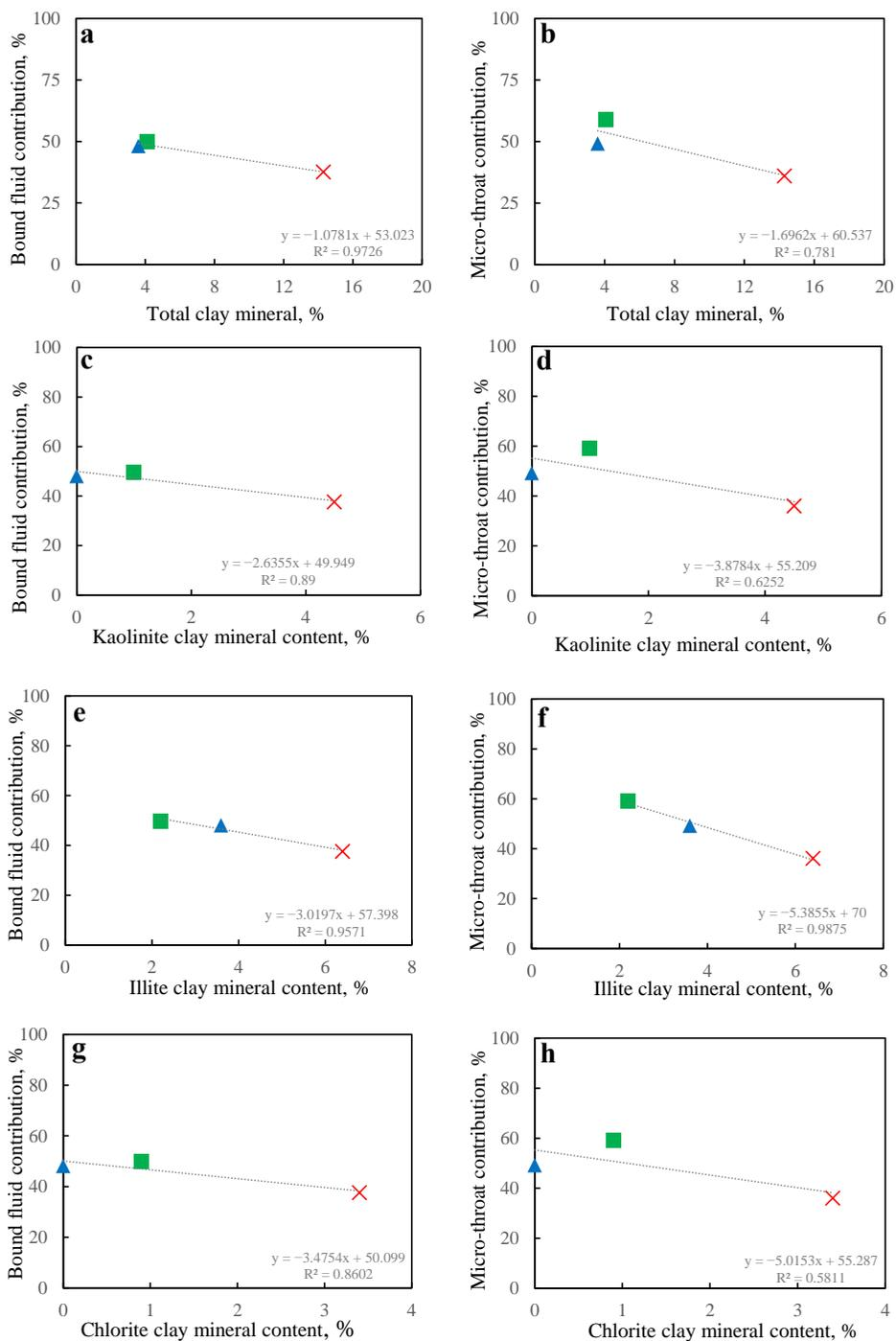
**Figure 3.3.** Cross-plots of bound-fluid contribution, micro-throat proportion and clay mineral content with: (a, b) total clay mineral content; (c, d) kaolinite clay content; (e, f) illite clay content; (g, h) chlorite clay content. (Note the trendlines show the relation between measurements).
