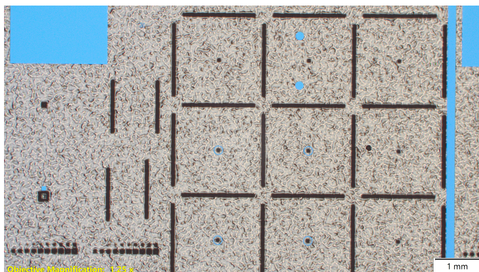
Figure 4.11: Example of rough surface of the spray-coated photoresist.
