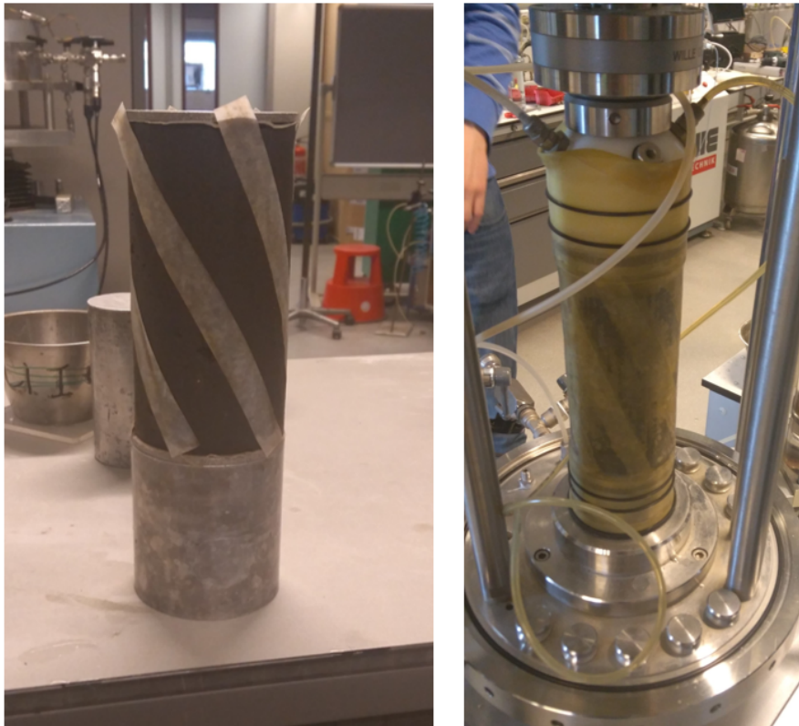
Figure 3.1: Left: drainage strips on the sample. Right: placement of the sample in triaxial apparatus
