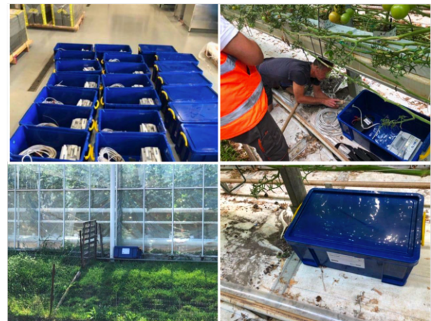
Figure 4: Installation of the seismic sensors that monitored the geothermal operation of Nature's Heat project in Kwintsheul, The Netherlands.
