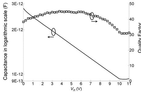
Fig. 6. Measured  $C-V_R$  and  $Q-V_R$  dependence at 2 GHz. Note that the  $C(V_R)$  measurements yield a straight line in the logarithmic plot as a function of reverse voltage, indicating a near-ideal exponential  $C(V_R)$  relationship.
