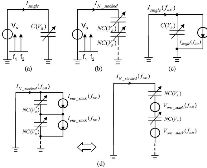
Fig. 2. (a) Schematic for a single-varactor stack; (b) schematic for the  $N$ -varactor stacks; (c) schematic to calculate third-order or fifth-order response for the single varactor stack; and (d) schematic to calculate third-order or fifth-order response for the  $N$ -varactor stacks.
