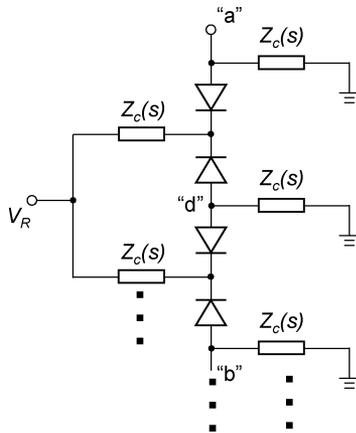
Fig. 3. Multistack topology for the NTSVS.
