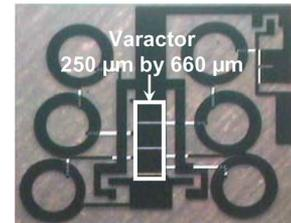
Fig. 5. The 2.7 pF three-stacked NTSVS used for the measurements (six 20 nH inductors are used to implement the harmonic baseband "short" while providing high impedance for the fundamental and harmonics).
