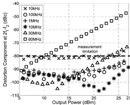
Fig. 7. Measured distortion components at  $2f_1 - f_2$  versus output power at different tone spacings for a two-tone input signal with the  $f_{center}$  of 2 GHz (capacitance at zero bias voltage = 2.7 pF,  $V_R = 5$  V).
