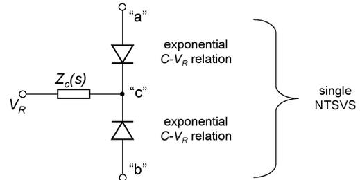
Fig. 1. Narrow-tone spacing varactor stack (NTSVS).  $Z_c(s)$  is used to fulfill specific harmonic termination conditions for  $IM_3$  cancellation.
