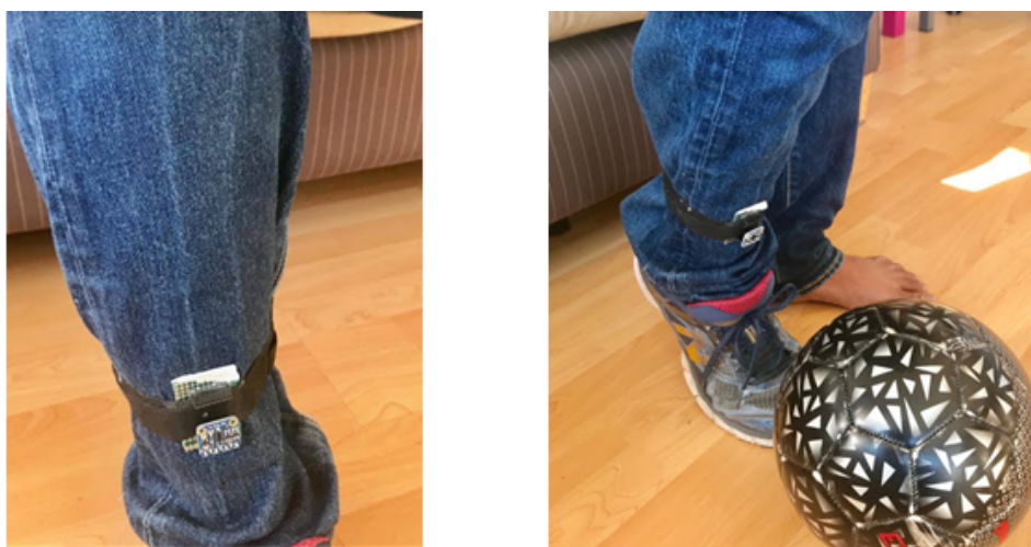
Figure 6.4: Mounting of ToF sensor on leg
