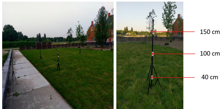
Figure 4.5: Nodes mounted at different heights on a metallic tripod (right) in a predetermined field setup (left)
