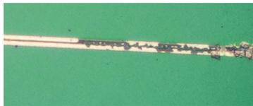
(d) Regular microscope picture of the Al line that should be  $5\mu\text{m}$  wide (black line in the middle, which in the top picture is visible on the right and in the bottom picture on the left), but is smaller and the TiN is severely damaged.
