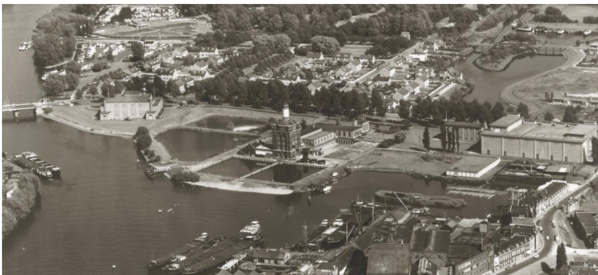
Figure 17 An aerial photograph of the Watertoren terrein from 1964. The image depicts the added steel tube and the two removed basins (Source: RegionaalArchiefDordrecht, n.d.).
