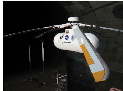
(b) Active flap on a rotor blade
