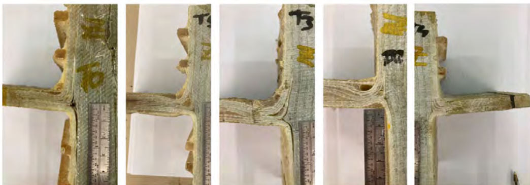
Figure 10. Failure initiation and delamination. Static component tests.
