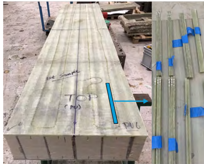
Figure 1. Coupons cut out from the sandwich panel.
