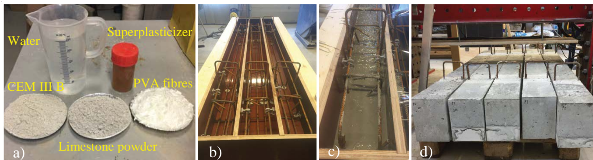
Figure 2 a) SHCC mix constituents b) before and c) after casting of SHCC d) whole beams
