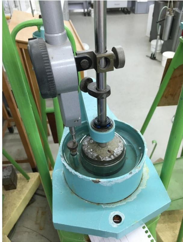
Figure G.12: Consolidation test, note the salt deposition
