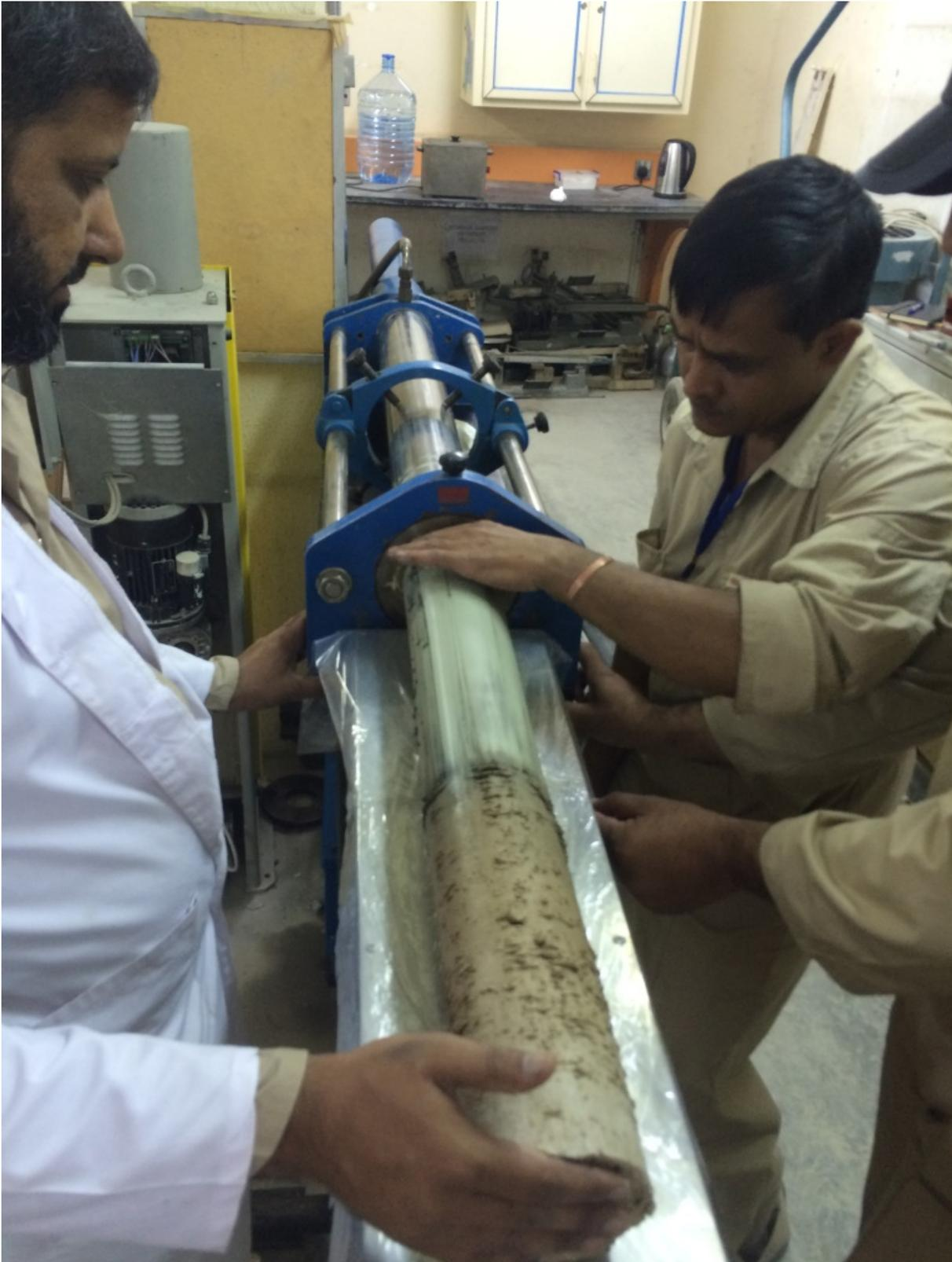
Figure F.6: Extruding the sample from the Shelby tube.
