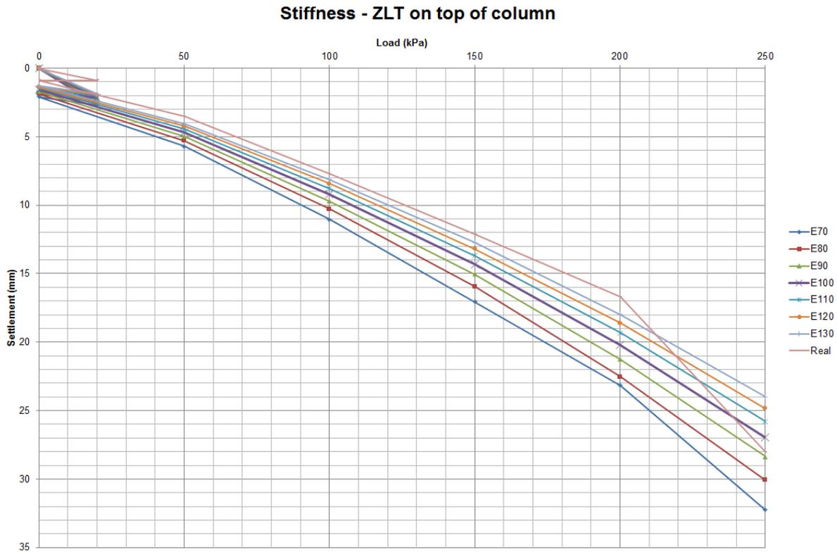
Figure I.3: ZLT between columns, varying platform stiffness
