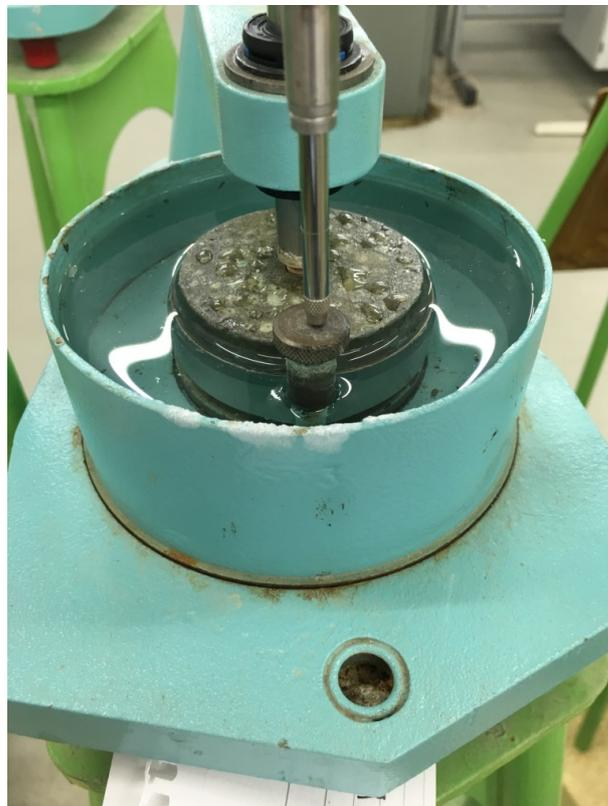
Figure G.13: Consolidation test, note the salt deposition
