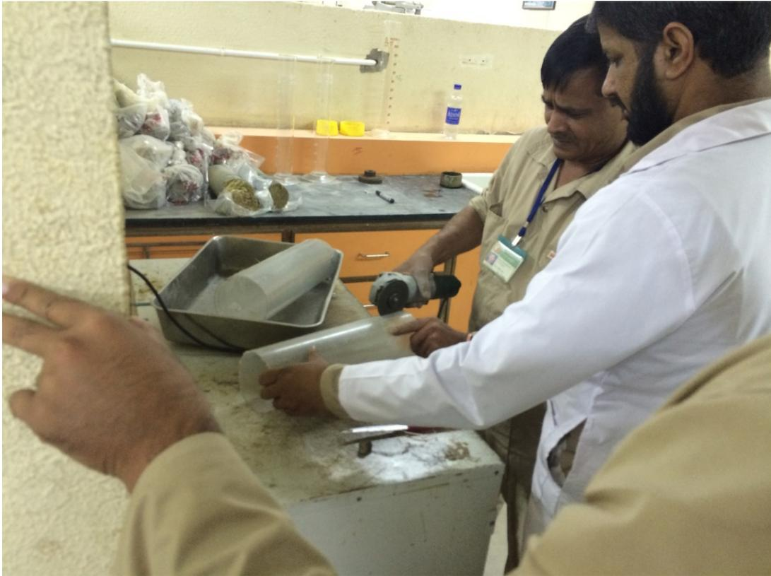
Figure F.9: Sawing the tubes lengthwise to allow for a nearly disturbance-free wrapping of the sample.
