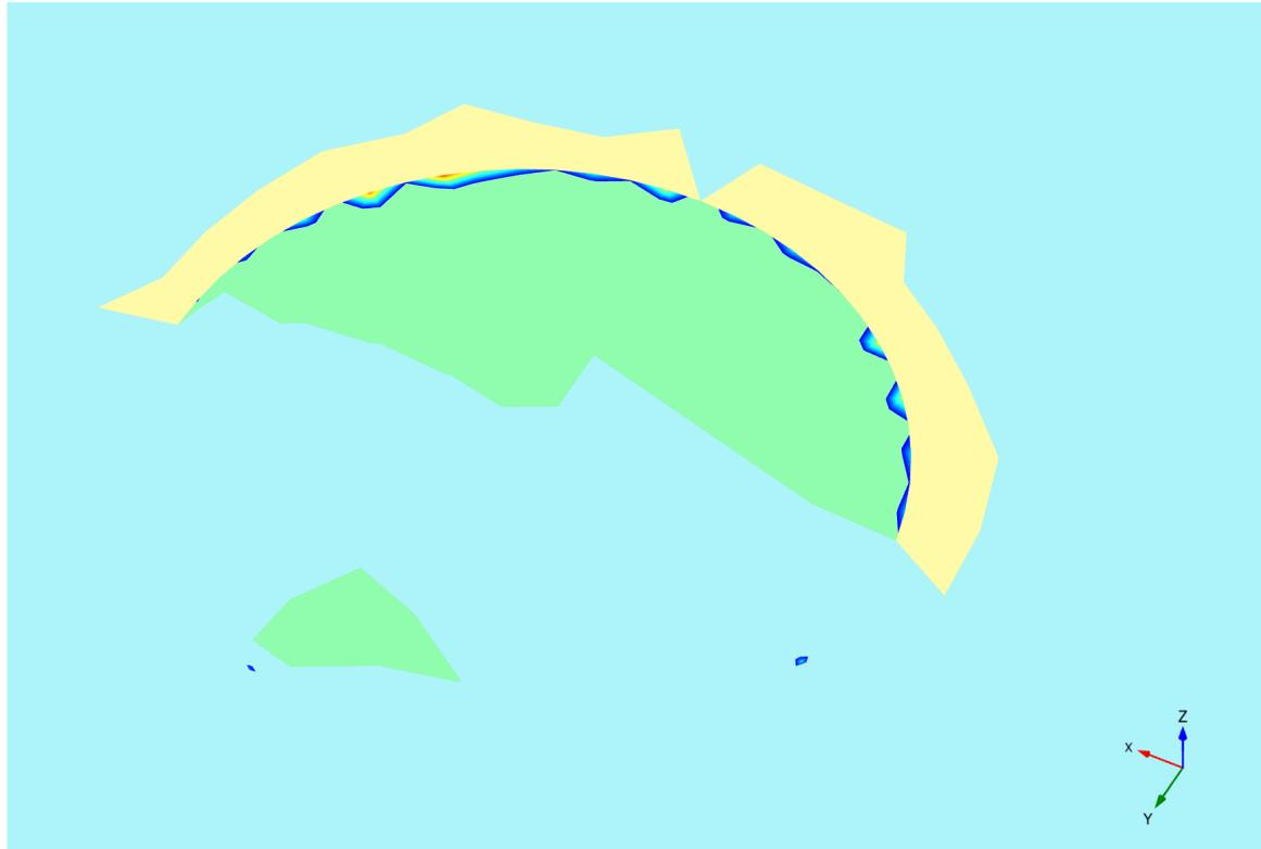
Figure I.12: Interpolation error near the edges of the sand column
