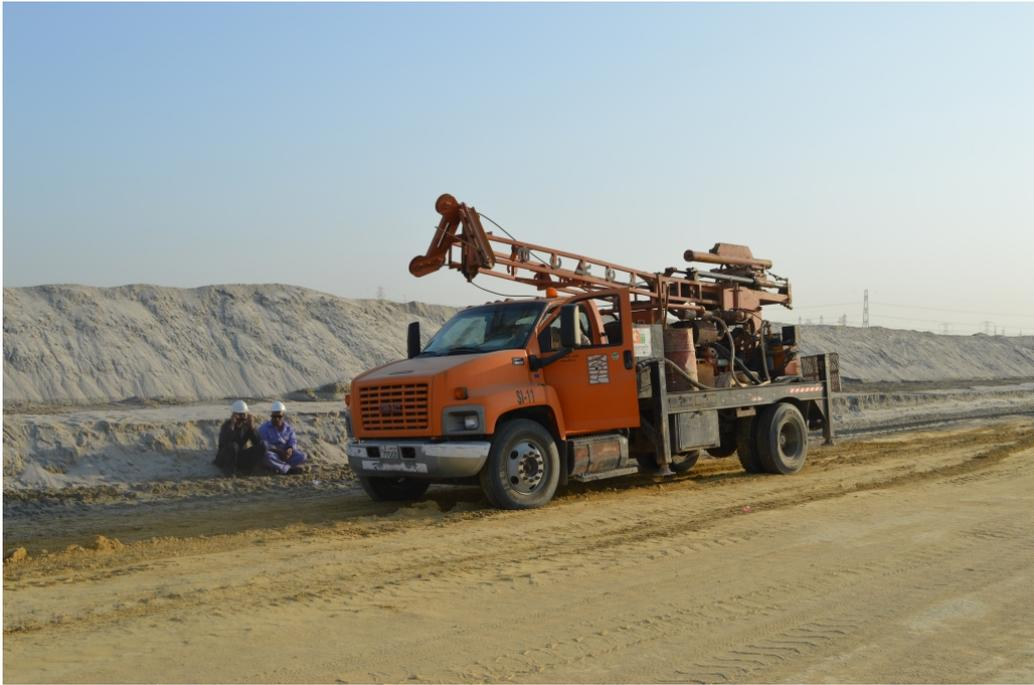
Figure F.2: The drilling rig mounted on a truck.
