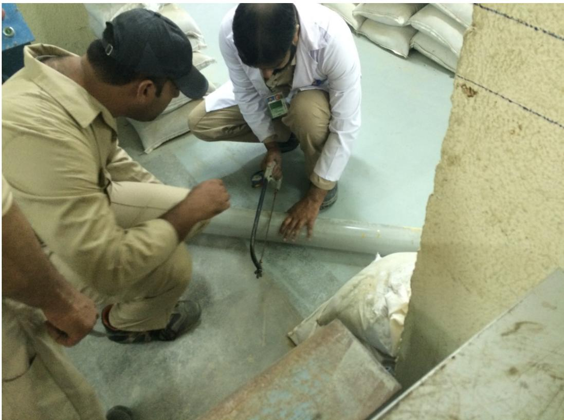
Figure F.8: Sawing the tubes in parts. The tubes should contain the samples for transport.
