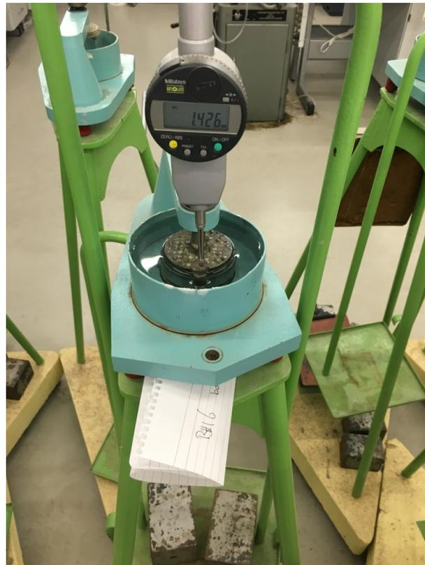
Figure G.11: Consolidation test
