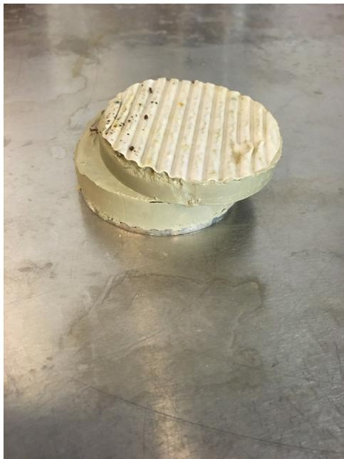
Figure G.19: Shear strength test sample after shearing
