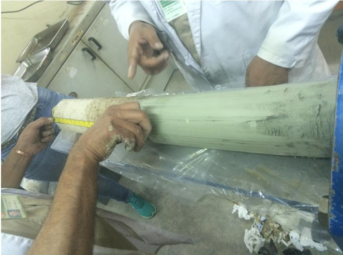
Figure F.7: Measuring the length of the layers of interest (the sabkha).
