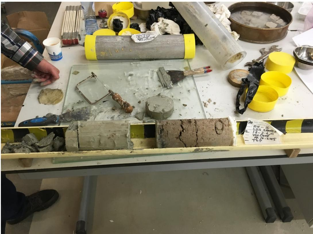
Figure F.14: Extruding samples from the packaged tubes. Note the layering inside the sample.
