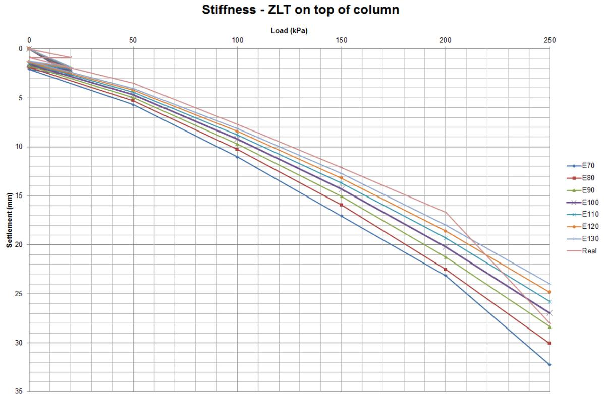
Figure I.7: ZLT on top, varying platform stiffness
