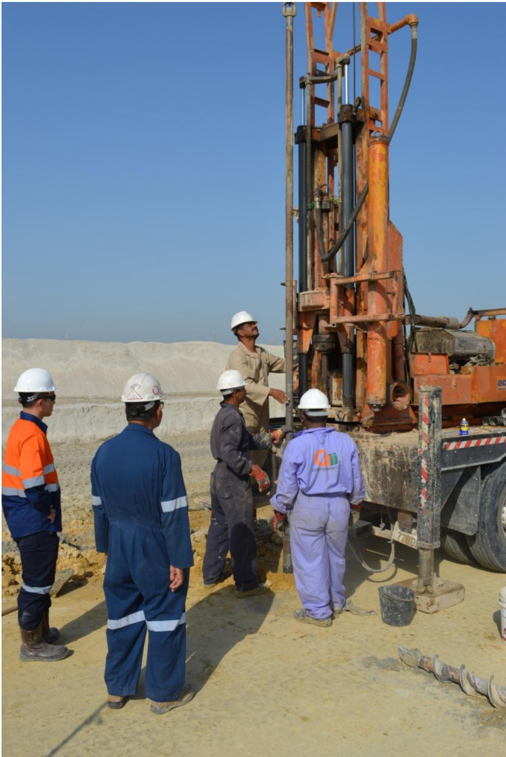
Figure F.1: The drilling rig mounted on a truck.
