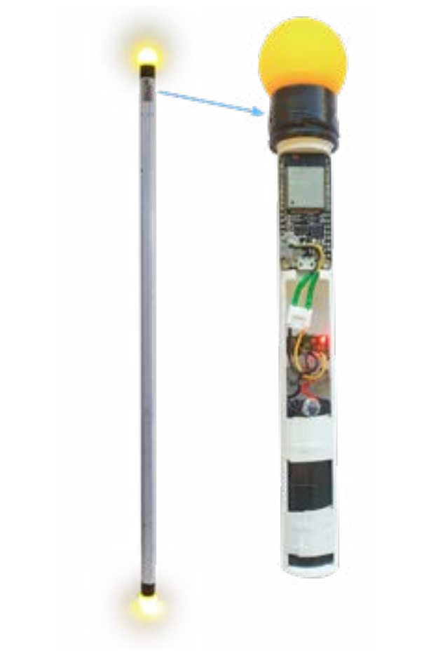
Figure 61: Testing prototype. left the overview right the probe that is inside with the battery, inertial measurement unit and arduino
