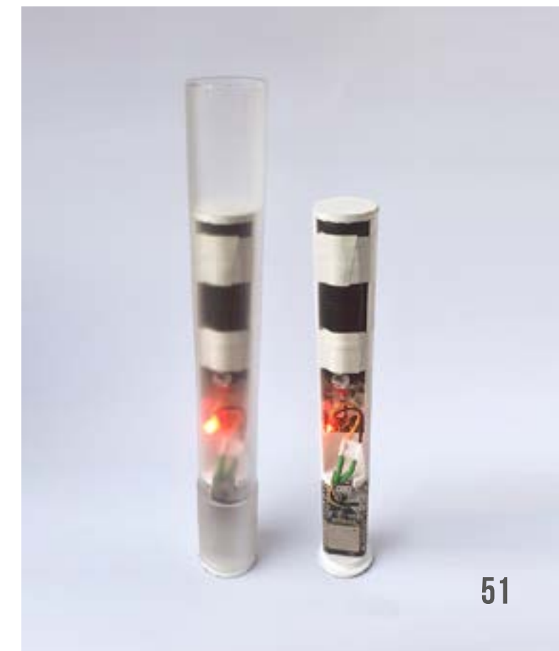
Figure 27: Arduino, IMU and battery inside a 3D printed housing
