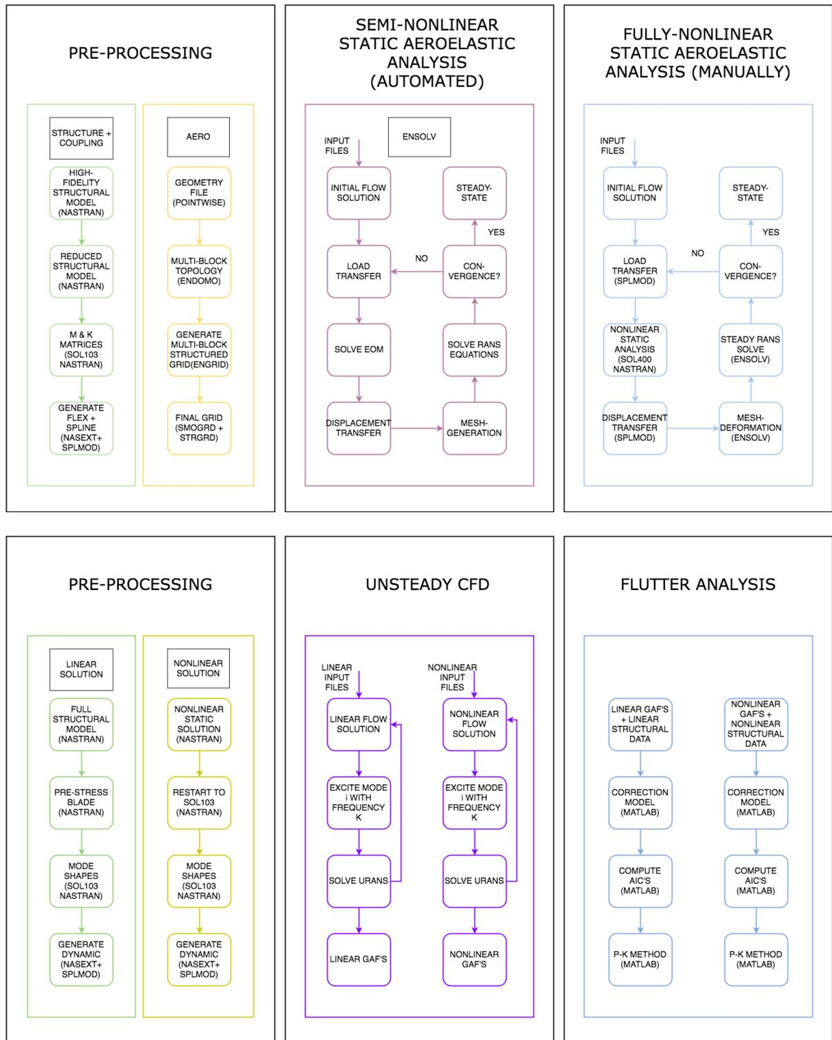
Figure 3.6: Overview of the entire analysis set-up
