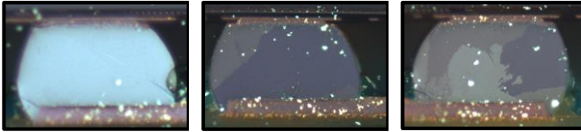
Figure 5: Single and Oligocrystalline Solder Joint
