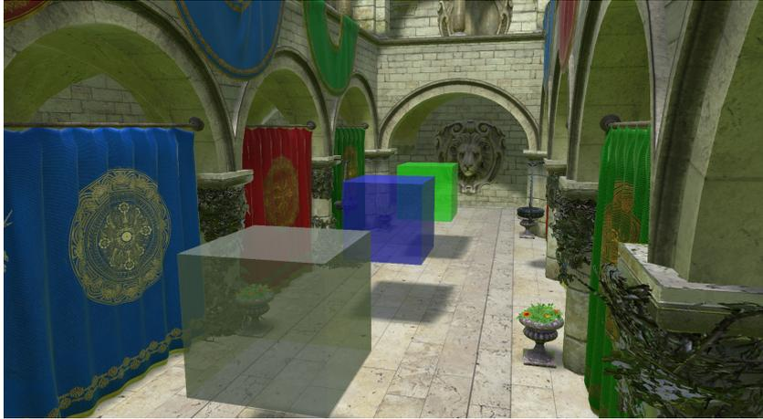
Figure 5.2: Our implementation of stochastic transparency in action, with 8 samples and stratified sampling. Here the cubes are half transparent ( $\alpha = 0.5$ ), while the rest of the scene is opaque.
