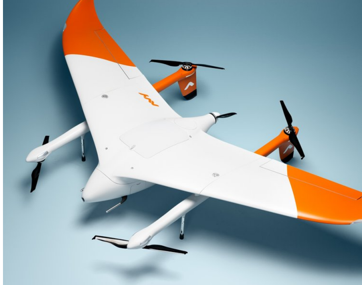
Figure 2: Photo from the eVTOL Avy Aera 3, built by the company Avy. The drone takes off and lands vertically as an octocopter, using the 4 vertical rotors. For forward flight manoeuvres, the horizontal propeller is used while the 4 rotors can also operate if additional trajectory stabilization and manoeuvrability is needed.
