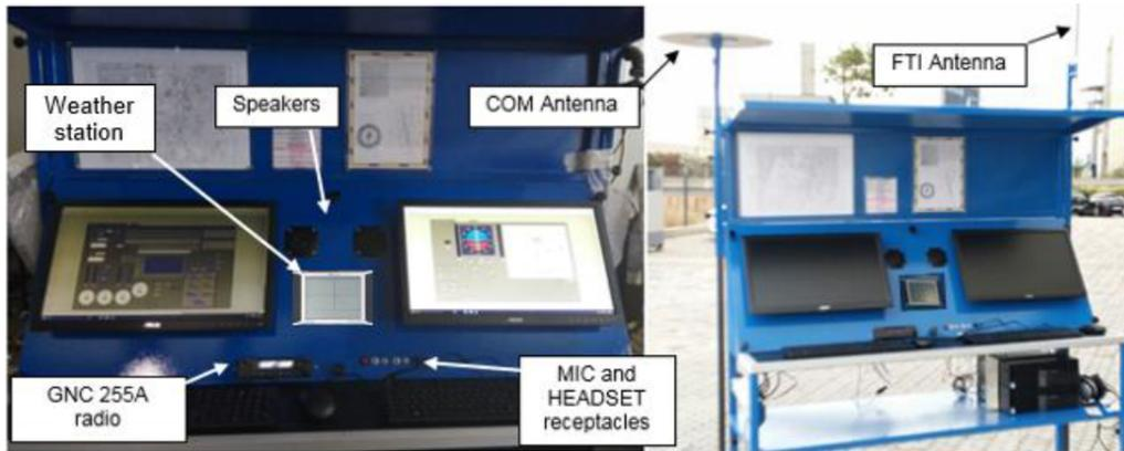
Figure 3.3: Ground station layout
