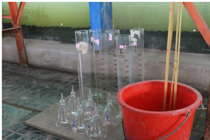
Figure 3.5: Containers of the collected water-sediment samples: six glass cylinders and six pycnometers.
