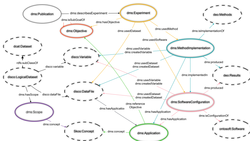
Figure E.5: Linking Datasets, Methods and Software. The ovals with different colors used in the figure are an indicator of different classes that we defined, and the dashed ovals are an indicator of old classes that were defined by the existing ontologies.
