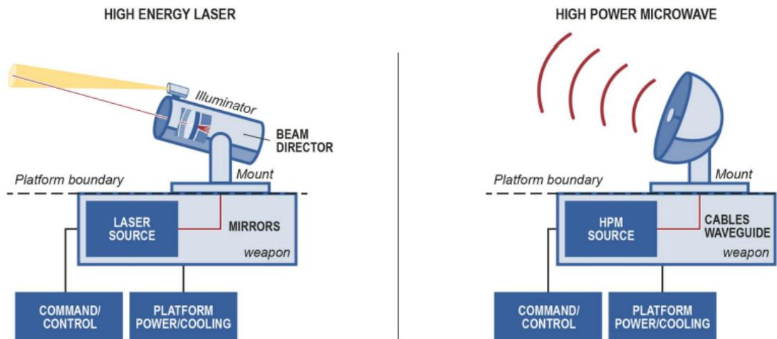
Figure 4.3: Illustration of modelled HEL and HPM systems [15]
