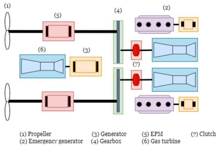
**Figure C.3:** Hybrid propulsion configuration suggested for an SMR prime mover in chapter 8
