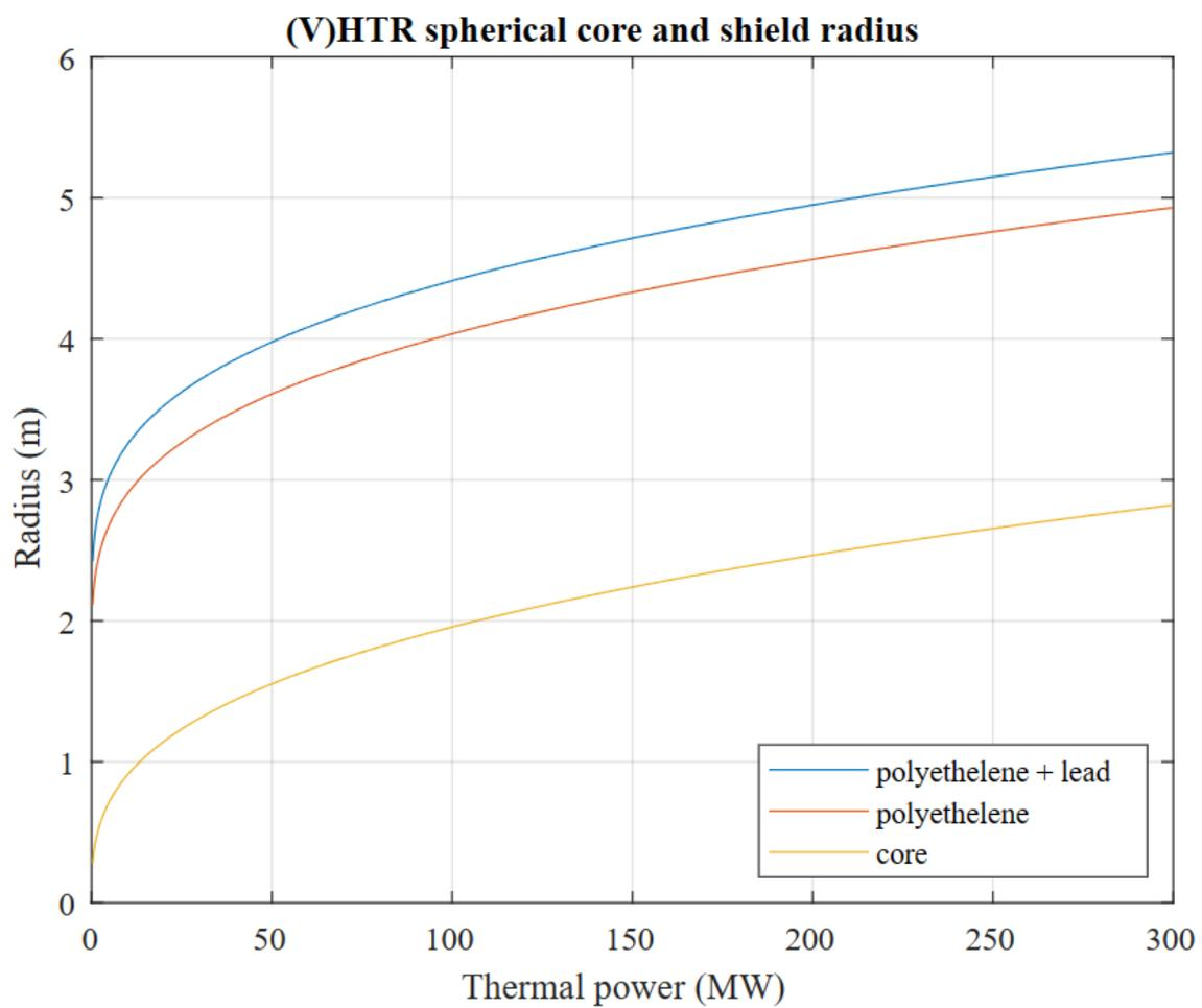
**Figure H.1:** The radius of the core and different shielding materials over thermal power of the (v)HTR
