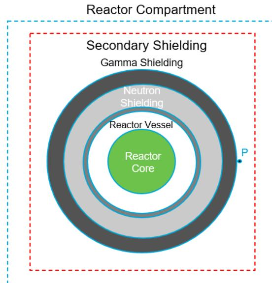
**Figure 5.4:** Schematic of a spherical reactor core surrounded by a spherical shield
