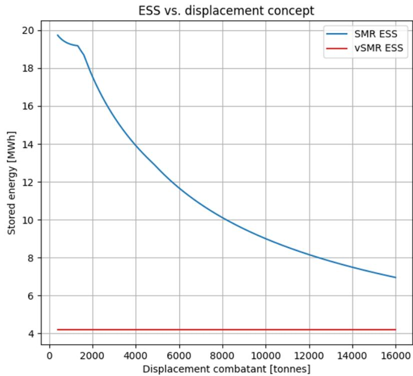
**Figure O.2:** Required ESS for (v)SMR technology for a SEWACO load of  $28MW_e$  (twice the initial load)
