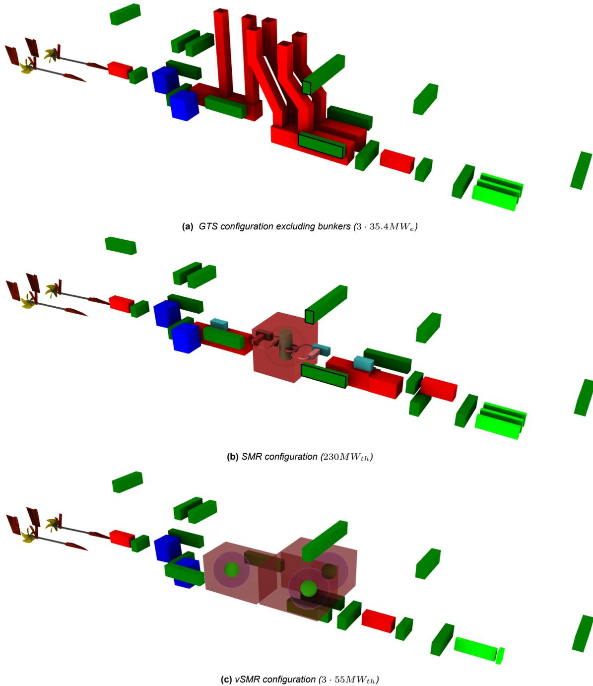
**Figure P.5:** Preliminary design viewing power generation, distribution and conversion components without hull. Power generation; red, power distribution; green, ESS; bright green and power conversion; blue.
