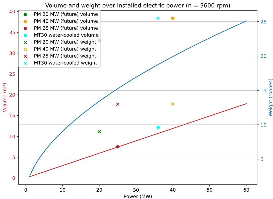
**Figure 6.6:** Size and weight of naval generator with a shaft speed of 3600 RPM
