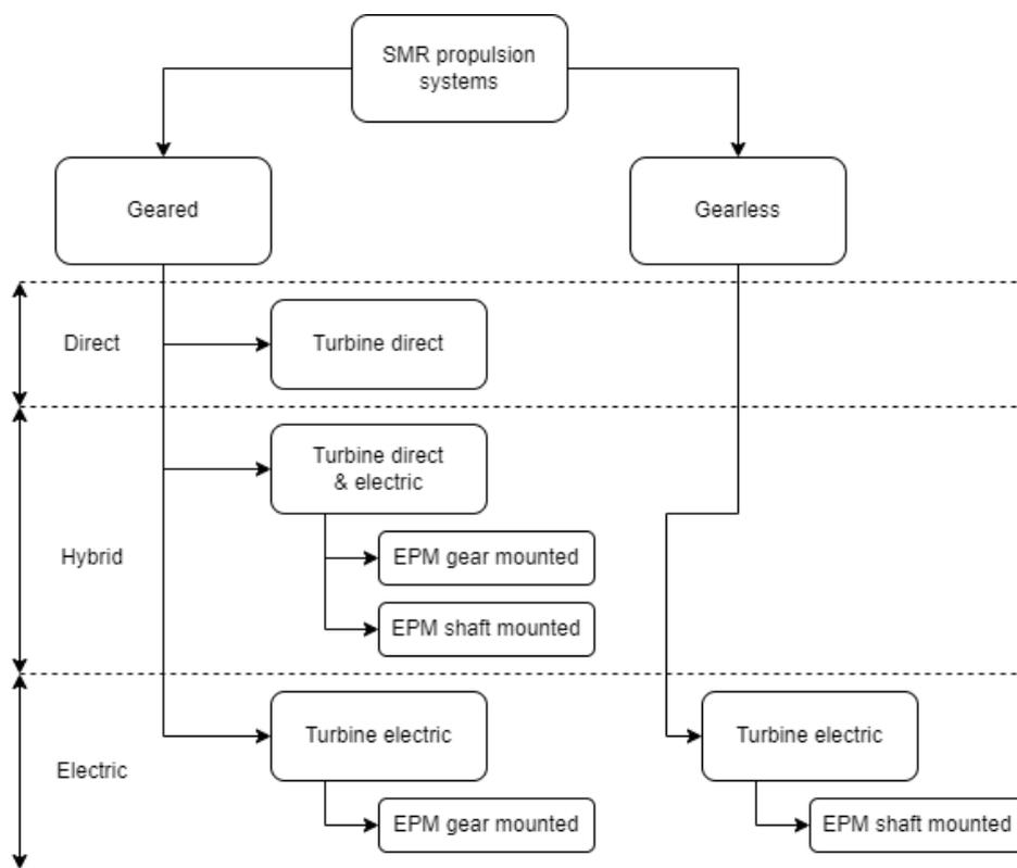
**Figure C.1:** Classification of SMR propulsion configurations
