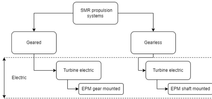
Figure 7.10: Classification of (v)SMR power distribution layouts using IPS
