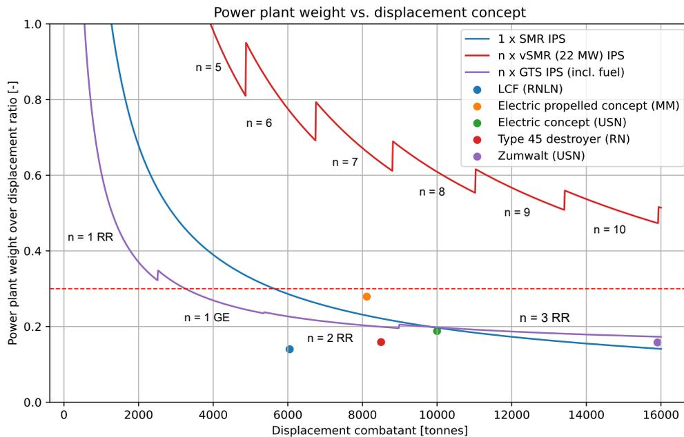
Figure 8.4: The weight impact of the power plant on the displacement of the combatant
