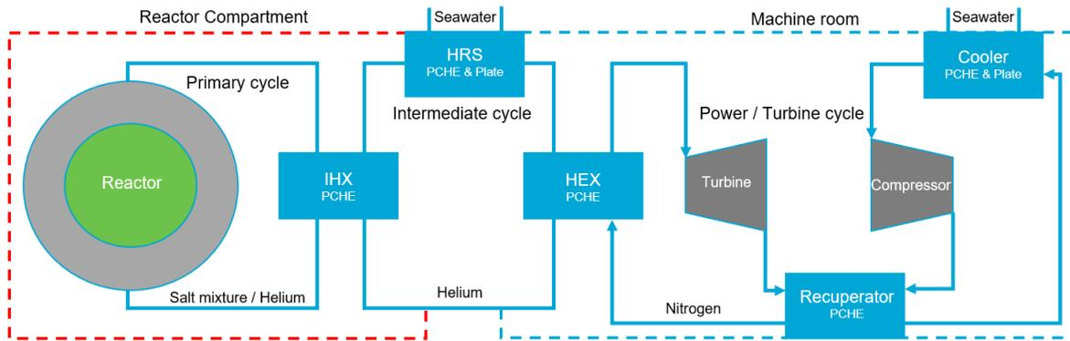
Figure 6.3: Schematic of required heat exchangers
