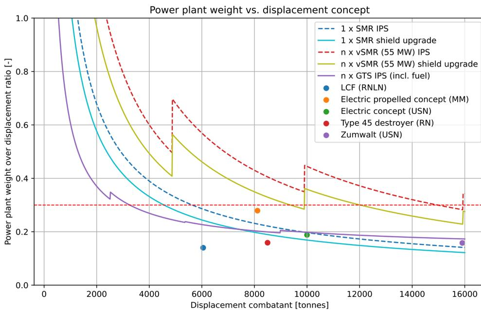
**Figure 8.10:** Soution 2, the weight impact of the power plant on the displacement of the combatant with an accomplished shield reduction of 30%
