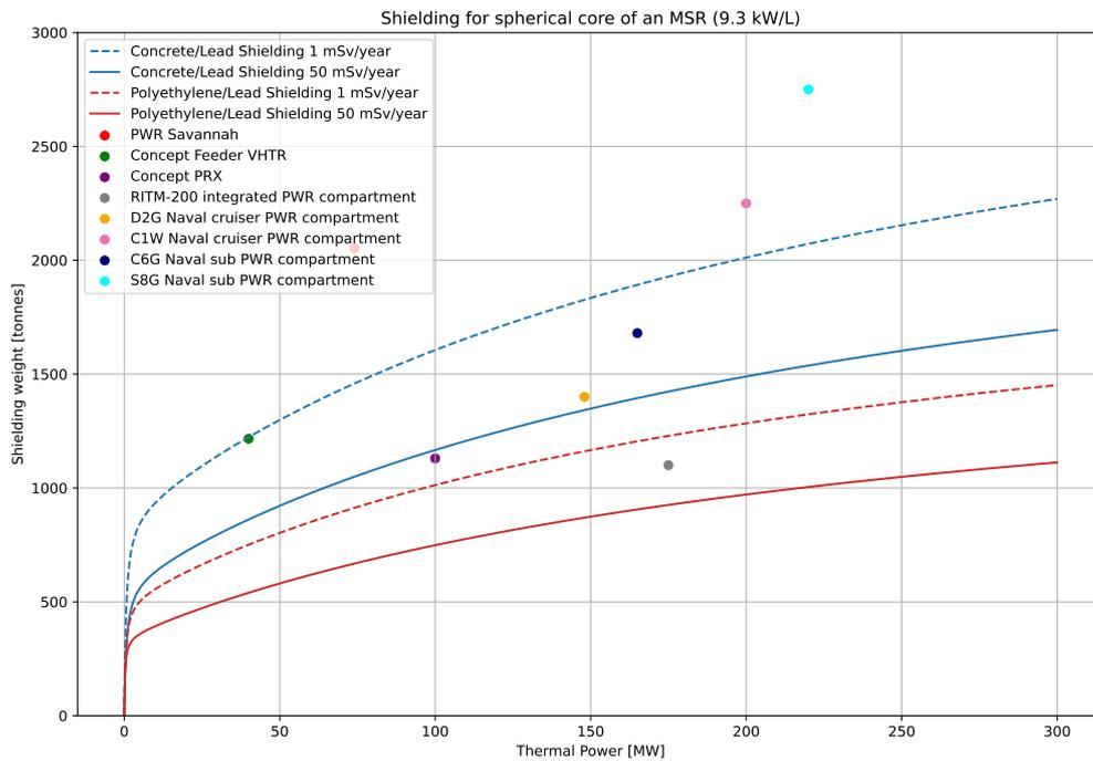
**Figure 5.6:** Shielding weight over installed thermal power for an MSR including reference designs
