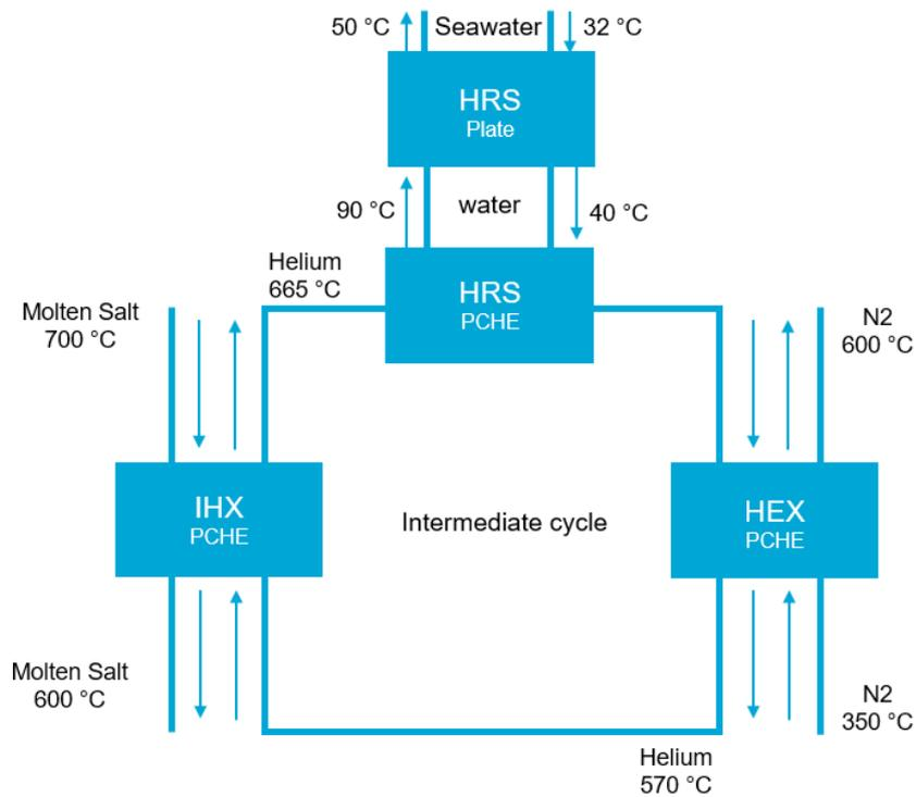
Figure K.1: Intermediate cycle
