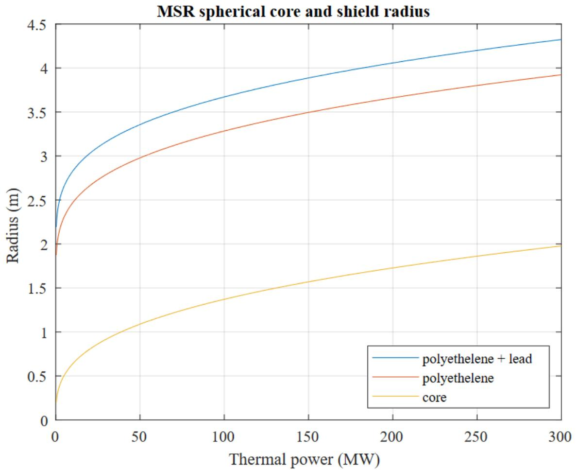
**Figure H.2:** *The radius of the core and different shielding materials over thermal power of the MSR*
