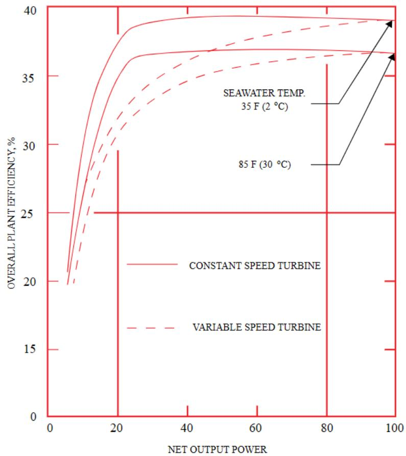
Figure J.1: Plant efficiency vs output power in % of the installed turbine power [54]
