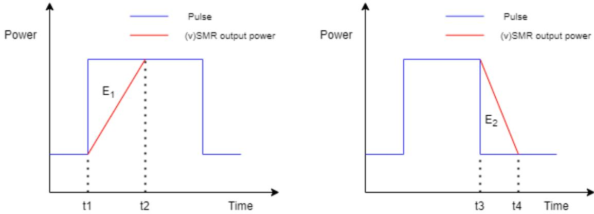
Figure 4.4: Example power profile during ramp up (left) and ramp down (right) period
