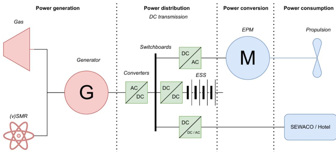
**Figure 7.1:** Schematic power train for conventional (gas) or nuclear (SMR) technology
