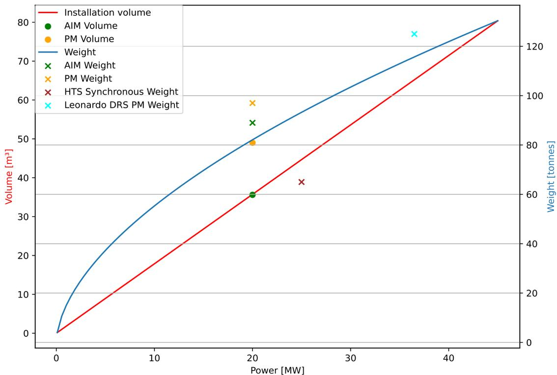
Figure 7.11: Size and weight of naval EPMs with a shaft speed of 150 RPM
