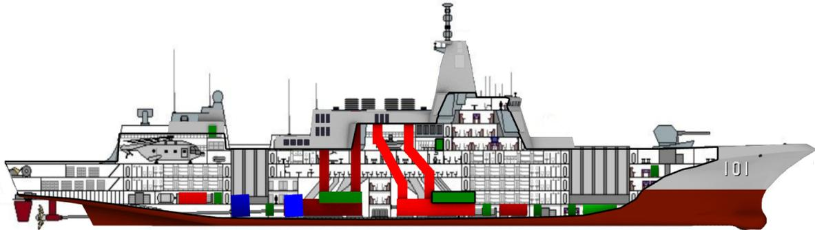
**Figure 9.1:** Side view of the conventional baseline visualising the GTS with IPS, including the preliminary general arrangement. Power generation; red, power distribution; green, ESS; bright green and power conversion; blue.
