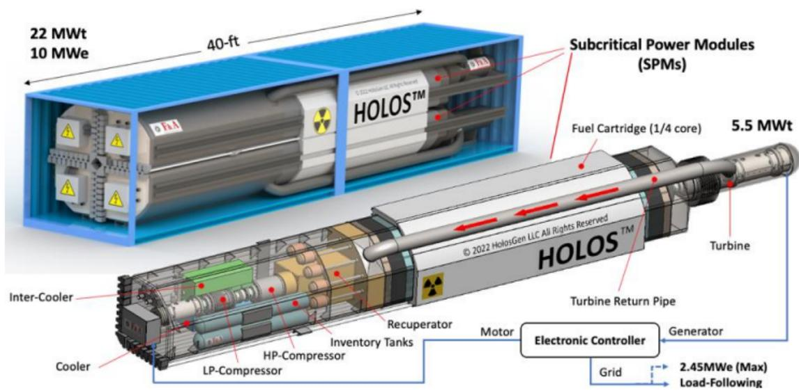
Figure B.1: Detailed Holos-Quad layout with component labels ( $22\text{MW}_{th}$ ) [8]
