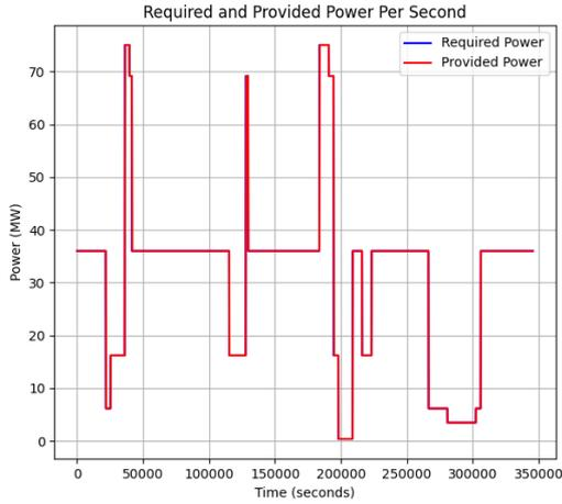
**Figure 7.8:** Required and provided power for  $P_{tot}$  ( $8 \cdot P_e = 10MW$  and  $f_{ramp} = 10$ )
