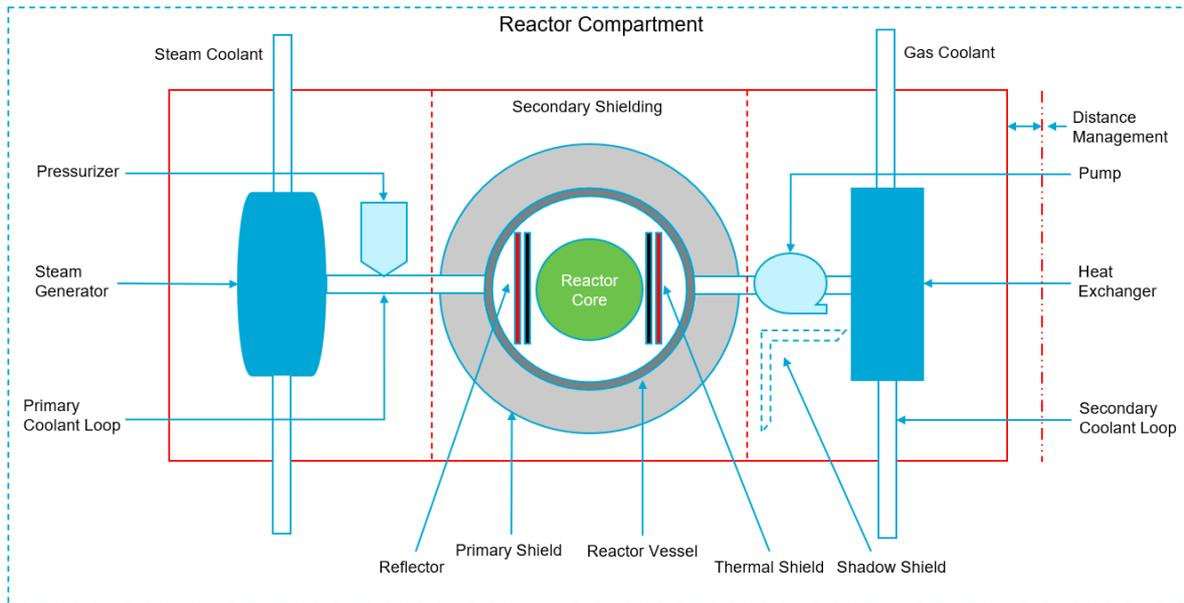
**Figure 5.3:** Schematic of a reactor compartment shield with water (left) and gas (right) coolant
