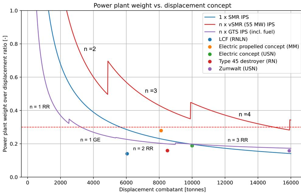
**Figure 8.9:** Solution 1, the weight impact of the power plant on the displacement of the combatant including a more powerful vSMR
