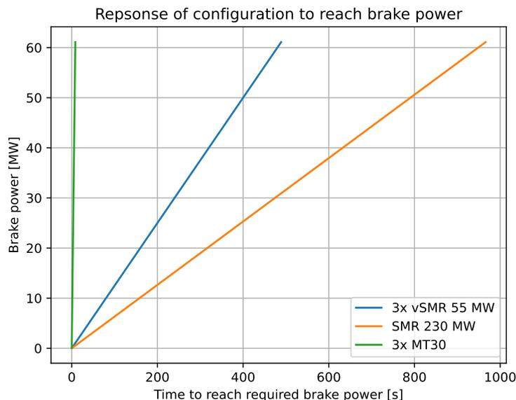
**Figure 9.4:** The response time to reach a brake power level for the GTS and (v)SMR configuration of the future surface combatant
