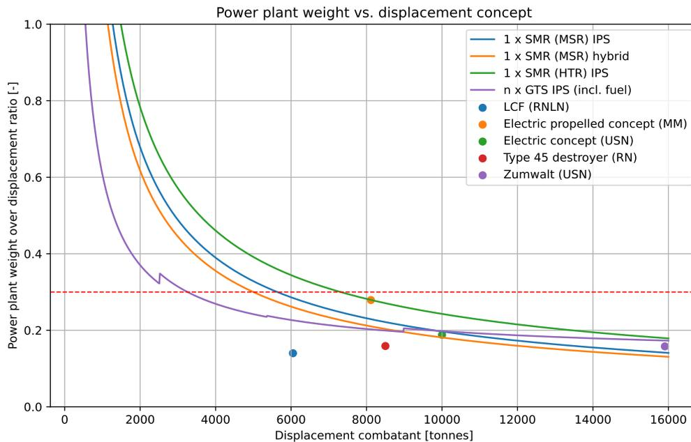
**Figure 8.6:** The weight impact of the power plant on the displacement of the combatant with a hybrid and HTR configuration. For  $n$ , see figure 8.4
