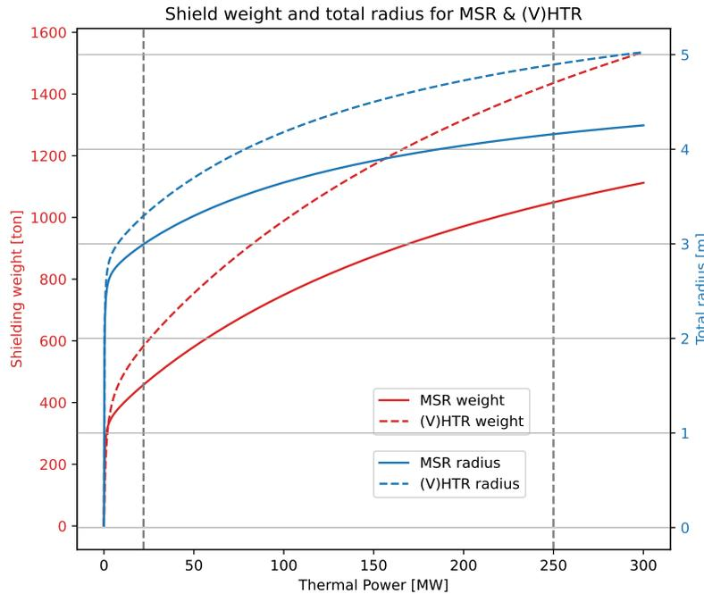
Figure 5.7: Shielding weight and radius over installed thermal power for an MSR and (V)HTR
