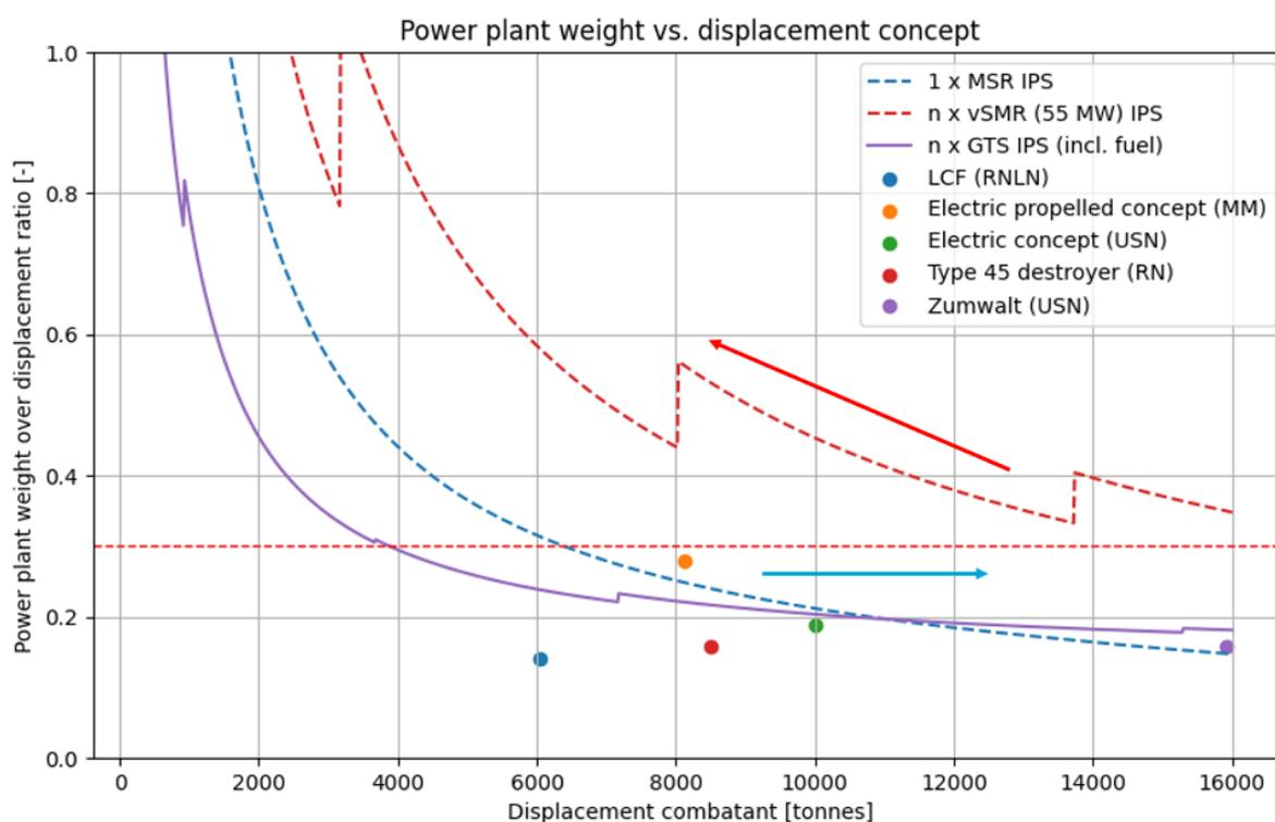
**Figure O.1:** The weight impact of the power plant on the displacement of the combatant for a SEWACO load of  $28M W_e$  (twice the initial load). The weight ratio of the SMR moves slightly to the left (blue arrow). After an increase in SEWACO load, the weight ratio of the vSMR moves to the right and upwards (red arrow).
