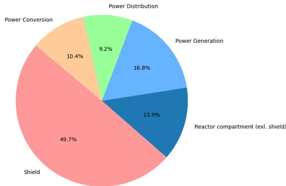
**Figure 8.7:** Weight distribution of the modelled SMR power plant for a 10,000 tonnes combatant
