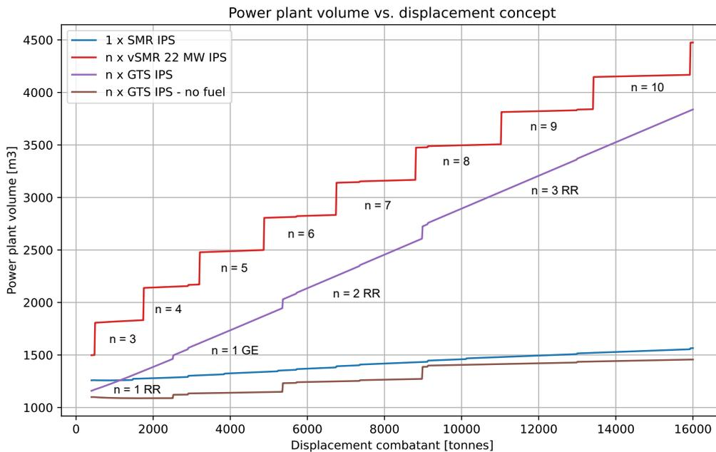
**Figure 8.5:** The volume impact of the power plant on the displacement of the combatant excluding cables, pipes and exhausts
