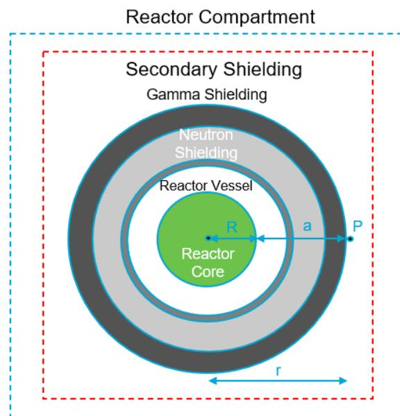
**Figure F.1:** Spherical reactor core surrounded by a spherical shield with parameters
