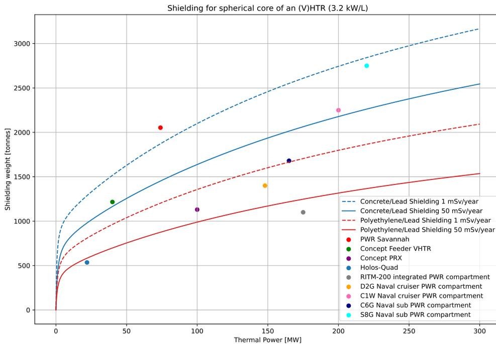
**Figure 5.5:** Shielding weight over installed thermal power for a (V)HTR including reference designs
