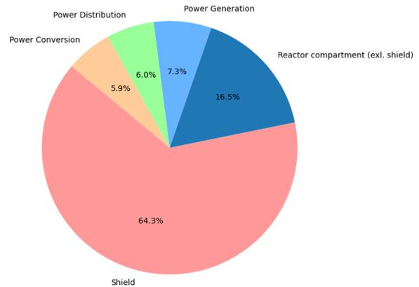
**Figure 8.8:** Weight distribution of the modelled vSMR power plant for a 10,000 tonnes combatant
