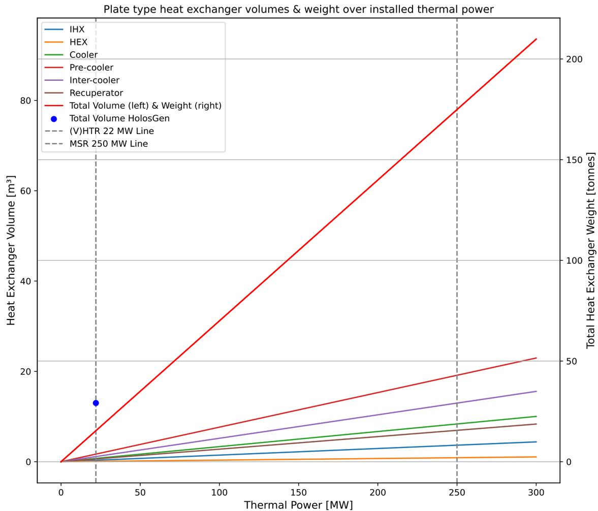
Figure 6.4: Heat exchanger volume (left) and weight (right)
