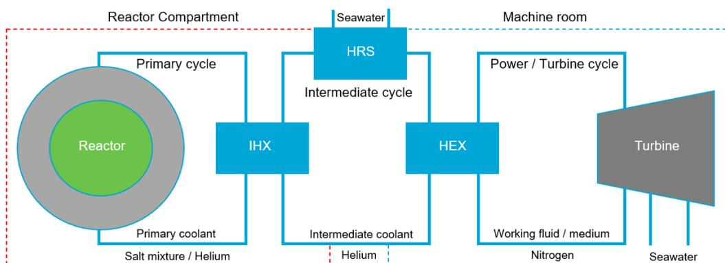
**Figure 6.1:** Schematic of closed cycles and the operating mediums
