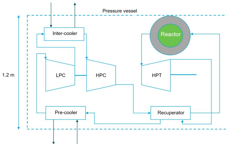
**Figure 6.2:** Schematic of the vSMR direct closed Brayton cycle
