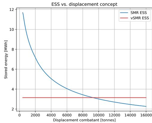
**Figure 8.3:** Required ESS for (v)SMR technology ( $10MW_e$  vSMR)
