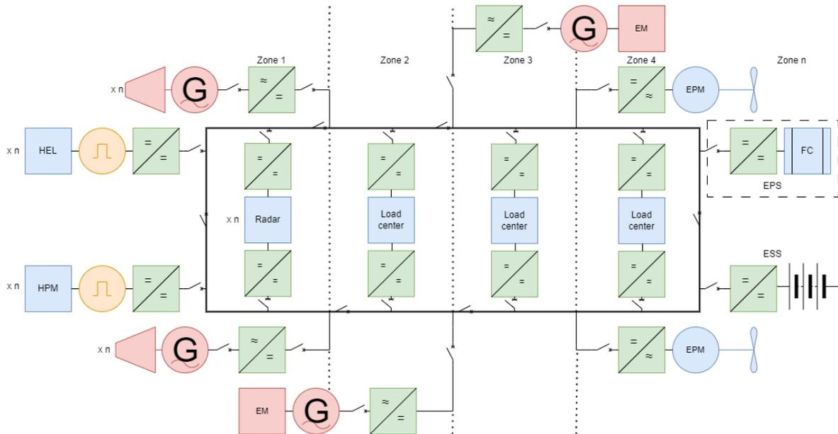
Figure 7.2: Main power distribution system for a future surface combatant using IPS
