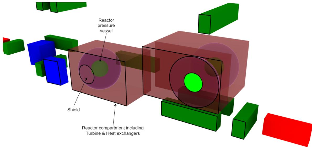
**Figure P.3:** *vSMR layout with component labels ( $3 \cdot 55 MW_{th}$ )*
