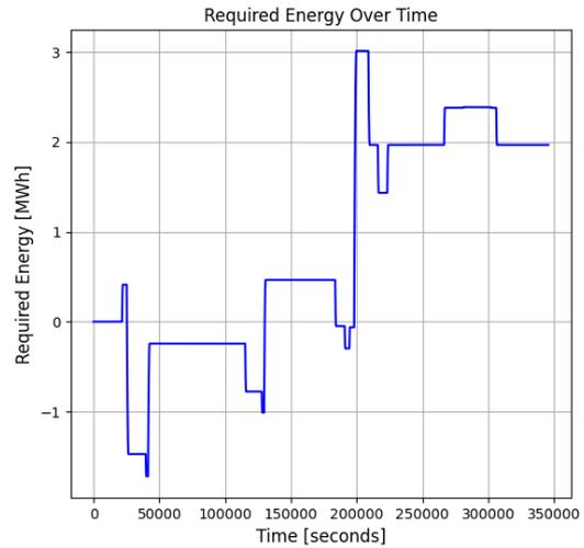
**Figure 7.5:** Required ESS capacity ( $P_{th} = 230\text{MW}$ ,  $f_{ramp} = 5$  and  $f_{ESS} = 0.1$ )
