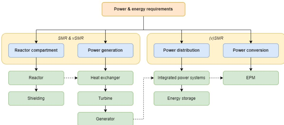
**Figure 3.3:** Design structure for the SMR and the vSMR
