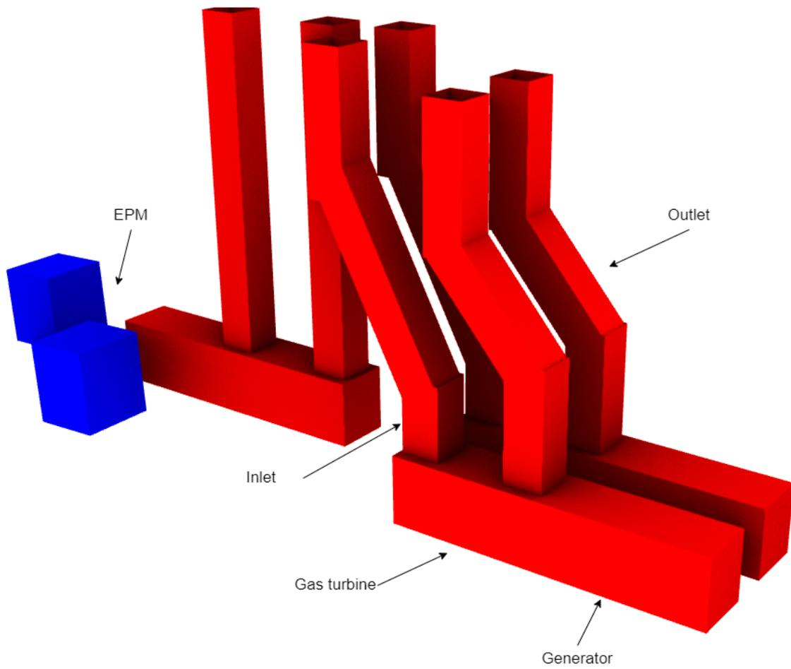
**Figure P.1:** Conventional GTS layout with component labels ( $3 \cdot 35.4\text{MW}_e$ )
