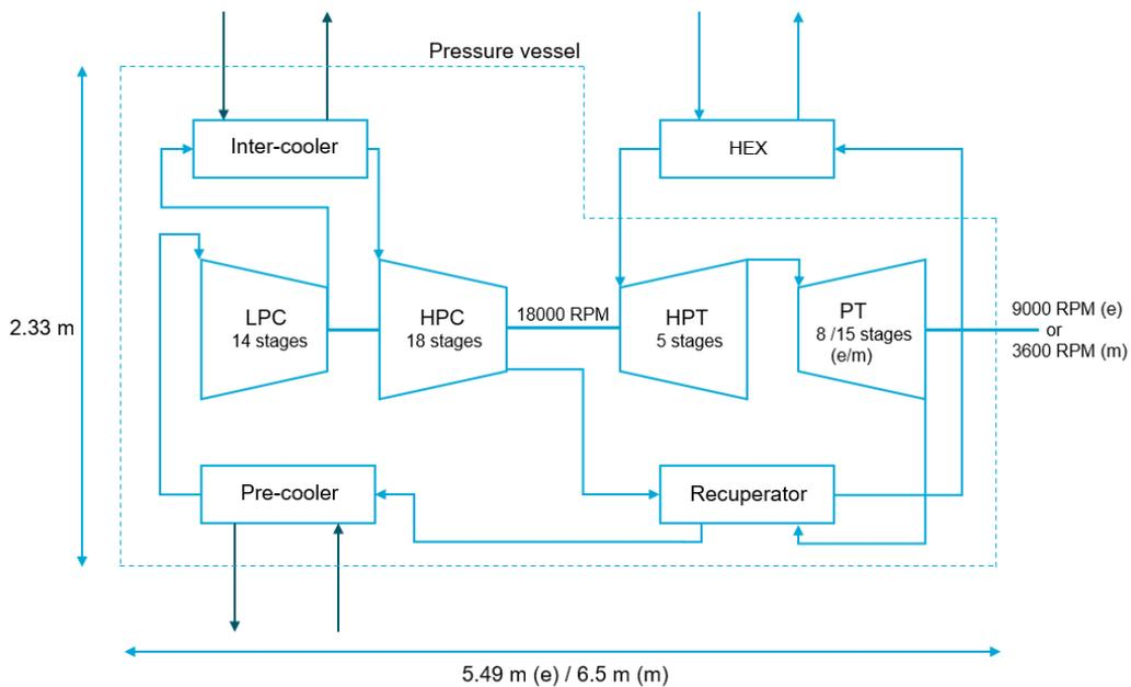
**Figure 6.5:** Schematic of the helium power cycle of a marine turbine delivering 52.2MW mechanical (m) or electric (e) power inspired by [54]
