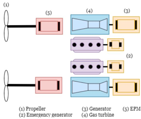
**Figure C.2:** IPS propulsion configuration used with SMR, vSMR and conventional GTS
