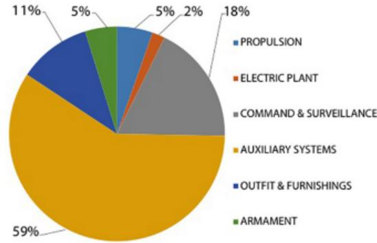
Figure 4.2: Proportional distribution of the total installed electric load on the F105 [11]
