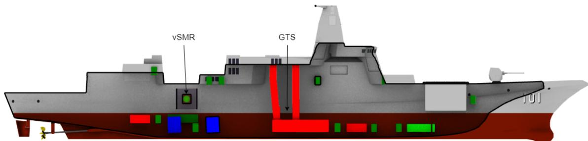
**Figure 9.5:** Side view of a hybrid configuration containing a vSMR for future SEWACO load and a conventional GTS
