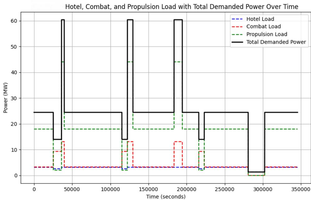
Figure N.1: Example of operational profile from table N.1 used in Python
