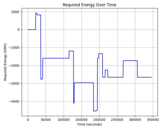
**Figure 7.7:** Required ESS capacity for  $P_{tot}$  ( $8 \cdot P_e = 10\text{MW}$  and  $f_{ramp} = 10$ )
