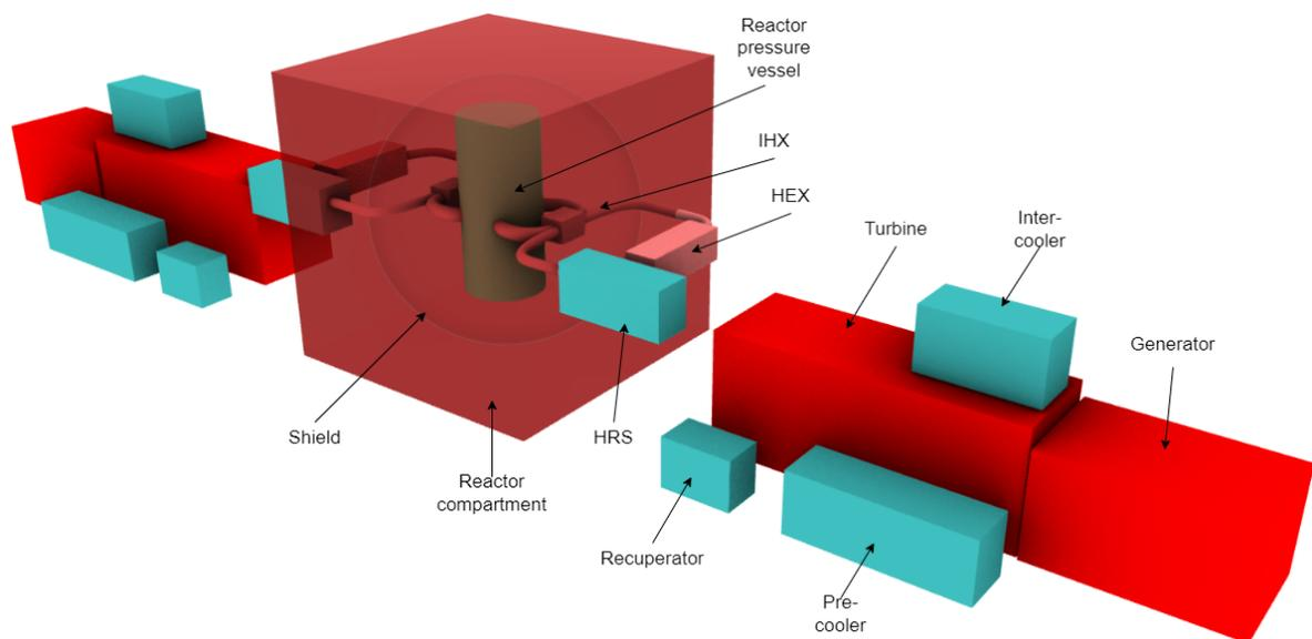
**Figure P.2:** SMR layout with component labels ( $230\text{MW}_{th}$ )
