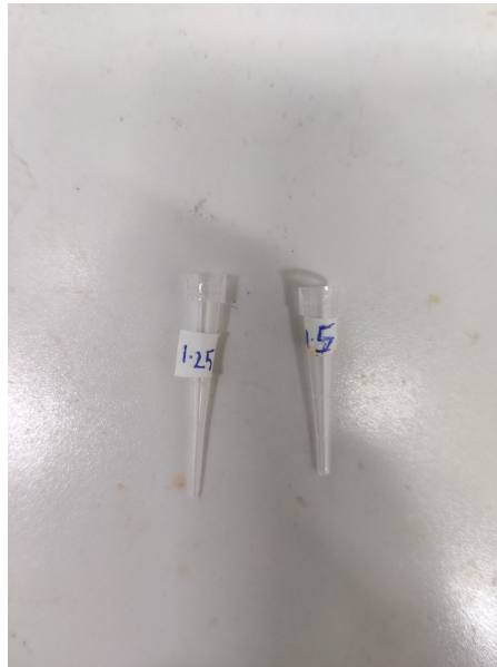
Figure 6.3: Pipette tips for ethanol, for drop of radii 1.25 and 1.5 mm. It can be seen here that the tip used to produce a drop of 1.5 mm radius is shorter and has a broader opening at the end.
