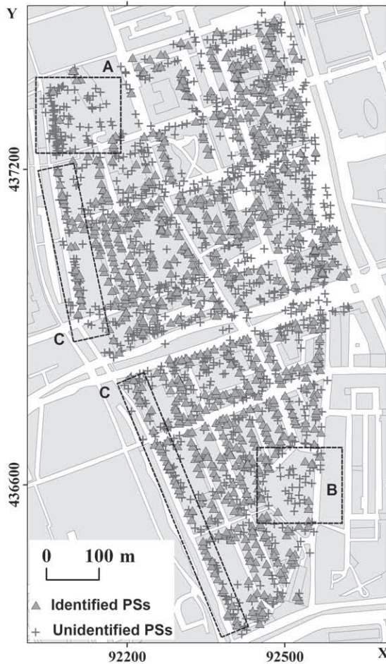
Fig. 14. Matched and unmatched PSs. A-labeled area: new building absent in the LOD2 model. B-labeled area: green-area free of buildings, where the PPs correspond to urban structures not included in the model. C-labeled areas: examples of predicted PSs at the linear structures of buildings and identified as triple bounce.
