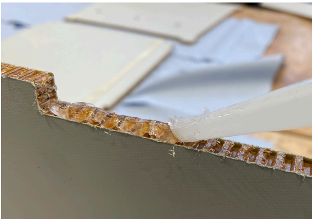
Fig 3.18: Using transparent adhesive to bond the panels
