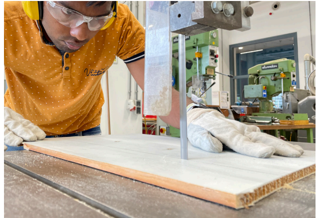
Fig 3.17: Cutting the panel with band-saw
