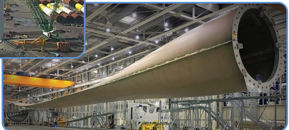
Fig 1.7: 107 meter long composite wind turbine blade 4
