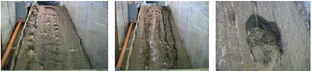
Figure 4.1: Forms of erosion (Weißmann, 2003)
