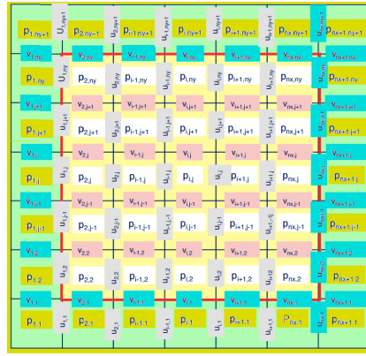
Figure 5.2: Staggered grid with (nx - 1) \times (ny - 1) control volumes: The square with red borders represent the computational domain where velocity and pressure components are unknown except the vertical velocities on the upper and lower boundaries and the horizontal velocity components on the right boundary due to periodicity
