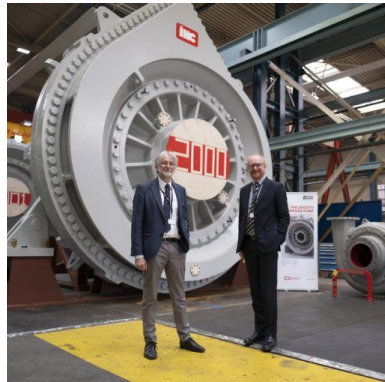
Figure 1.1: An 8500 kW dredge pump with a 1050 mm diameter suction pipe and a 2520 mm diameter impeller (source: Royal IHC).
