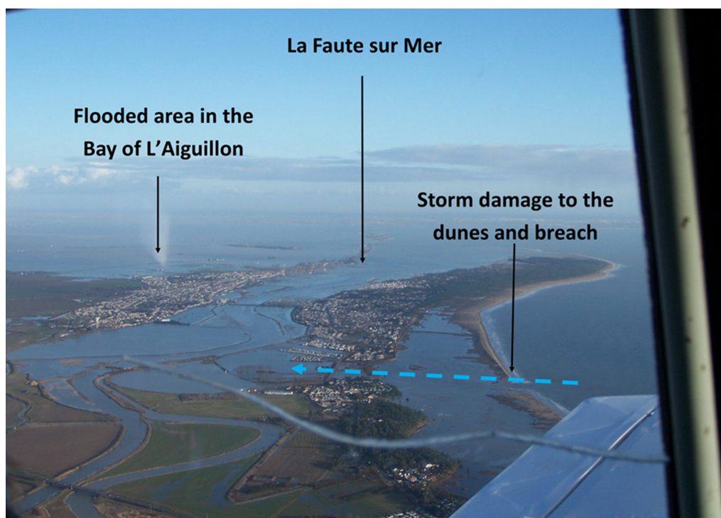
Figure 1. Aerial photograph (28 February 2010) illustrating how the erosion of Belle Henriette (right) created an additional pathway for floodwaters (blue arrow) into La Faute-sur-Mer, France during Storm Xynthia 2010 (Photo J.-P. Bichon, interpretation M. Garcin, BRGM; see also Pedreros et al., 2010, Gerard and Lang, 2019).
