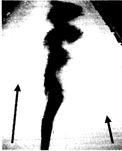
Figure 2.2: A bird's-eye view of a dye injection downstream of the splitter plate. The arrows indicate the magnitude and direction of the velocity.
