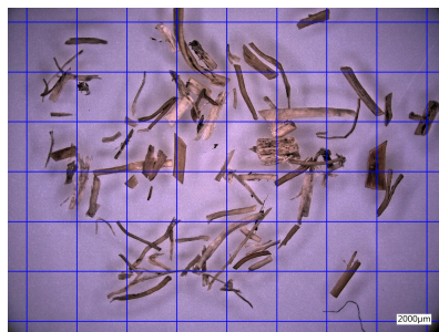
Figure A.7: Particle size distribution of EFB fibres prior to the FTIR analysis
