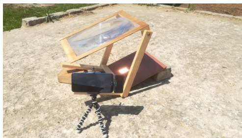
Figure 4.1: Set up for the thermal experiments using the Fresnel lens
