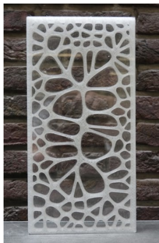
Figure 2 Thin glass composites, based on a structural efficiency increasing design strategy (Neeskens, 2018)
