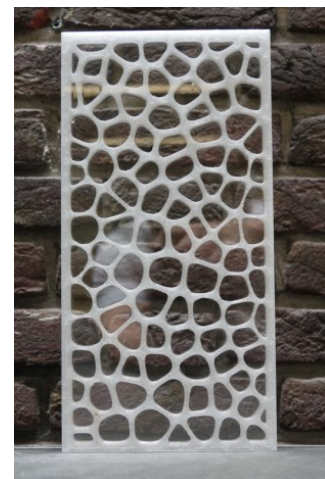
Figure 2 Thin glass composites, based on a structural efficiency increasing design strategy (Neeskens, 2018)
