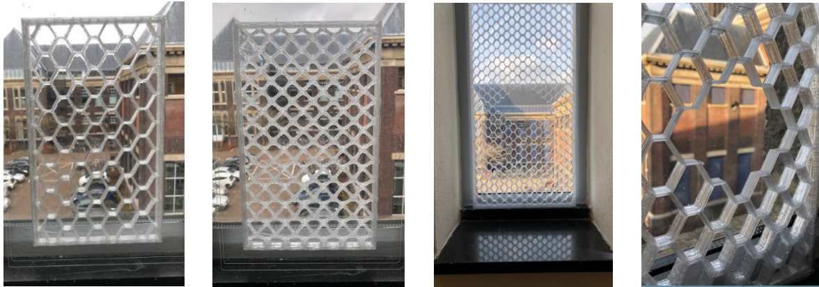
Figure 3 Ultra-thin composite panel: A research on the durability and stiffness of a composite panel of (thin) glass and recycled PET (Saleh, 2019)
