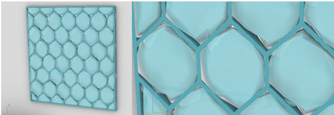
Figure 92 Inflatables in hexagonal core, where the inflatables have the same shape as each cell
