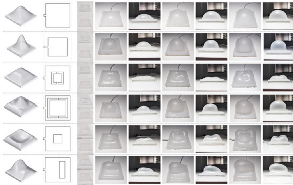
Figure 57 Sample swelling testing and morphology detection of inflatable module, the patterns used respectively none, central, average, average central, periphery and one-sided (Wang, 2023)
