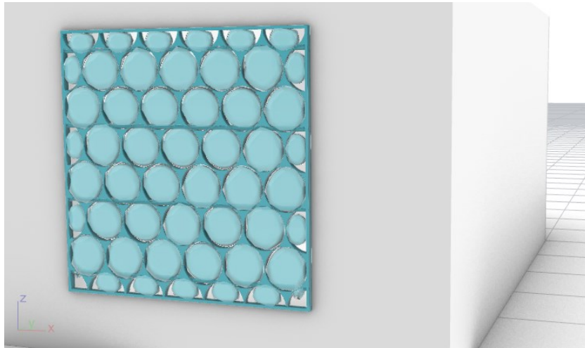
Figure 91 Inflatables in core pattern with circular cells
